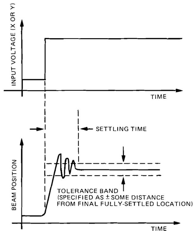
Figure 3-4. Settling Time
