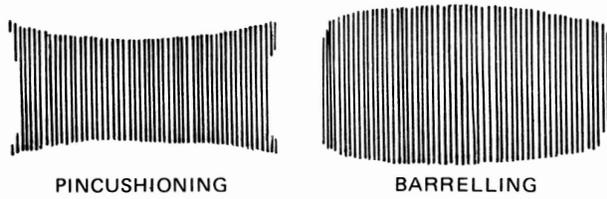
Figure 3-6. Geometric Distortion Caused by CRT (exaggerated)
