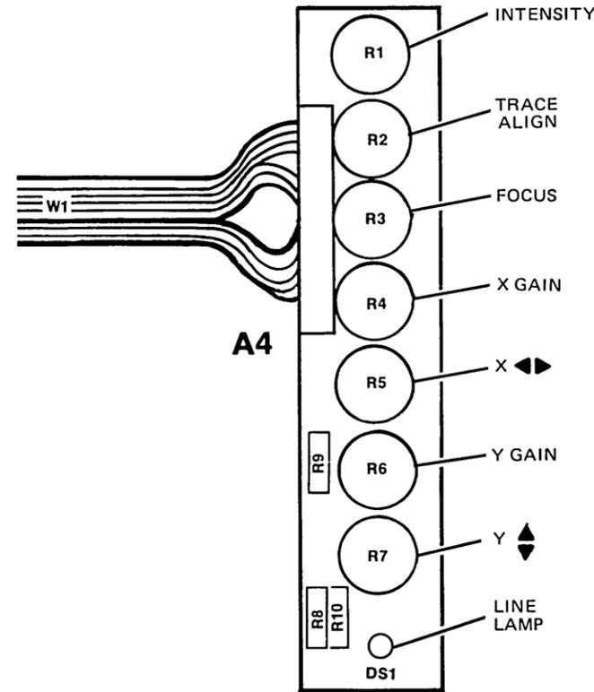
Figure 8-2. Component Identification, Control Assembly, A4
