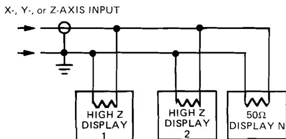
Figure 3-2. Input Termination Impedance of Displays Connected in Parallel
