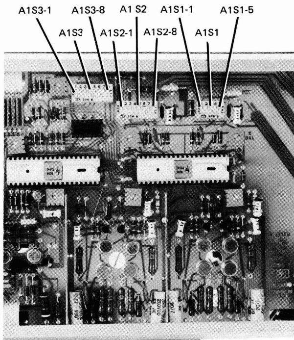
Figure 3-1. Input Attenuation and Bandwidth Selection Switches
