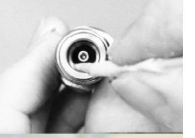
Never apply pressure to inner conductor
