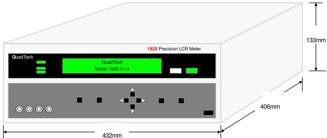
**Figure 1-3: Instrument Dimensions**
