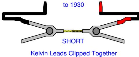
Press the **[START]** to initiate **short calibration** measurement
