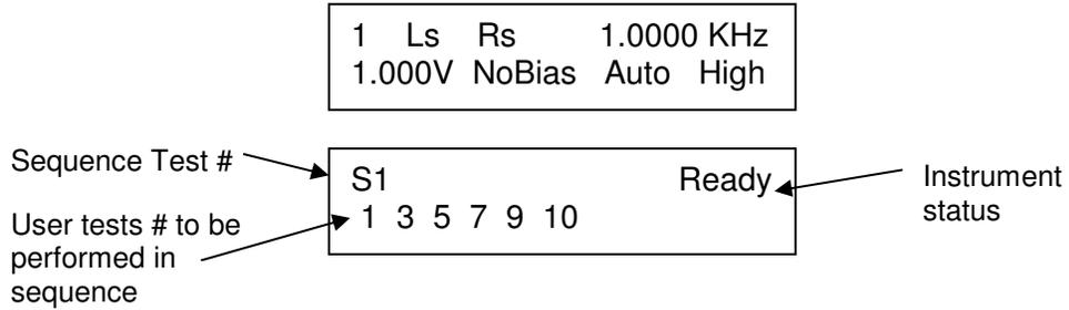
The above display is typical showing **S1** is the sequence test setup #, the sequence programmed to perform user tests **1,3,5,7,9,and 10** in succession, and **Ready** the instrument status. To select any other sequence test number simply press the **Up or Down** arrow keys while in the Ready state.
