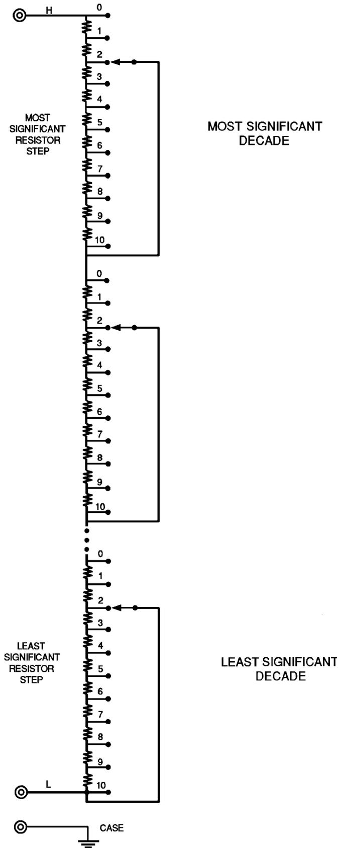
Figure 4.1. HARS Series Schematic Diagram
