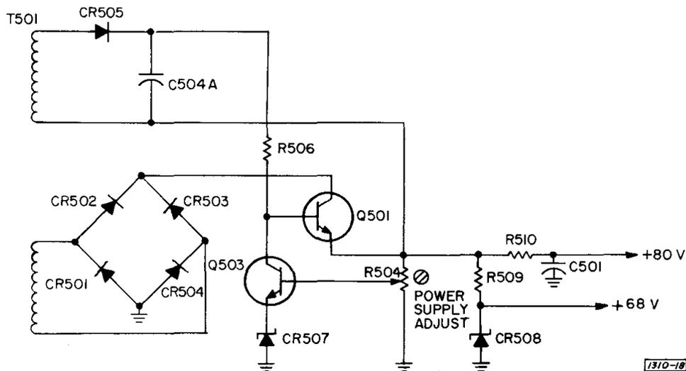
The power supply contains two regulators which provide two outputs: +80 volts B+, and +68 volts B+.
