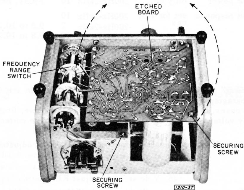
Disconnect from the etched board the six wires that are connected to the FREQUENCY range switch, remove the two securing screws, and swing the board up.
