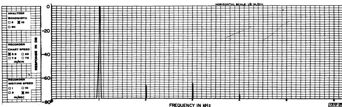
**Frequency multiplication.** The harmonic content of the reference can be used for precise frequency multiplication since the oscillator can be synchronized to the harmonics. The accuracy and long-term stability of the submultiple reference are maintained and the oscillator output is, of course, sinusoidal. This technique can be used with most signals because harmonics are usually present or can be easily generated.
