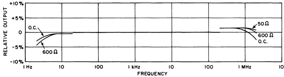
The output is 20 volts, open-circuit, behind 600 ohms and is adjustable over a 50-dB range by a constant-percentage-resolution attenuator. The output is constant within  $\pm 2\%$  from 20 Hz to 200 kHz for loads of 600 ohms or higher. Within the audio range, changes are imperceptible on the usual analog type of voltmeter.
