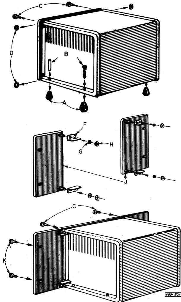
be necessary, however, to remove the end frames when reinstalling the rigid (metal shafts) front feet. The end frames slide off the side panels. Make sure the spring and pin are inserted in the bottom threaded hole on the frame, with the spring inserted first. Push the pin back with a pointed object and insert the rigid foot through the frame, threaded end first; screw the feet on to the shafts.
