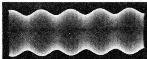
Reduction in am in the output of the oscillator locked to the signal above.
