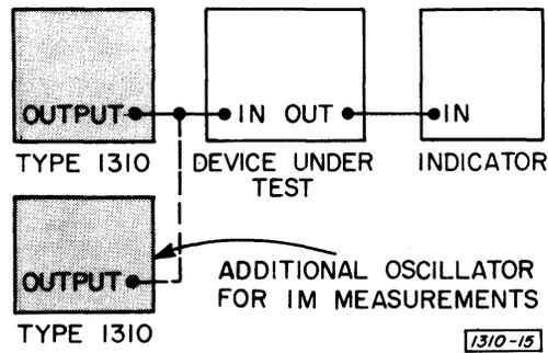
**Response measurements.** Constant output over a wide frequency range facilitates frequency-response measurements.
