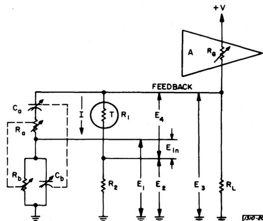
In order to stabilize  $E_3$  with changes in frequency and amplifier gain, a negative-temperature-coefficient thermistor is used for  $R_1$ . An ordinary resistor is linear, its resistance remains essentially constant as the current through it changes. But the thermistor used in the Type 1310 is non linear, its resistance *decreases* as the current through it *increases*.
