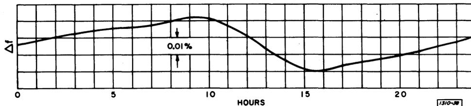
High-stability, frequency-determining components in the oscillator and low, internal power dissipation result in a stable output frequency. Drift during warm-up is typically below 0.1% at frequencies above 20 Hz.
