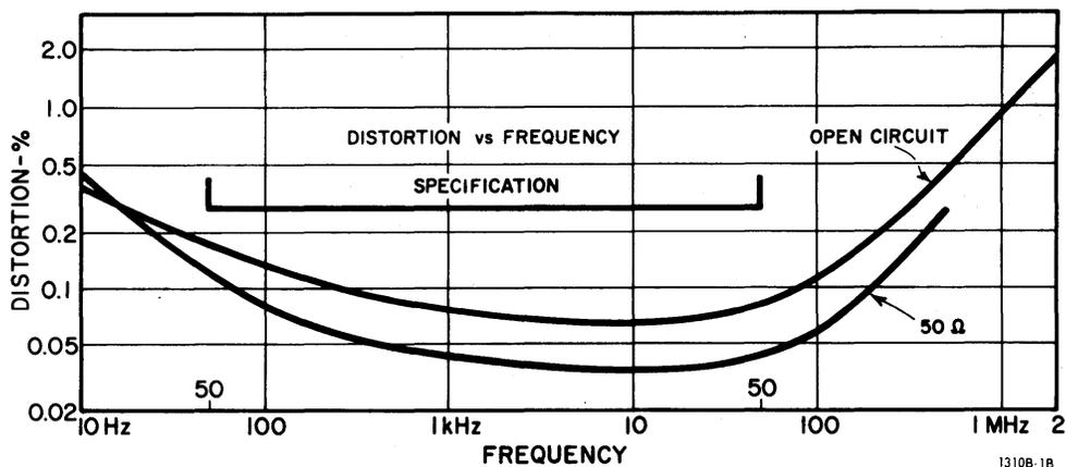
Harmonic distortion is less than 0.25% over most of the audio range (50 Hz to 50 kHz). This low distortion is always available, even at full output, because it remains essentially constant regardless of the size of the linear load applied, including a short circuit.
