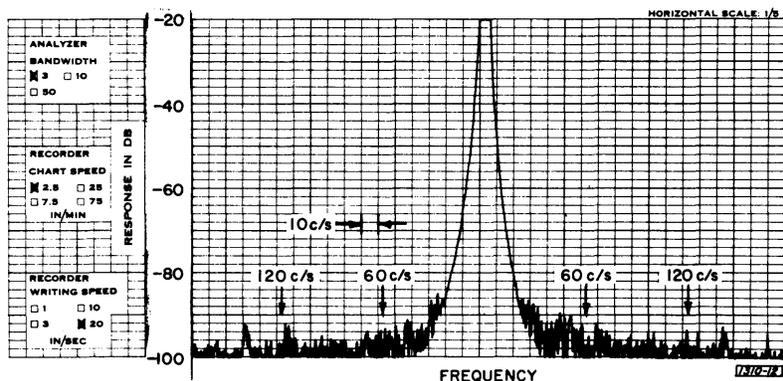
Hum is below 0.02% of the output (typically 0.005%), regardless of the attenuator setting. Noise at frequencies distant from a 1-kc fundamental, measured in a bandwidth of 5 Hz to 500 kHz, is typically less than 0.02%. Noise close to the fundamental is also low as the spectrum analysis of a 1-Hz output shows. Note the absence of components at the line frequency or its multiples.
