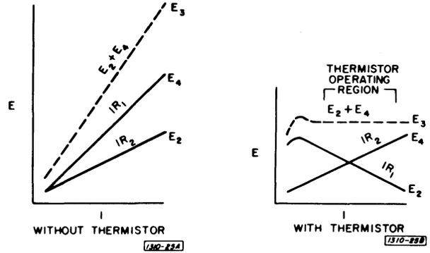
When an ordinary resistor is used for  $R_1$ , the voltage drops across  $R_1$  and  $R_2$  change in direct proportion to the current through them, which, in turn, changes in direct proportion to the gain (current-delivering capability) of the amplifier. In the above graph, the result of increasing current,  $I$ , is shown. Since  $E_3$  is the sum of  $E_2$  and  $E_4$ ,  $E_3$  rises linearly as the gain of the amplifier rises.
