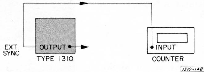
**Balanced output.** The output sync signal is  $180^\circ$  out-of-phase with the front-panel output, which makes it possible to obtain a high-impedance output, balanced with respect to ground, to drive push-pull circuits. The degree of balance is conveniently set with the LEVEL control.
