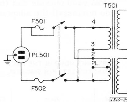
**230-volt line.** Power required is 210 to 250V, 50 to 400 Hz, 12W. Input plate for 230-volt operation is part number 5590-1664 and attaches to the rear of the cover, under the hole for the power connector, by means of two 4-40 x 3/16-inch screws with attached lockwashers, part number 7090-4030 each. For transformer wiring, connect 2 to 3 only. Fuse for F502 is 0.125 A, 3AG Slo-Blo, part number 5330-0450. F501 is a spare fuse.
