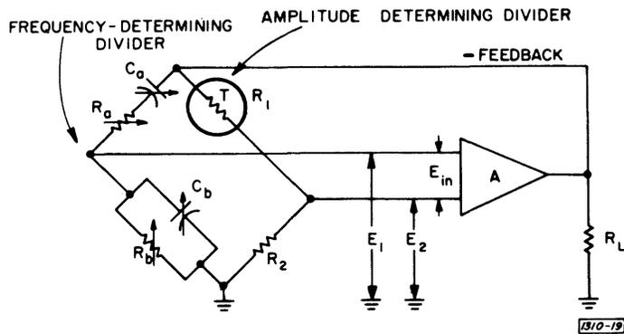
A Wien bridge consists of two parts, a frequency-determining impedance divider which provides positive feedback to sustain oscillation and an amplitude-determining resistive divider which provides negative feedback to stabilize amplitude.
