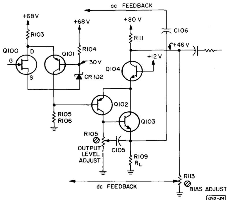
The drain (D) current of Q100 is applied to a grounded-base amplifier, Q101. Dc bias for Q100 is maintained at +15 volts by a divider, R104 and CR102. The amplified signal is taken from the collector and applied to the base of Q102 in a common-emitter connection.
