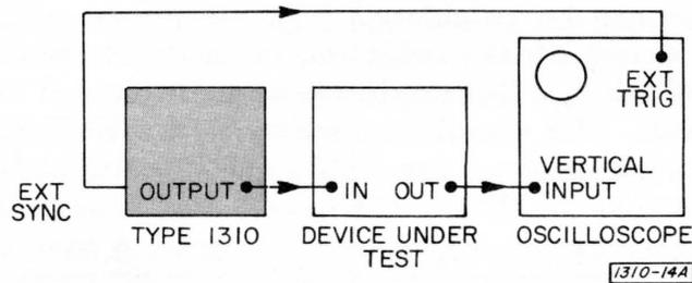
**Counter trigger.** A counter can be driven from the EXT SYNC jack when more precise adjustment of frequency is desired or when the front-panel output is not sufficient to trigger the counter.
