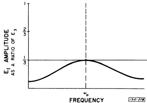
The transfer function (gain and phase shift) of the frequency divider is:
