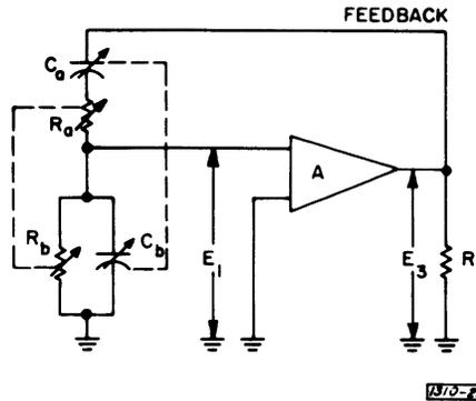
The operating frequency,  $f_o$ , of a Wien-bridge oscillator depends on the values of the components in the impedance divider:
