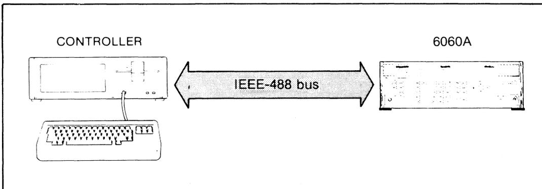
Figure 2-5. 6060A Signal Generator Connected to a 1722A
