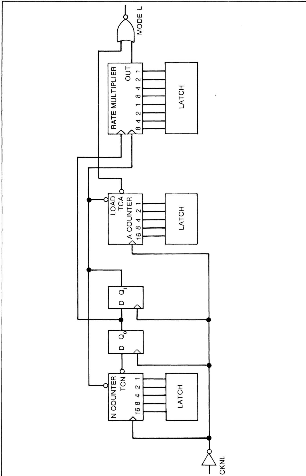
Figure 3-2. N-Divider Operation
