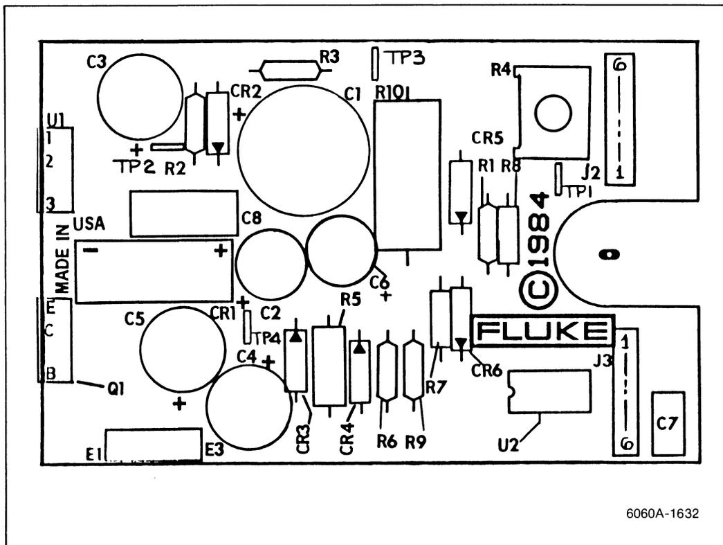
Figure 130-1. A3A2A1 High Stability (Ovened) Reference PCA
