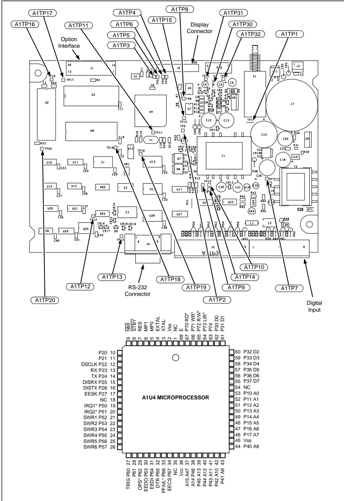
Figure 5-1. Test Point Locator, Main PCA (A1)
