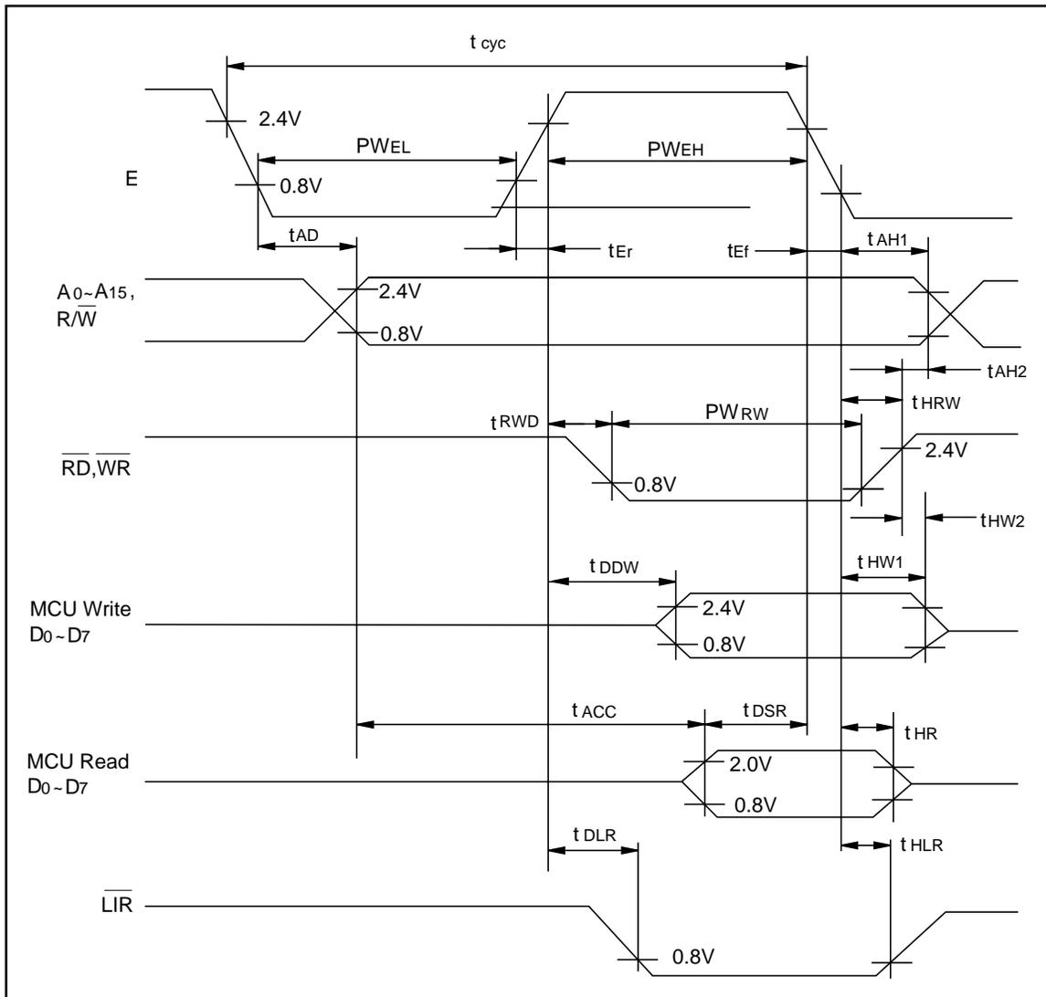
**Figure 5-7. Microprocessor Timing**
