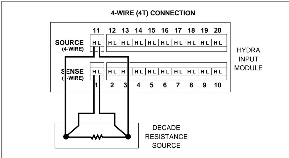
Figure 4-5. 4-Terminal Connections to Decade Resistance Source
