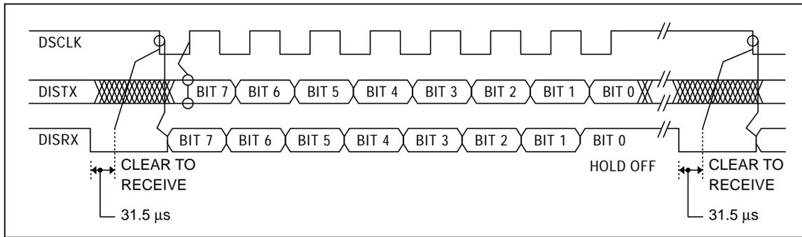
**Figure 5A-9. Display Controller to Microprocessor Signals (2635A)**
