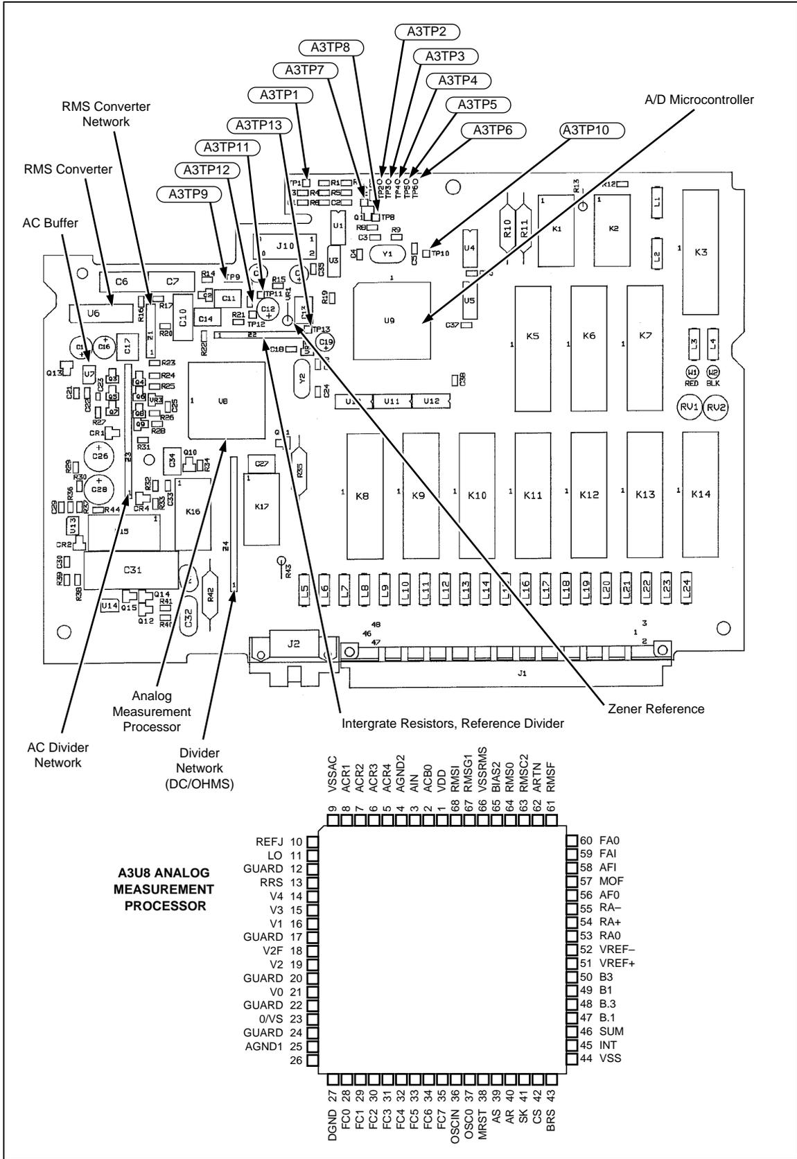
Figure 5-4. Test Points, A/D Converter PCA (A3, A3U9)
