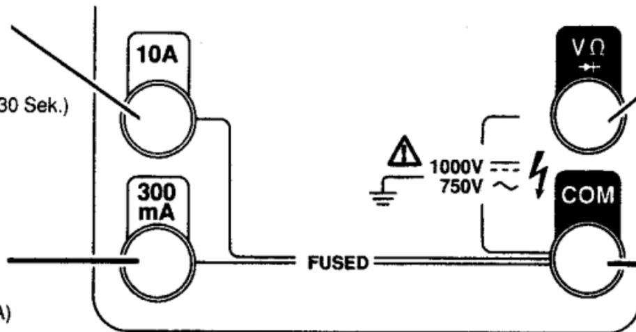
VOLTS, OHMS, DIODE TEST
