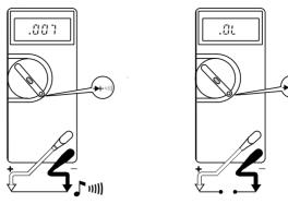
If continuity exists (resistance < 210  $\Omega$ ), the beeper sounds continuously. The meter beeps twice if it is in the Touch Hold® mode.
