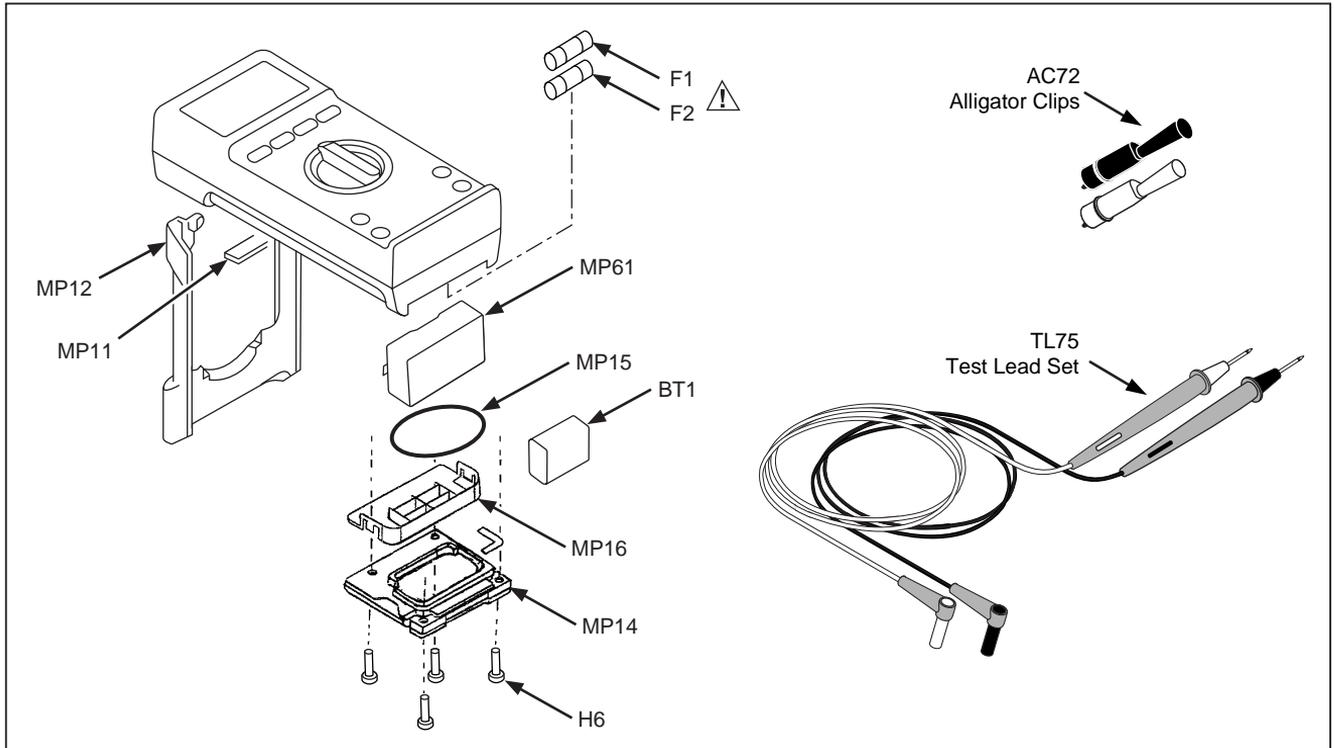
Figure 2. Replaceable Parts
