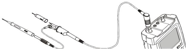
**Figure 36. Probing Using 2-mm Heavy Duty Test Probes**
