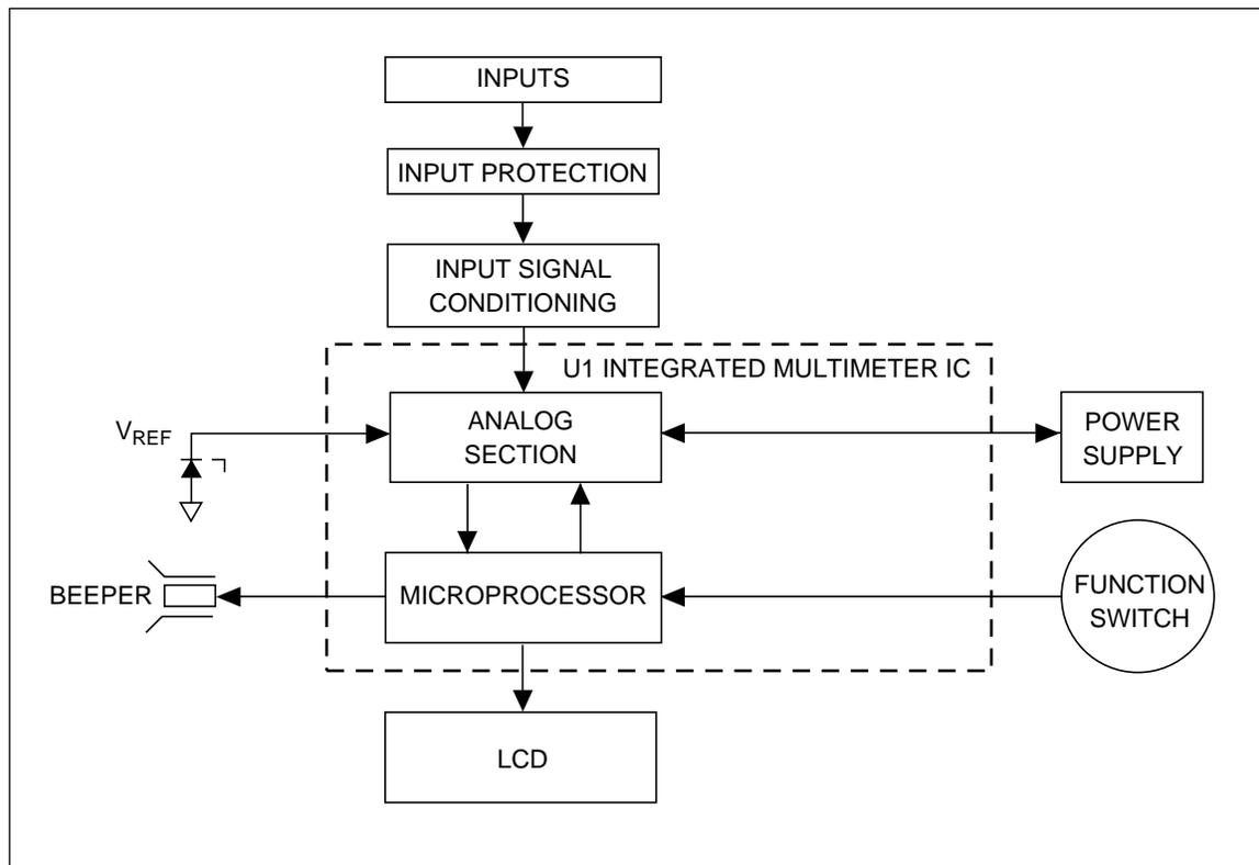
Figure 2-1. Block Diagram
