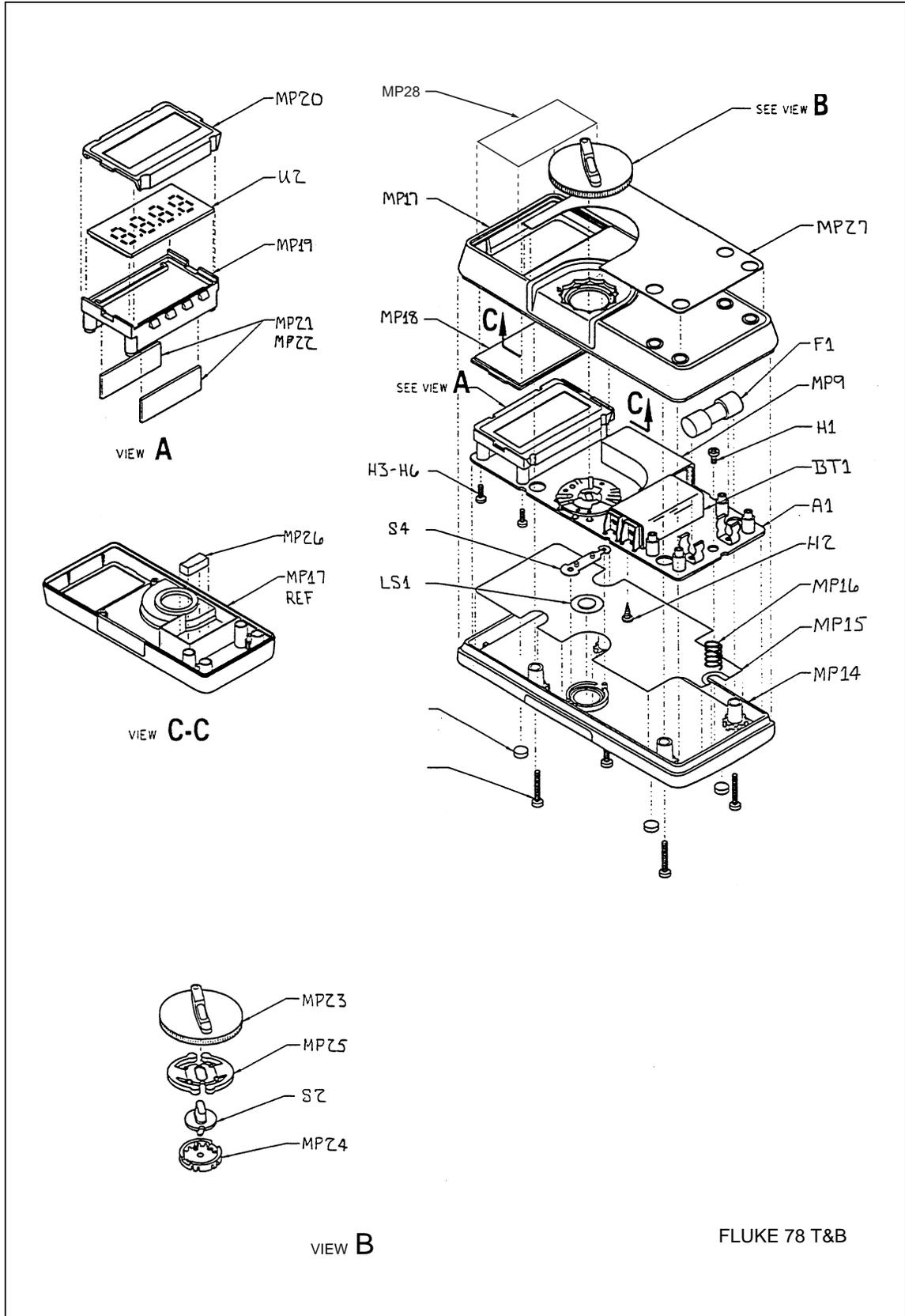
Figure 4-1. Fluke 78 Final Assembly
