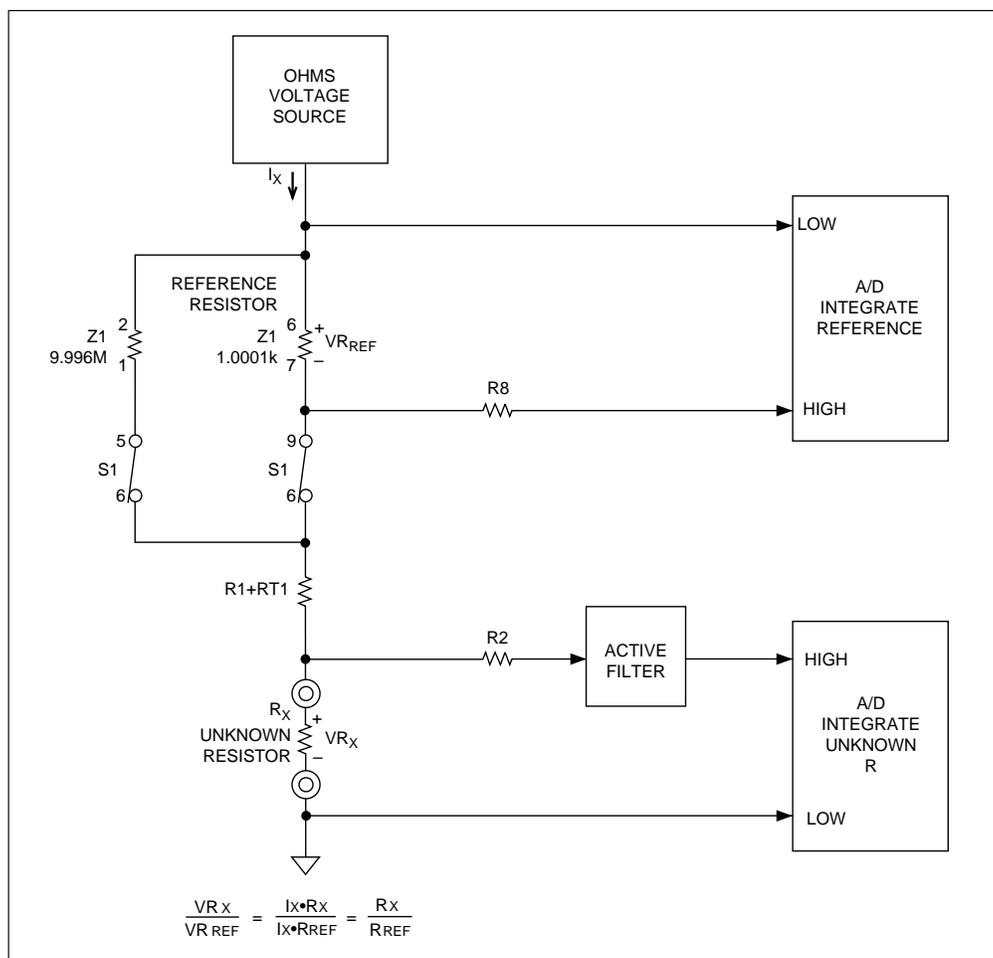
Figure 2-3. 400 Ohm Range Simplified Schematic
