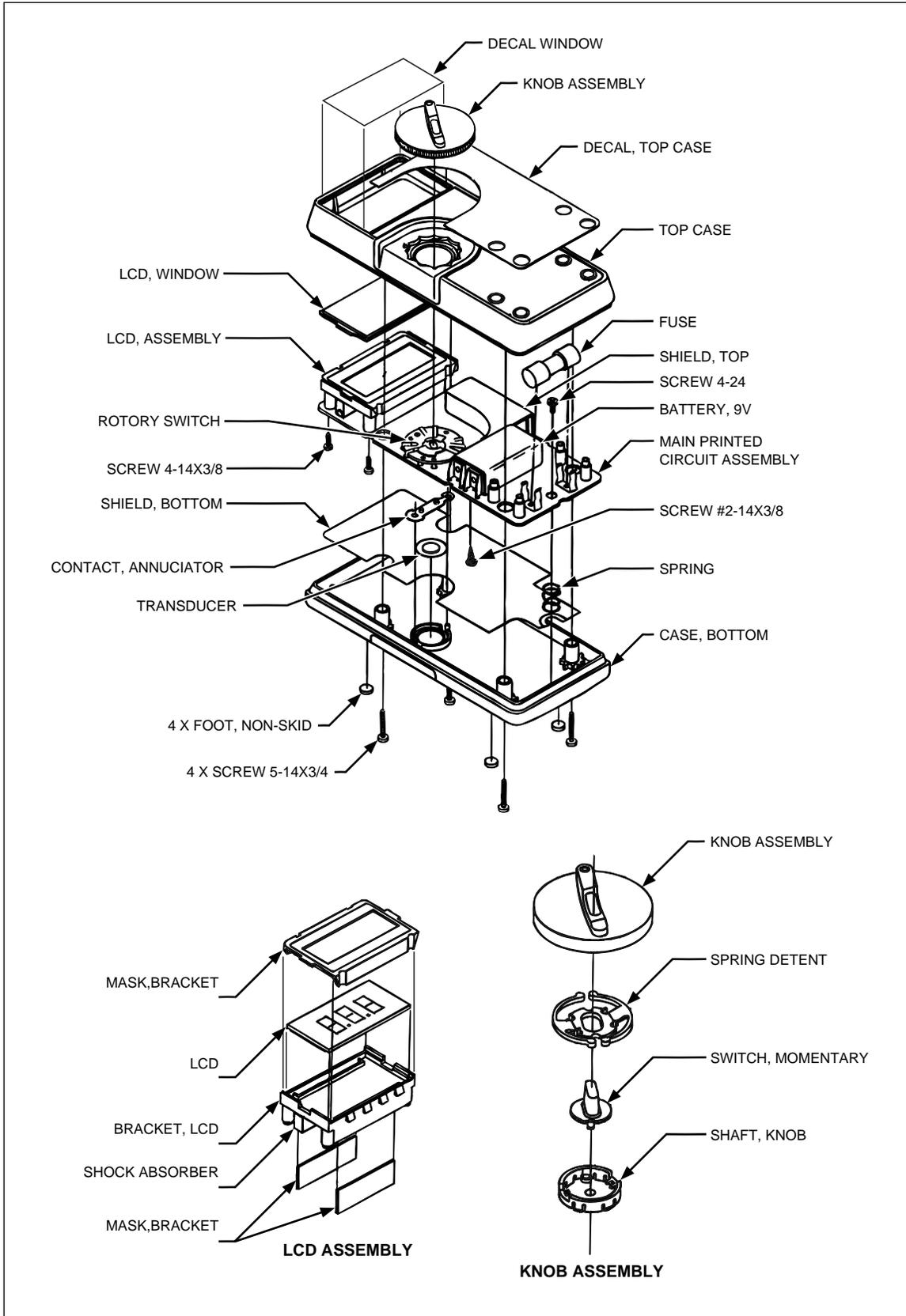
Figure 3-1. Disassembled Fluke 78
