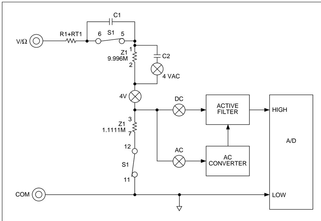
Figure 2-2. 4 V Range Simplified Schematic
