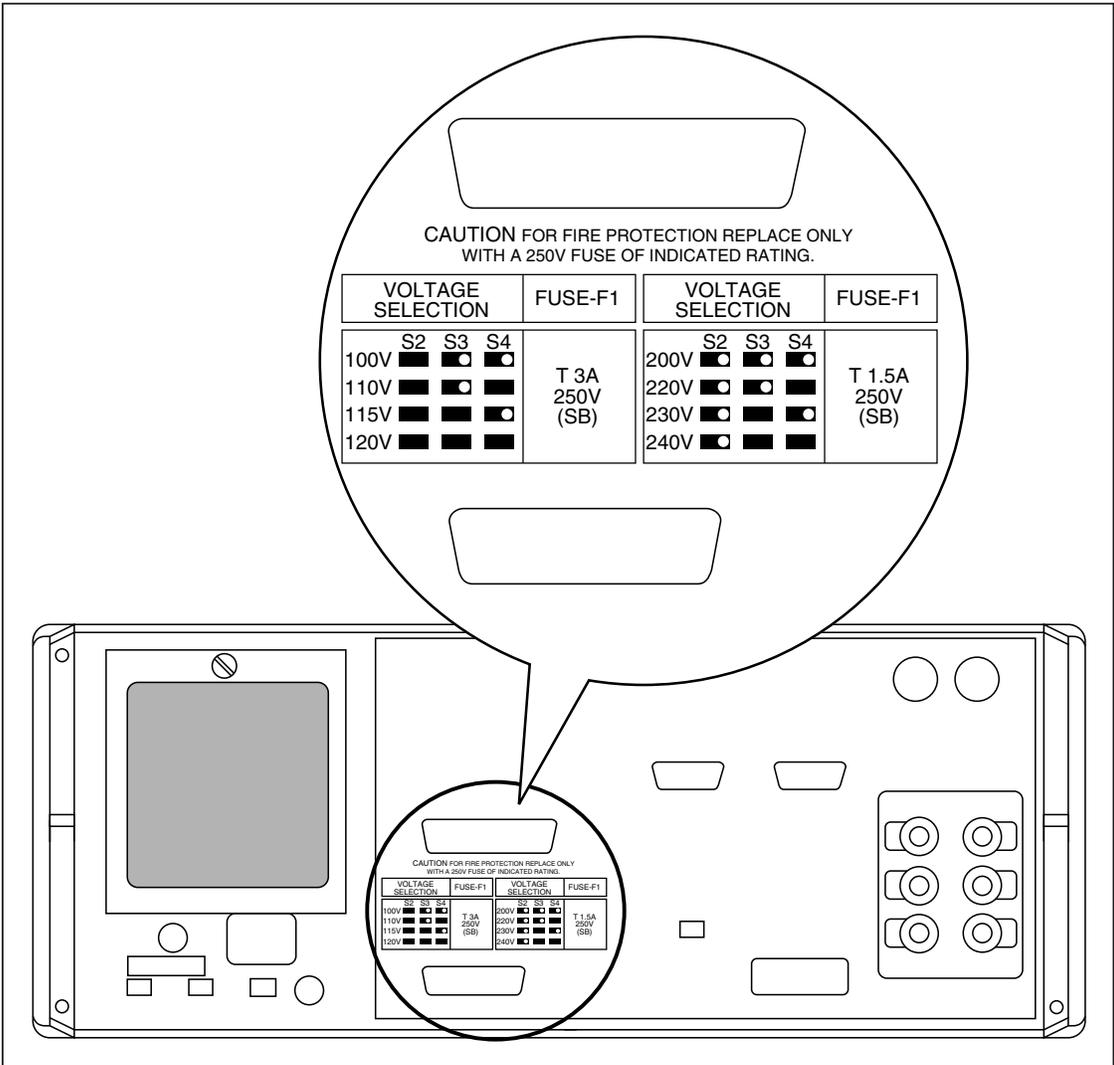
**Figure 4. Line Power Label and Switch Location**
