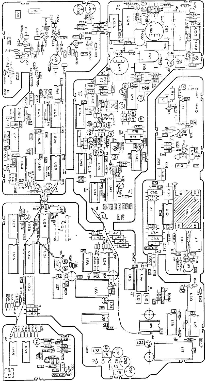
Figure 8-6. A2A1 Synthesizer PCA
