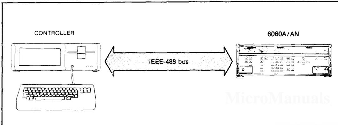
Figure 2-5. 6060A/AN Signal Generator Connected to a 1722A
