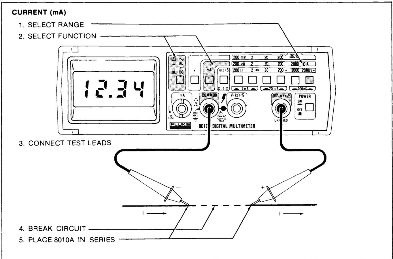
Figure 2-5. AC/DC Current Operation, 10A (8010A only)
