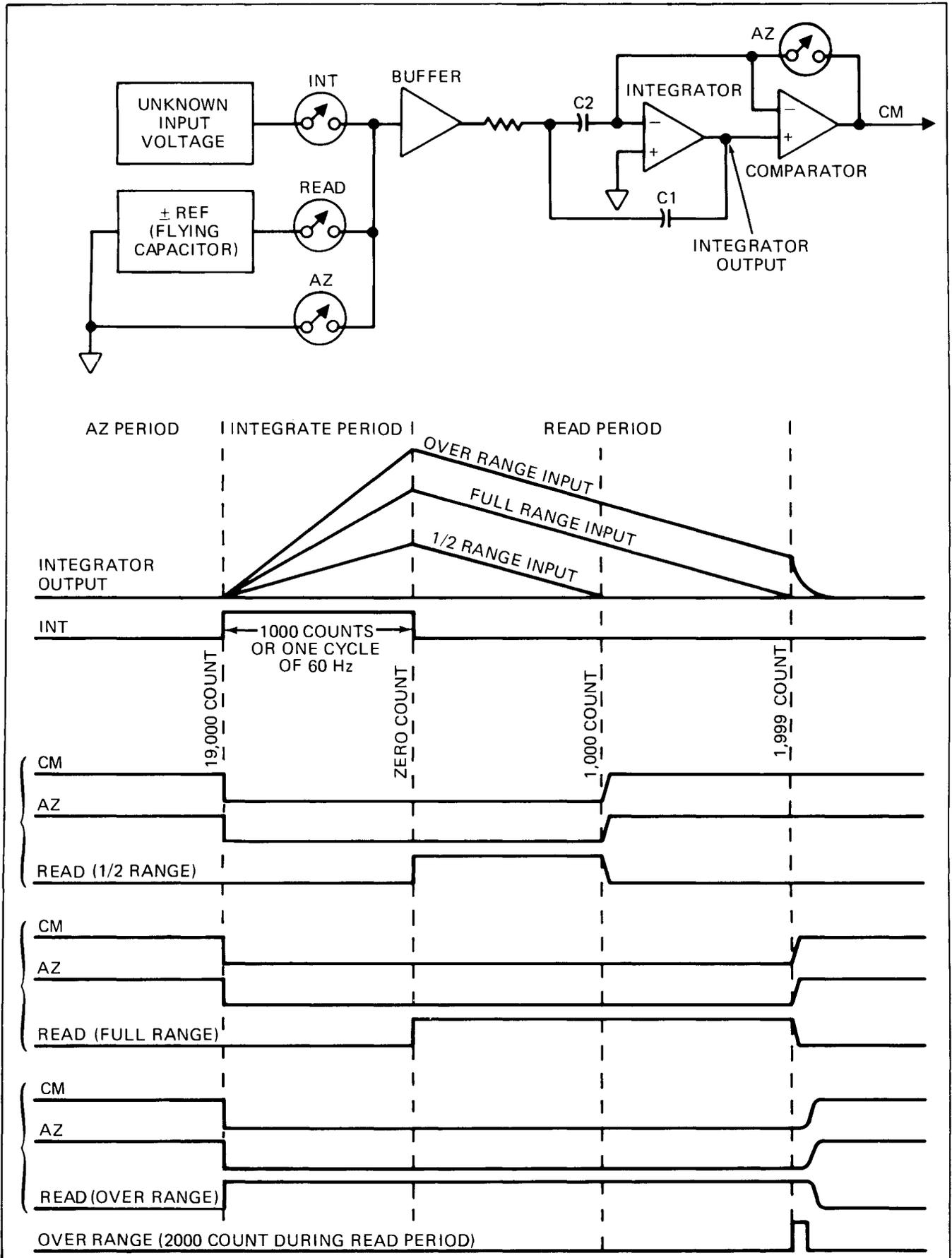
**Figure 3-2. A/D Converter Simplified Schematic and Timing Diagram**
