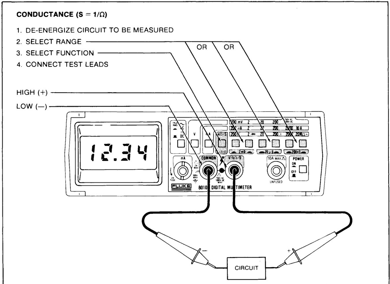
**Figure 2-8. Conductance Operation**
