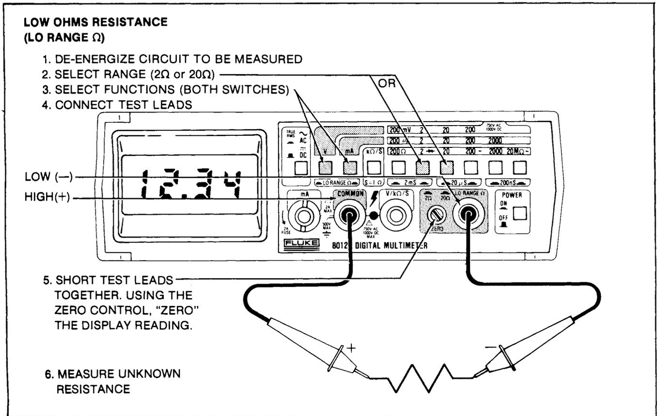
**Figure 2-7. Resistance Operation, LO Range  $\Omega$  (8012A only)**
