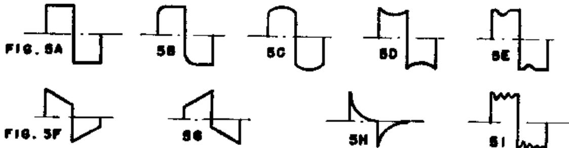
Fig. 5b shows "rounding" of the leading edge of the square wave. This indicates a drop off in gain at high frequencies. "Rounding" will generally be observable when there is a substantial drop in the gain by the tenth harmonic (or less). Therefore, if a 2 Kc square wave fed to the amplifier is reproduced on the 'scope without "rounding", the amplifier is flat to  $10 \times 2 \text{ Kc} = 20 \text{ Kc}$ .
