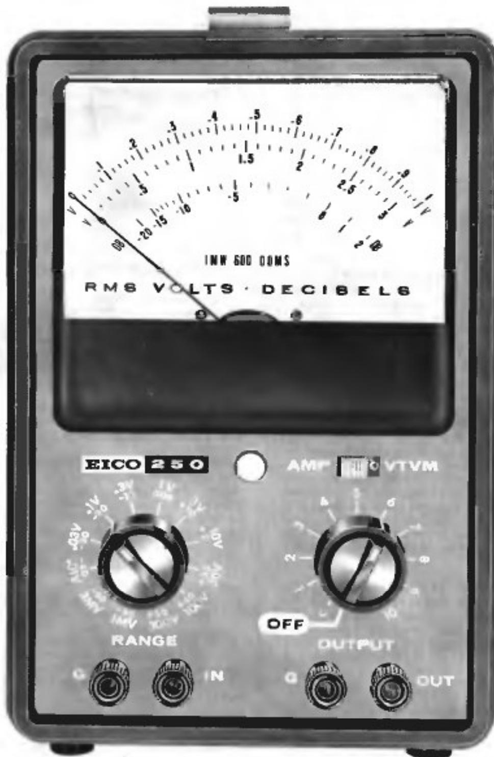
Figure 2-1. Front Panel Controls and Terminals
