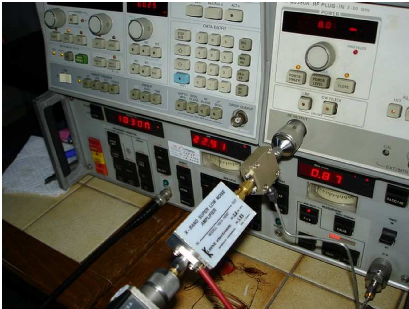
F5DQK February 2009 part 2/2 2 to 18 GHz NF+gain measuring with Eaton 2075 or HP 8970b and ADDS
