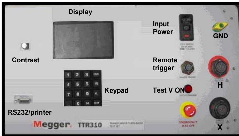
Figure 4-6. Three-Phase TTR310 Control Panel
