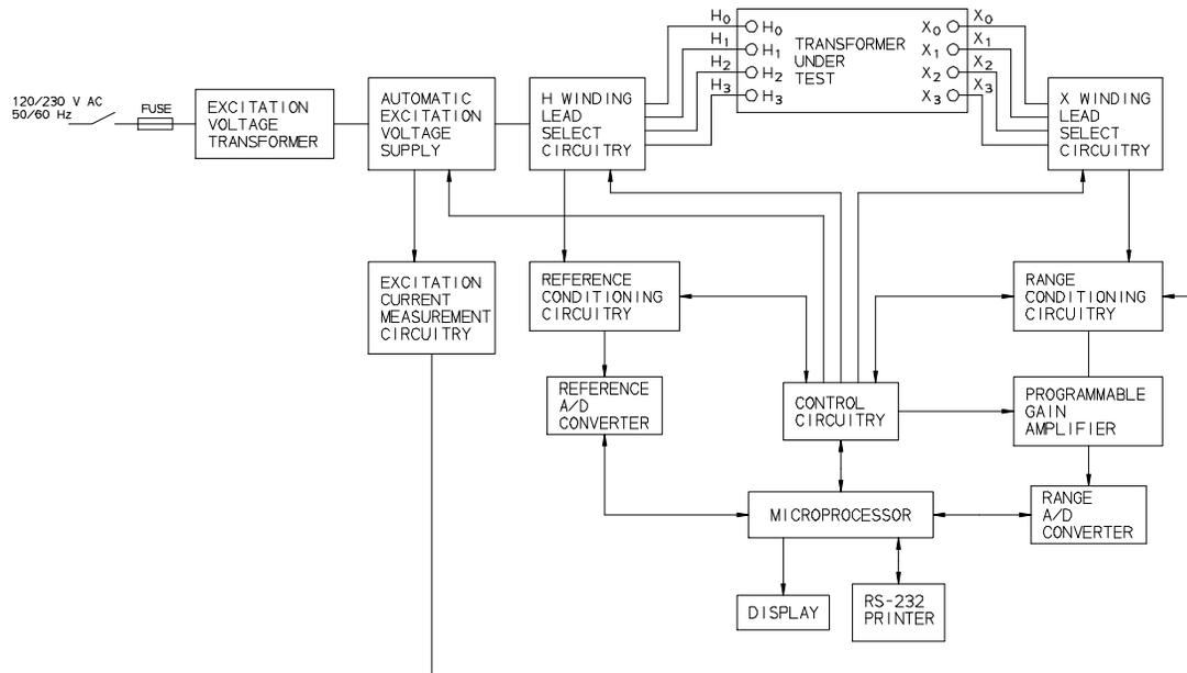
Figure 4-1. Three-Phase TTR310 Test Set Block Diagram
