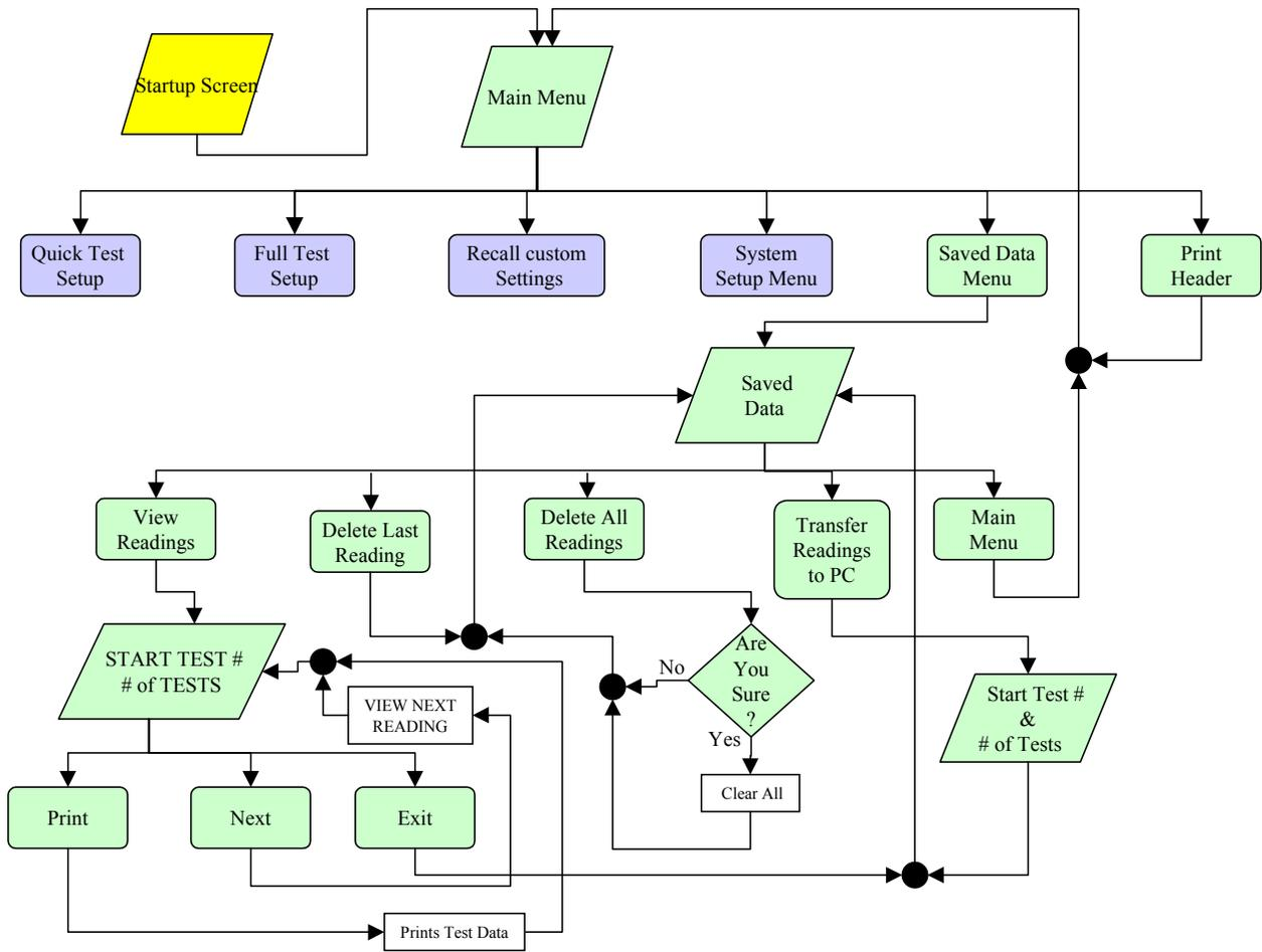
Figure 4-5. Saved Data Menu with Print Header
