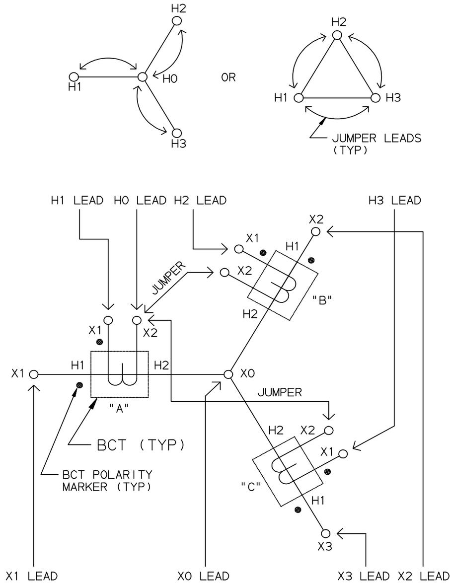
Figure 5-9. Setup for Testing BCT Mounted on Wye Winding of a Three-Phase Transformer
