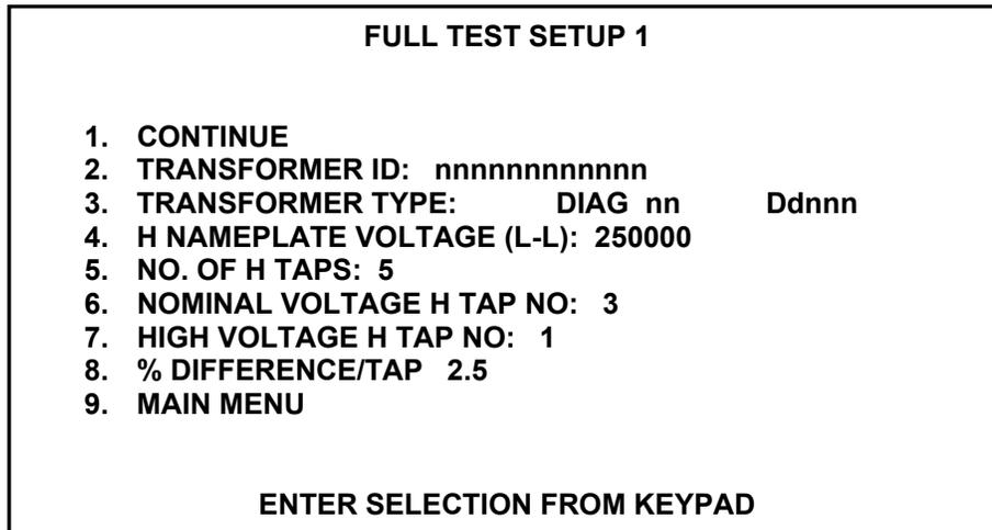
Figure 6-6. FULL TEST SETUP 1 Screen
