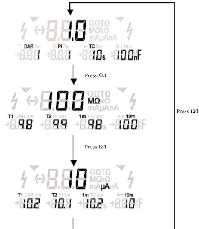
**Figure 3 - The result of a dielectric discharge test (DD)**
