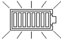
When mains power is present the indicator shows the battery is being charged by animating the segments of the bar graph.
