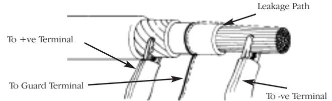
The guard terminal is at the same potential as the negative terminal. Since the leakage resistance is effectively in parallel with the resistance to be measured, the use of the guard causes the current flowing through surface leakage to be diverted from the measuring circuit. The instrument therefore reads the leakage of the insulator, ignoring leakage across its surface.
