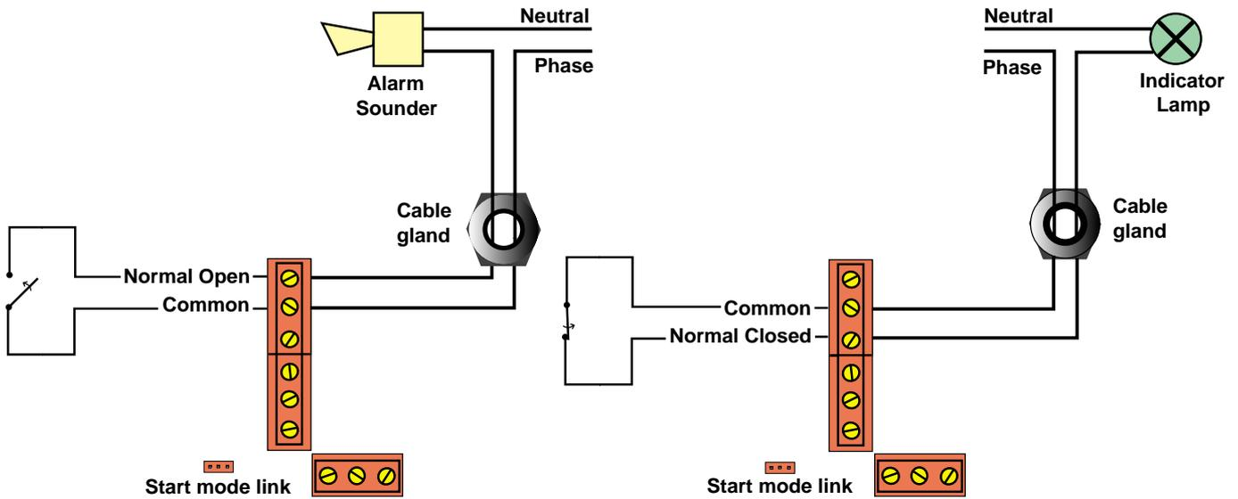
When the 'Failed' condition is active, the Common terminal is shorted to the Normally Open (N/O) terminal.
