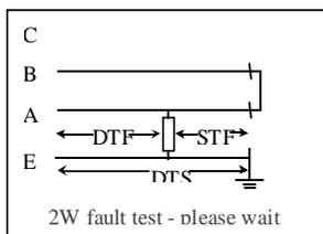
If the reading is within range, you will be asked if the cable under test is made up of one type of wire along its length (SINGLE) or multiple sections with different types of wire (MULTI).
