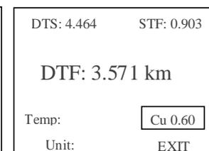
If the gauge of the cable under test is not included in the built in table, you can define your own gauge of wire by specifying its resistance per metre (or ft). This must be within the range 0.01000  $\Omega/m$  to 0.32500  $\Omega/m$  (0.10000  $\Omega/ft$  to 0.00300  $\Omega/ft$ ) or a warning of ABOVE MAX OF or
