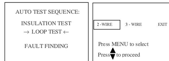
With the loop test, the auto sequence is used to verify that any loop resistances are  $< 2 \text{ k}\Omega$ . This is the A-B loop only on the 2-wire test and A-B and A-C loops on the 3-wire test.
