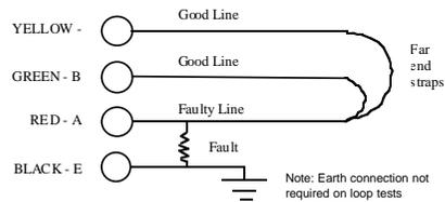
The 2-wire test method assumes that the Good Line and the Faulty Line are of the same gauge wire and approximately equal in length. Then the assumption that the strap is at half the total loop distance is valid. However, it is preferable to use a second return wire if possible to make use of the 3-wire testing method. Each of the Good Lines can be of different resistances and lengths compared with the Faulty Line. This can allow for a direct
