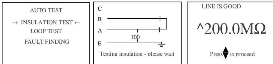
The result of the insulation test is then displayed as an insulation resistance ( $R_e$ ) – see the bridge specification for the measurement resolution and increments.
