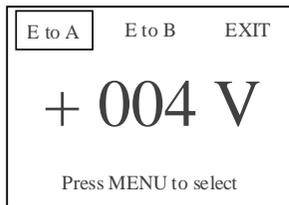
Use the MENU key (see #4 above) to automatically select the displayed DC voltage, either E to A Volts or E to B Volts and to highlight the exit option. Then use the Gain key (see #7 above) to confirm exit from the Voltmeter Mode.
