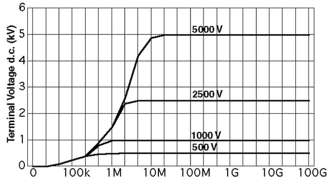
**Typical Terminal Voltage Characteristics**
