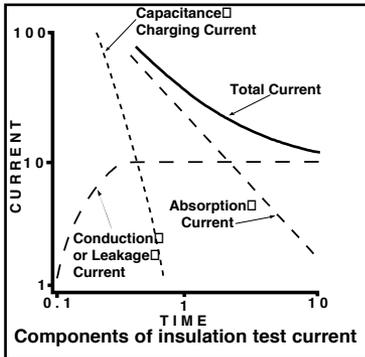
2. Absorption current. This current is also initially high but drops at a much slower rate than the charging current.
