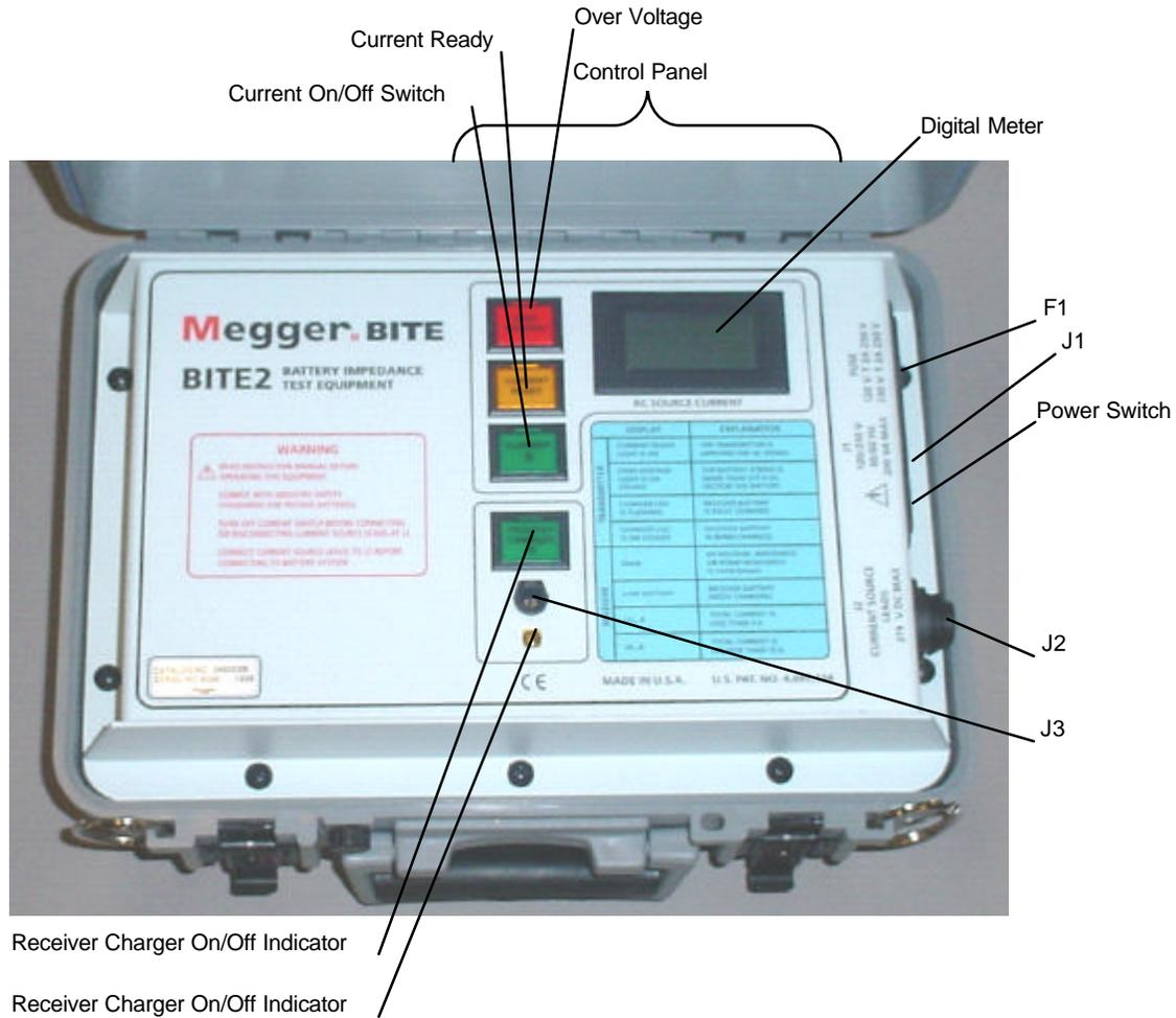
Figure 3-1: BITE 2 transmitter
