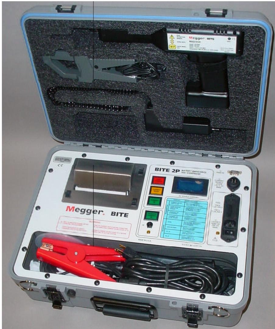
*Figure 1-2: BITE 2P instrument*
