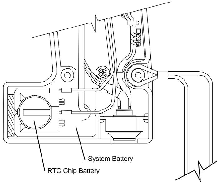
**Figure 9-1: RTC battery "piggybacks" the system battery**
