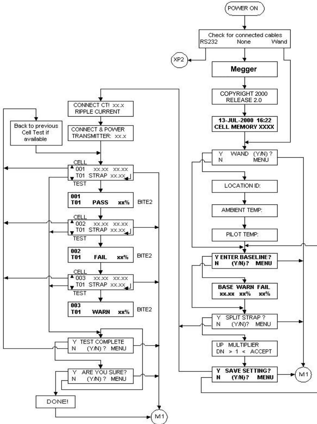
Figure 3-5: Flowchart for Receiver menus
