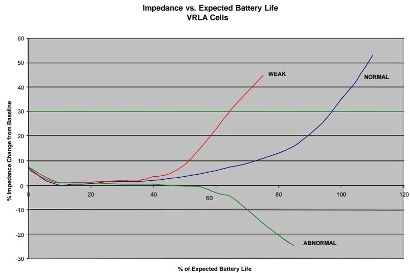
**Figure 7-1: Generic curve of impedance vs. cell life**
