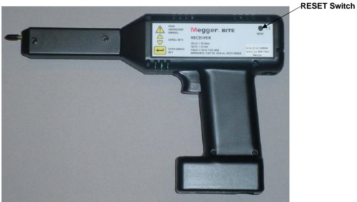
*Figure 3-9: Receiver RESET switch*
