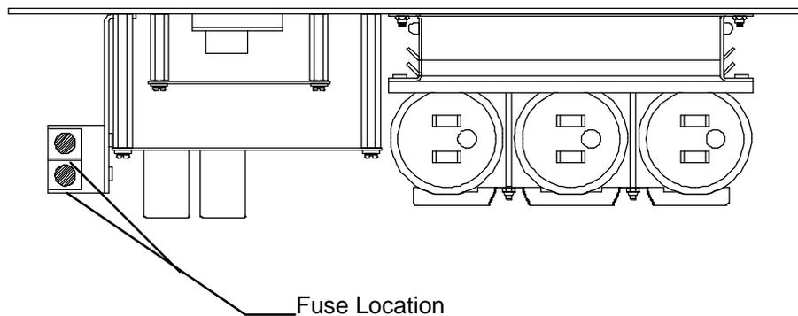
**Figure 9-3: BITE 2P transmitter secondary fuses (front view)**
