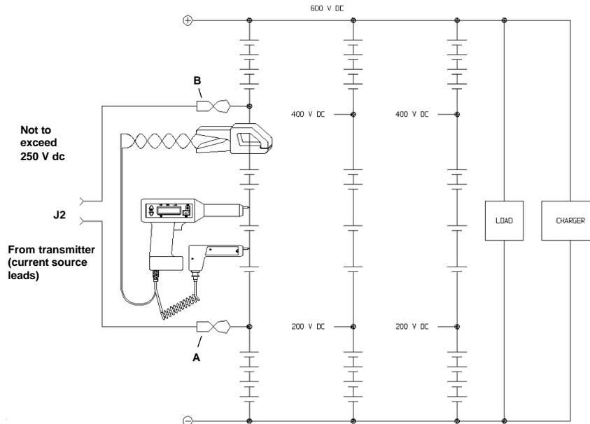
**Figure 5-2: Sectioning a battery system greater than 275 V**
