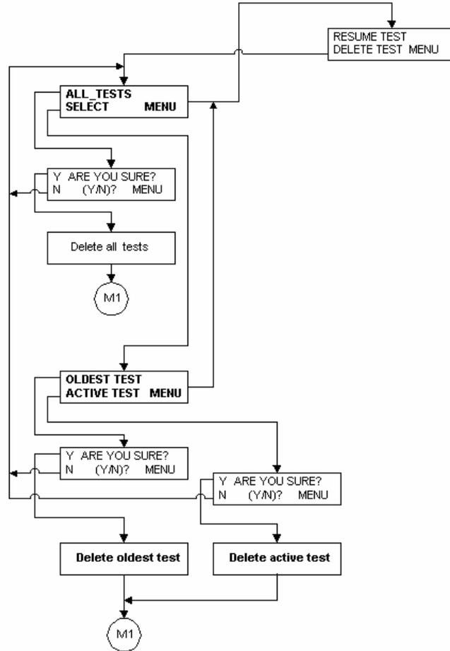
**Figure 6-3: Deleting test results from the Receiver**
