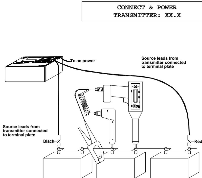
Figure 4-5: BITE 2/2P transmitter connected to the battery
