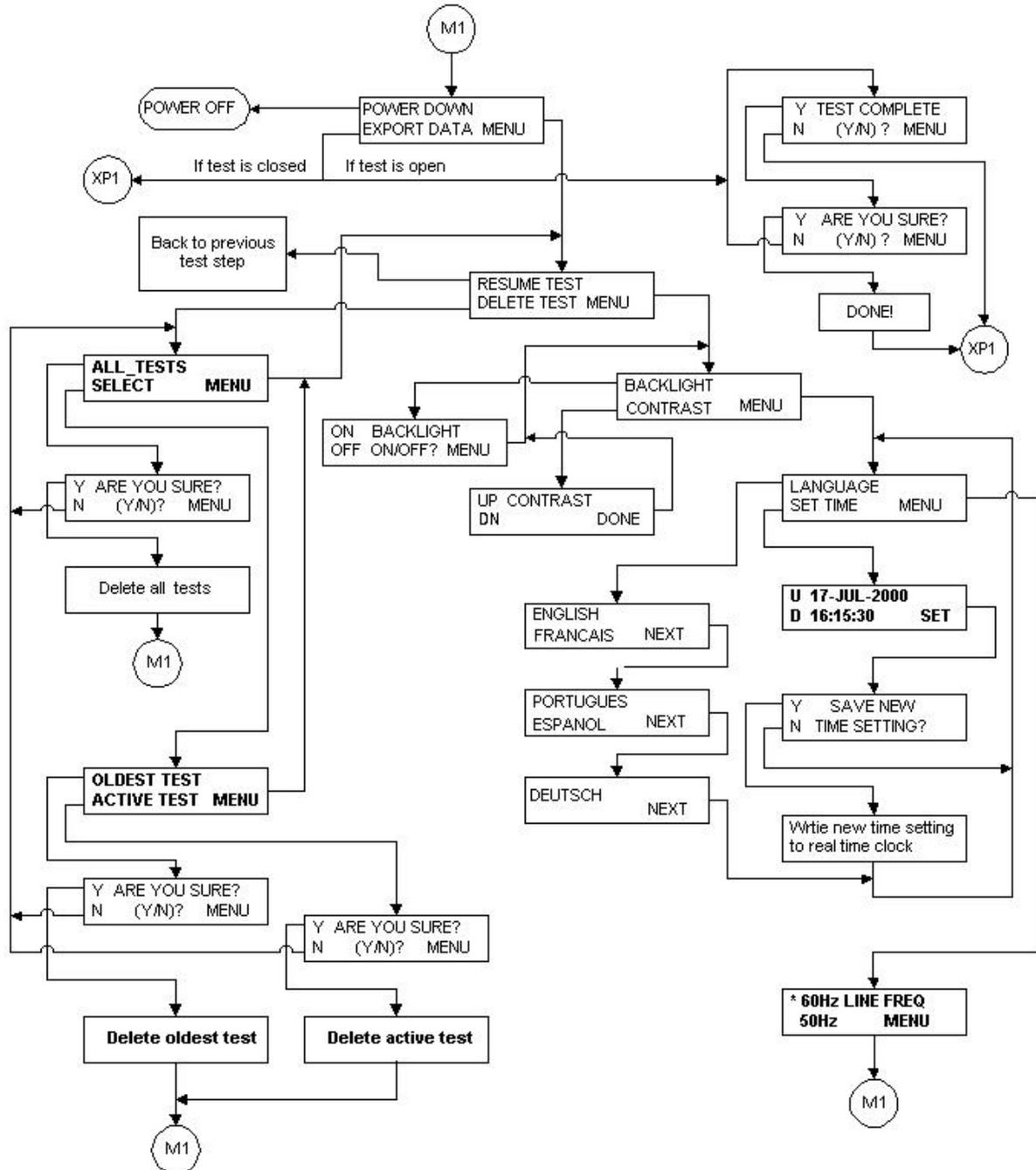
Figure 3-6: Flowchart for Receiver menus (cont'd)
