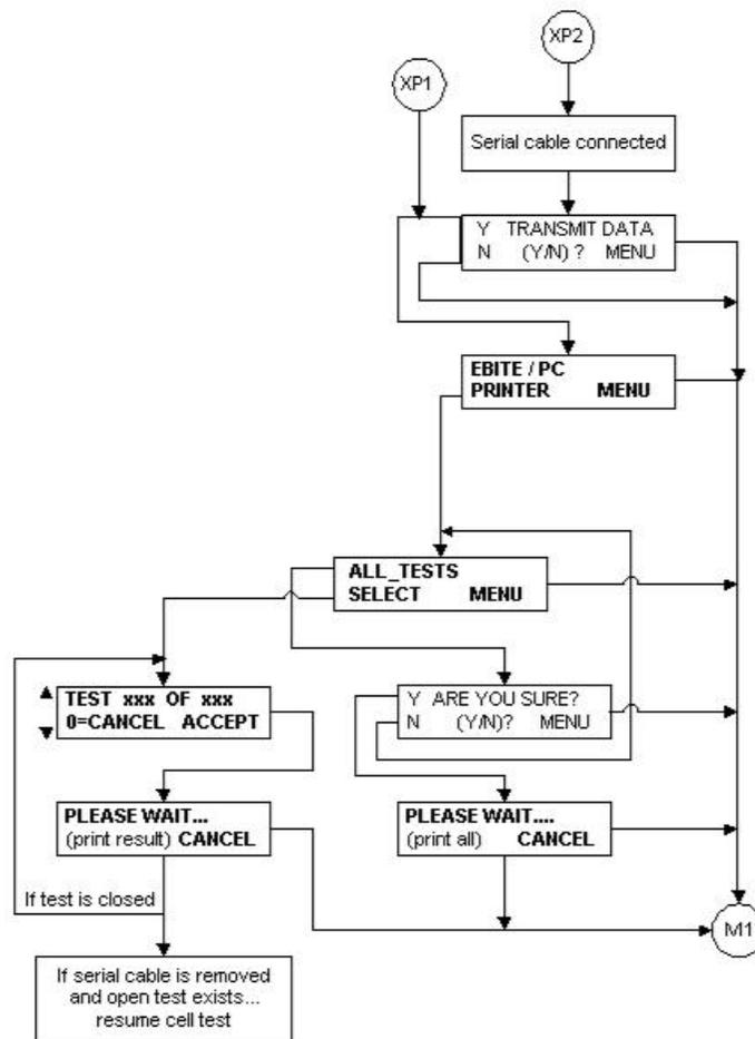
Figure 6-2: Printing test results
