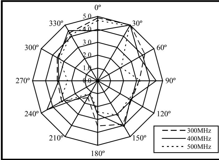
Antenna gain vs Frequency
