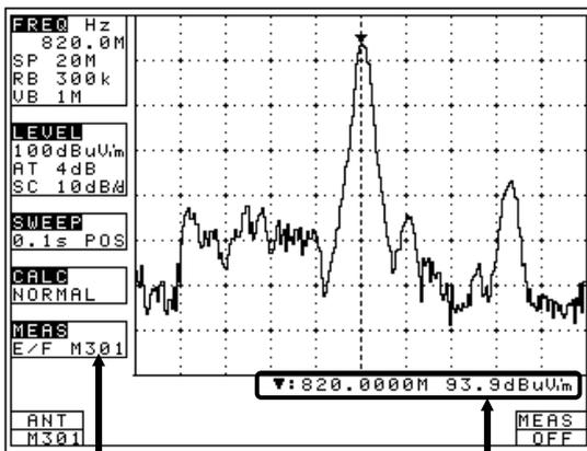
[Electric field strength measurement mode]
