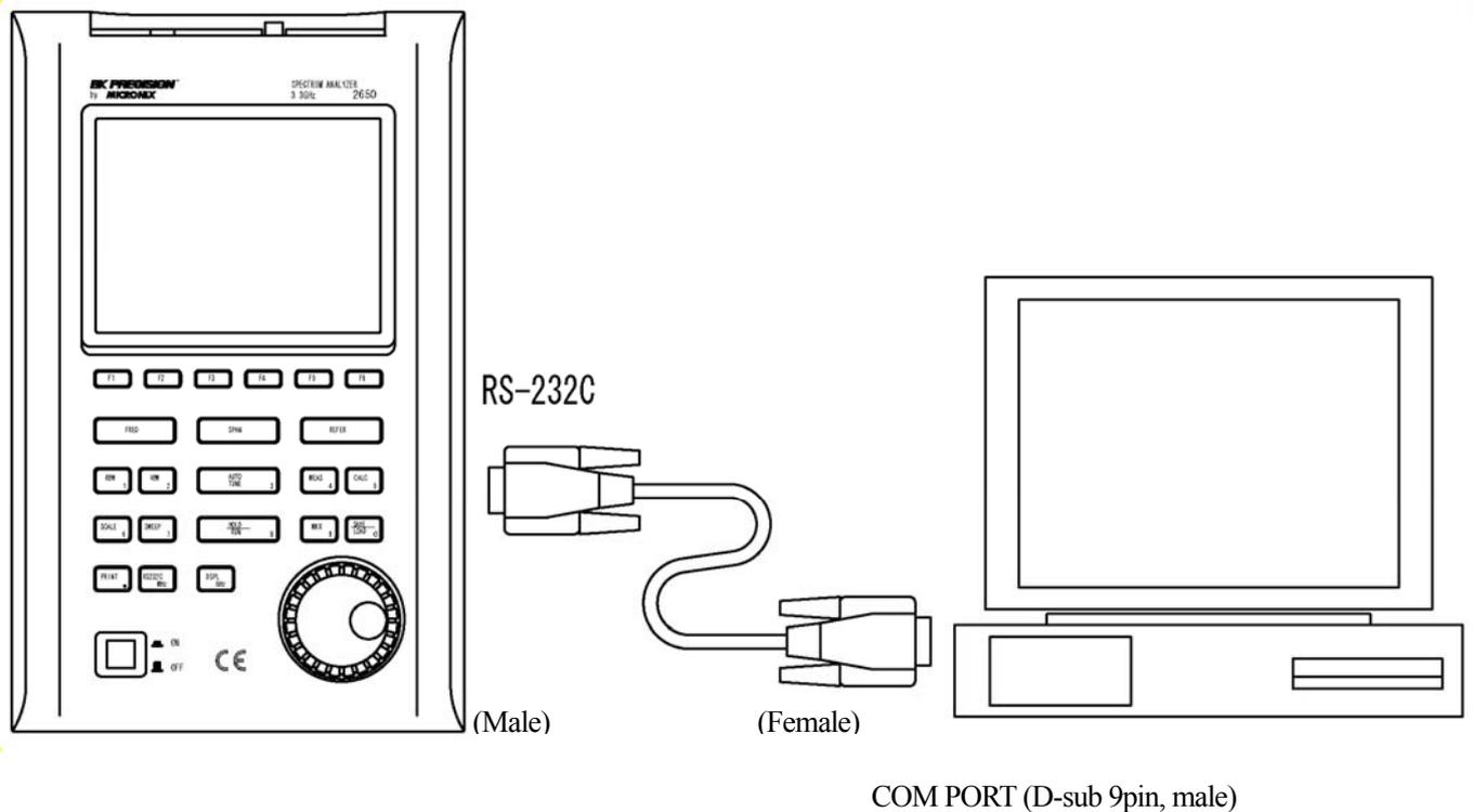
\*Use the conversion connector, in the case that is D-sub 25pin (male)
