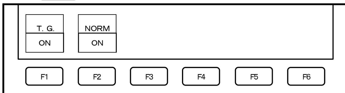
2. Each time **F1** is pressed, the T.G. output is alternately switched to ON or OFF.
