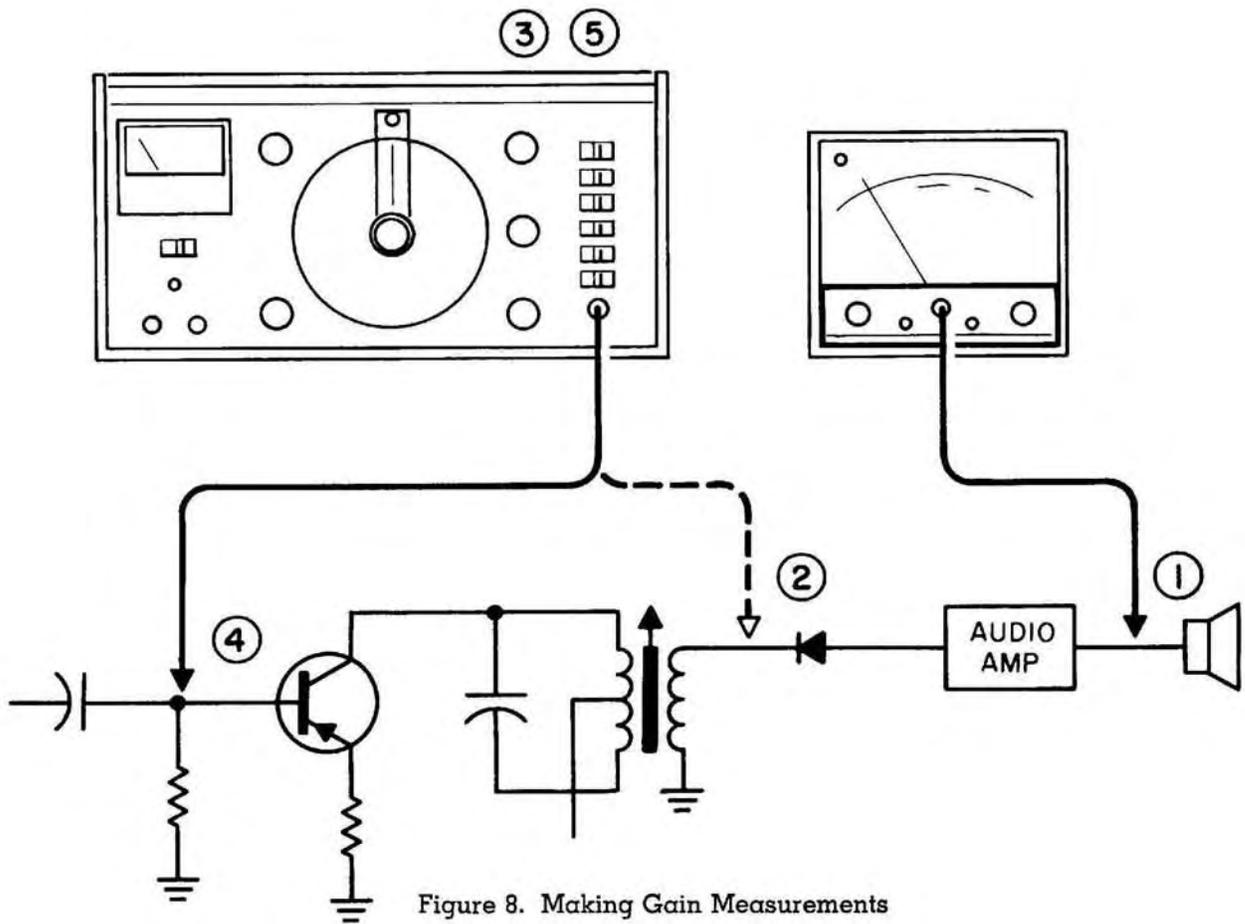
Figure 8. Making Gain Measurements
