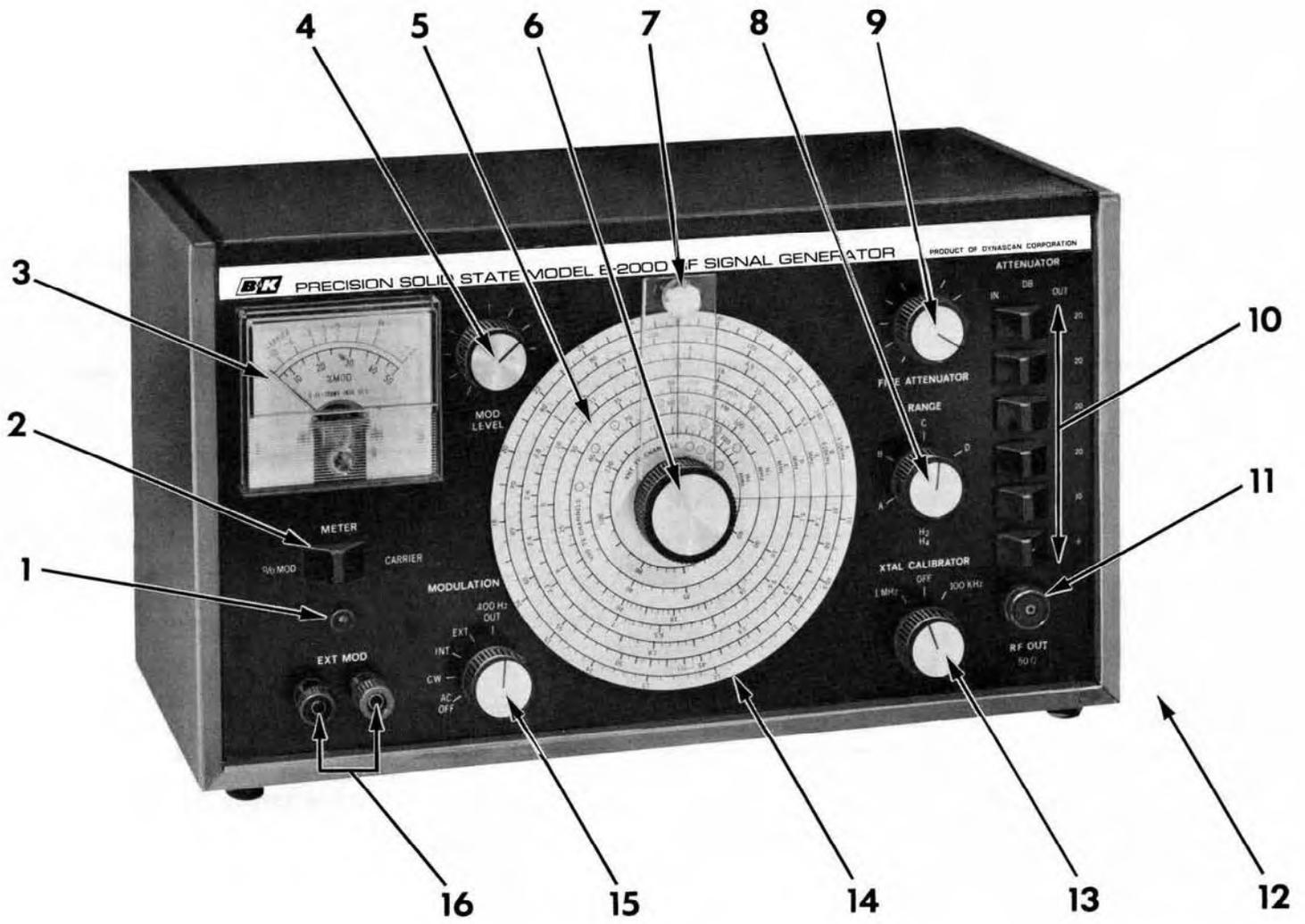
Figure 1. Operator's Controls and Indicators
