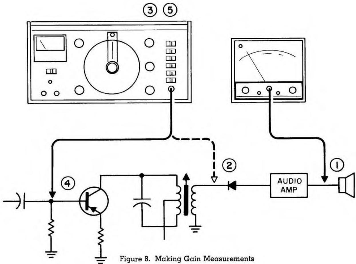
Figure 8. Making Gain Measurements
