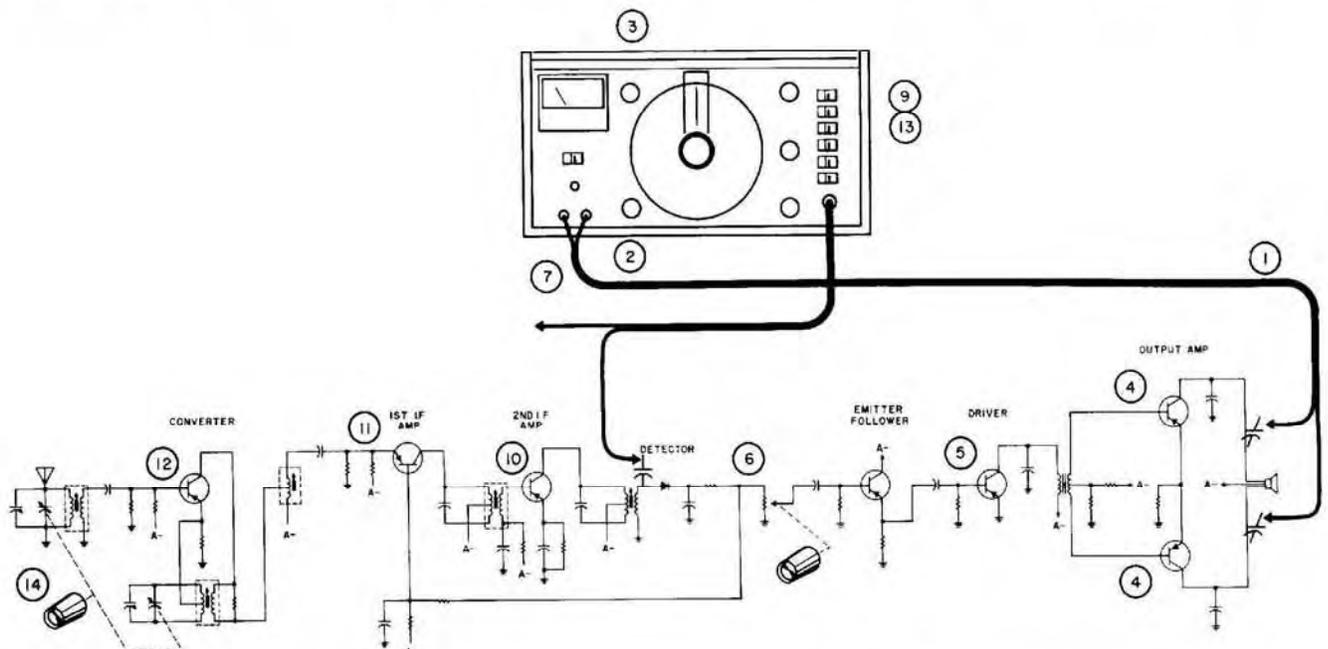
Figure 7. Typical Troubleshooting Technique Using RF Signal Generator
