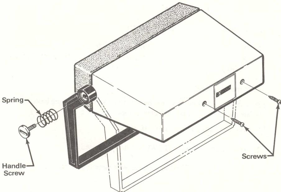
Fig. 14. Removal of rear case from Model 1820.
