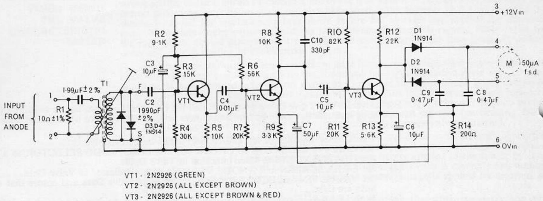
FIG. 4 AMPLIFIER CIRCUIT DIAGRAM
