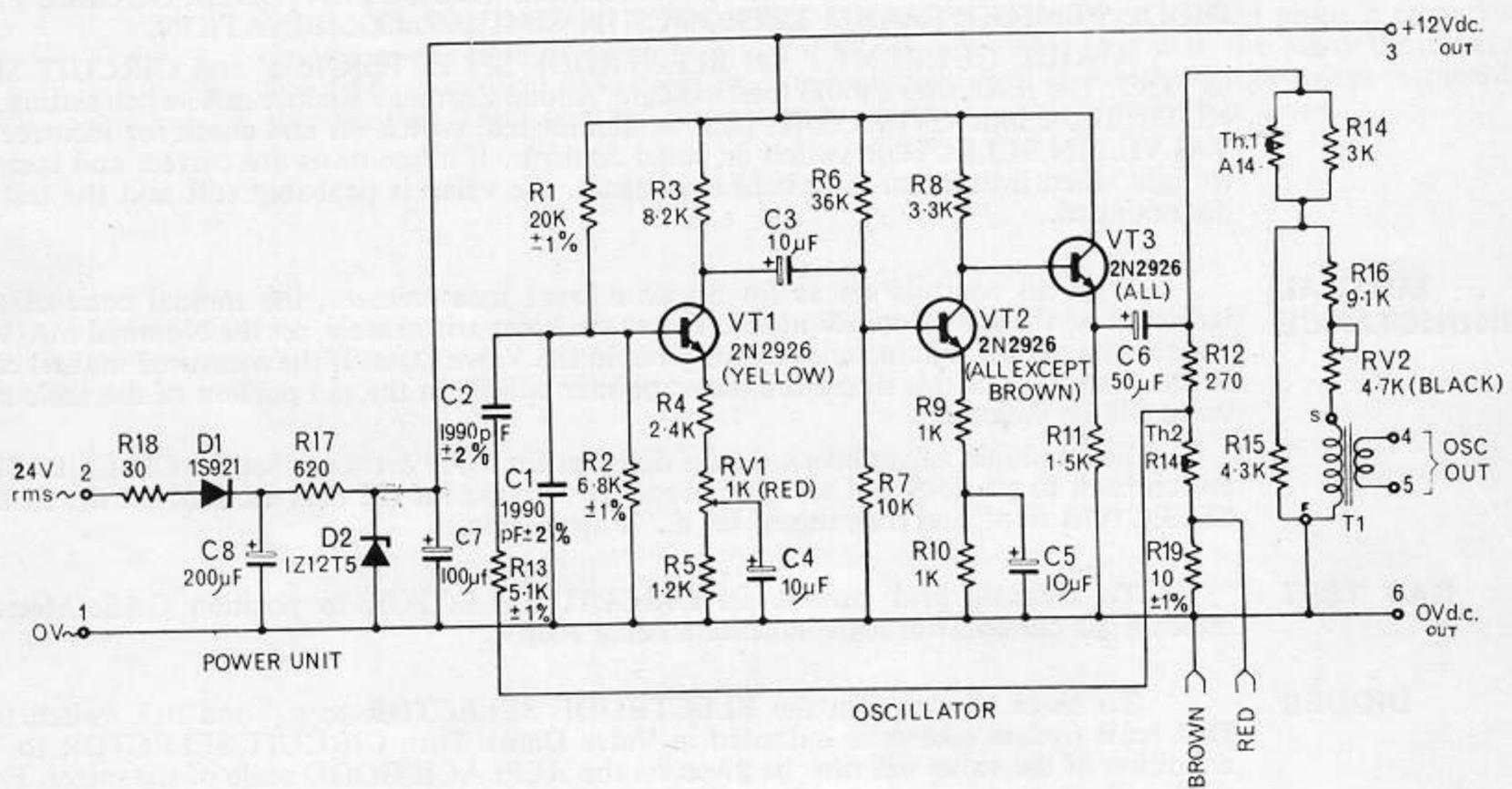
FIG. 5 OSCILLATOR AND POWER UNIT CIRCUIT DIAGRAM
