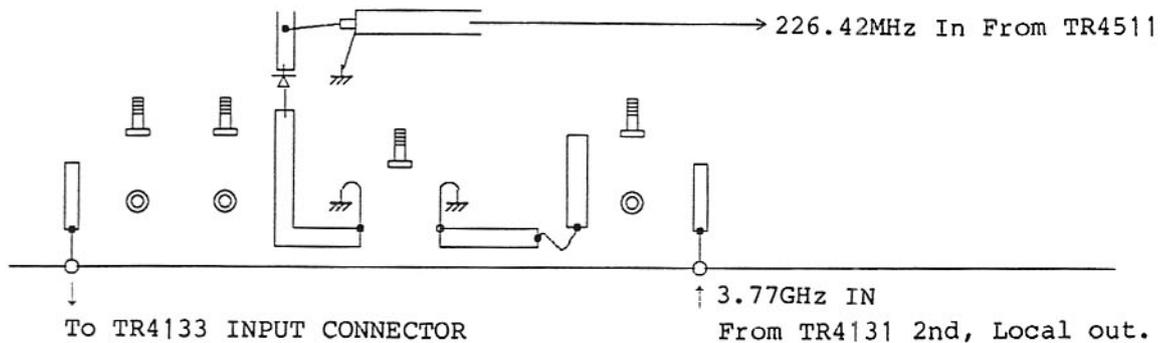
Figure 7-2 Adjustment of 4.0 GHz BPF
