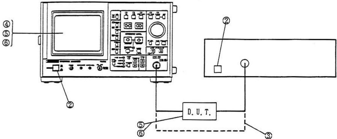
Figure 2-3 Procedure for Reading the Frequency Characteristic Directly
