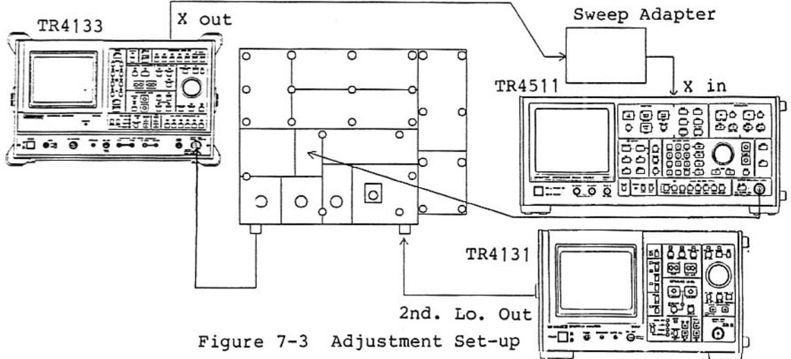
Figure 7-3 Adjustment Set-up
