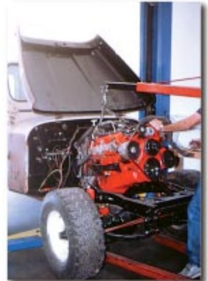
When mounting the block into a Jeep, it is recommended to remove the grille and fenders for ease of installation.
