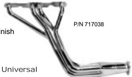
**GEN III CHEVY V8 HEADERS:** The Chevy Gen. III headers are welded to a 3/8" steel flange. These headers use the stock flange gasket and metric bolts. We provide two collector rings for the exhaust shop and the collector gaskets. All headers can be ordered in a chrome finish or a non plated finish by adding a (NP) to the numbers listed below.
