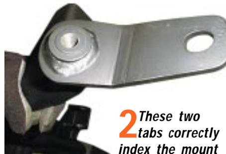
**2** These two tabs correctly index the mount into the frame.
