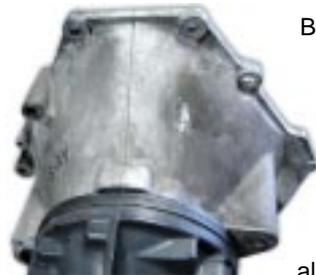
Before disposing of the old AX5 transmission, you will need to retain the shifter housing from that transmission. You will also be using the stock 4 cylinder bellhousing, the stock release arm, and crossmember mount.
