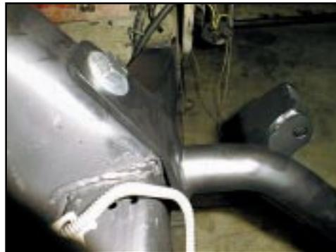
**1** This is the mount bolted to the passenger side shock tower.
