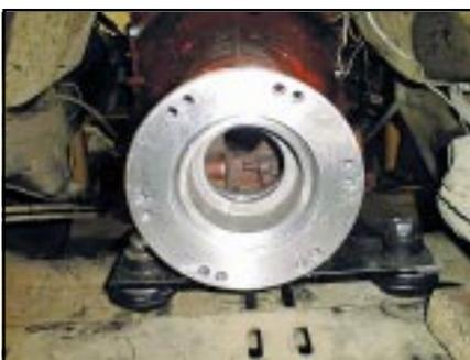
**8** The Atlas will bolt in one of the two rotations on the adapter. We rotated ours almost flat to give us optimum ground clearance.
