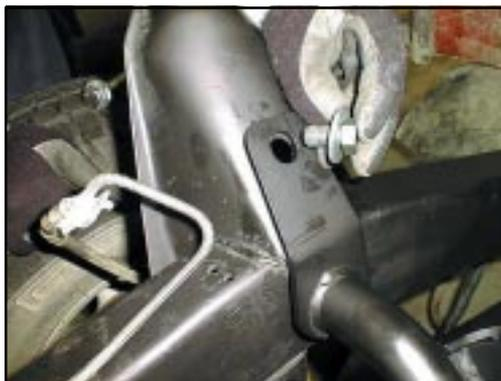
**4** Installation of the upper frame bolt. (Note the removal of the shock to access the nut from the outside.)
