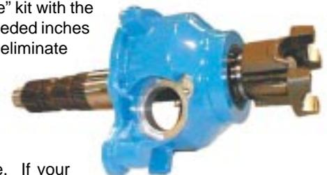
The installation of this kit requires you to nearly disassemble the entire transfer case. If your transfer case is in need of a rebuild, now is the perfect time to do it.
