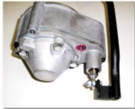
Both above photos illustrate the shift rod installation on the Saturn Overdrive. The shift rod must remain in close proximity to the overdrive unit for proper floorboard clearance. The configuration of some of the shifter rods are to avoid transfer case shifter lever interference.
