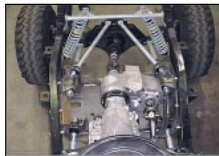
**9** The transmission, adapter, and Atlas are a fairly short combination with an overall length of 38.1". This allows for a 22.5" driveshaft in the rear and a 31" shaft in the front.
