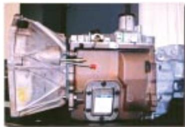
If the overall length is not a concern or you're looking for the easiest adaptation, we also offer a complete line of adapter plates for these transmissions. The adapters are all based around the Dodge transmission and the length of the Dodge input shaft. The Dodge transmission input shaft has a stickout length of 7-1/2". This allows us to use an adapter plate and then couple it to the stock AMC bellhousing.
