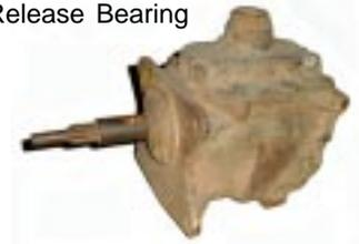
**AMC TH400** (1972-79) - This transmission can be identified by a case length of 24.250". In 1972, this transmission was introduced into the Jeeps; however, this early transmission used a cast iron adapter plate to fit this tranny to the AMC block. *We manufacture an adapter to mate only the 1974 & newer transmissions to the Chevy blocks.*
