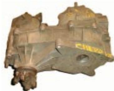
We also offer a kit, [P/N 50-2501](#), to adapt the 700R4 to the Quadra-Trac transfer case. Since this transfer case is a full-time 4WD unit, the front yoke is normally a C.V. style. If installing a 700R to this transfer case, the C.V. yoke may cause interference. The easiest fix for this problem is to change to a standard yoke assembly. The overall length of this combination is identical to the TH400.
