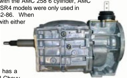
The adapter between the main case and transfer case is 5-7/8". The input shaft has a stickout length of 7-1/16", and a pilot tip diameter of .590", which is identical to all Chevy transmissions. The input shafts on these transmissions are normally 1-1/8" 10 spline; however, in some 1986 applications we have found a 1"-14 spline. These applications will require a special clutch disc, [Part No. 716104](#).
