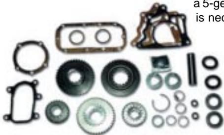
3.15:1 low gears, [Part No. 418315OD](#). We also offer just the Saturn Overdrive bowl gear if you have already obtained your low gear set, [P/N 911098](#).
