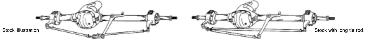
The Saginaw steering system requires the elimination of the stock gear box and bellcrank. The new steering box is mounted on the inside of the left front frame rail, just behind the bumper. Although this sounds simple, there are several things that must be considered before the installation can be completed. Such things include:
