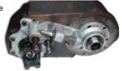
Another option for the Dana 300 transfer case is a twin stick shifter. Our twin stick application requires the installation of two new shift rails. This kit is a securely mounted assembly off of the stock aluminum shifter housing. The new shifter rod allows a heim joint linkage for a smooth, positive shifter motion.
