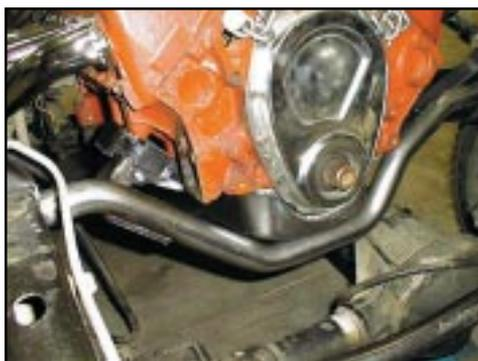
**6** The engine is bolted in using the stock GM mounts provided by Advance Adapters.
