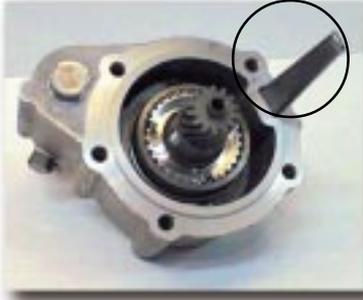
6. Install the oil scoop into the case assembly (Fig. 4). **NOTE: Be sure the oil scoop is in place. Failure to install this scoop will cause lack of proper oiling and eventual overdrive failure.**
