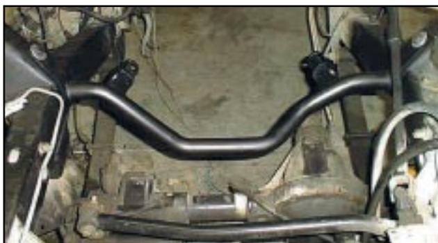
**5** Both sides are in place and are ready for the engine and transmission to be dropped in. Take care that the mounts are positioned so that they are behind the crossmember.
