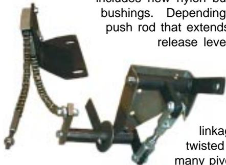
One of the biggest problems with the stock Jeep clutch linkage is its reliability on the trail. Most Jeep owners have either experienced or seen the stock linkage fall apart when a vehicle is tweaked or twisted while 4-wheeling. The linkage has too many pivoting and non-secured points and, when put under stress, they tend to come undone.
