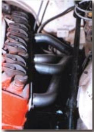
Most stock manifolds will require the exhaust system to be routed on the inside of the frame rails, while most headers will carry the exhaust on the outside of the frame rails. We offer both fenderwell & inside-the-frame rail headers.
