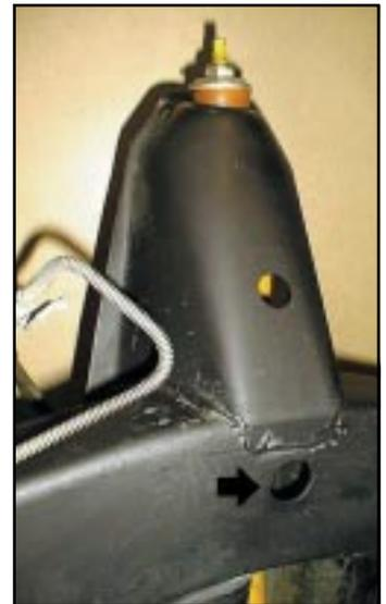
**3** These are the stock frame holes used by Advance Adapters. The lower hole is used to bolt the cradle from the outside of the frame.
