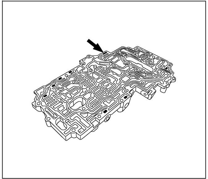
13. Install the check valve NO.1(9), ball(8) and check valve NO.2(7) to valve body.
