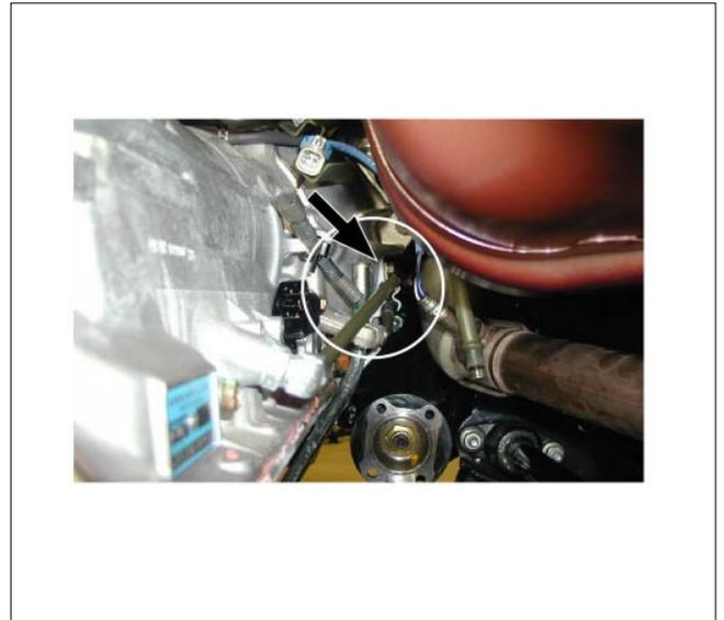
19. Install the transfer case assembly. (4WD only)
