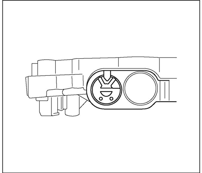
3. Install the cut back valve(29), spring(28) and plug(27) into the bore.
