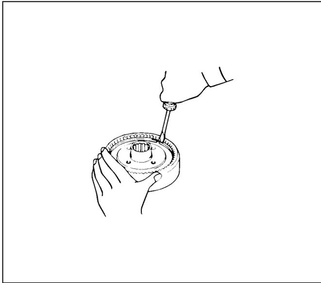
13. Remove ring gear flange from OD planetary ring gear.
