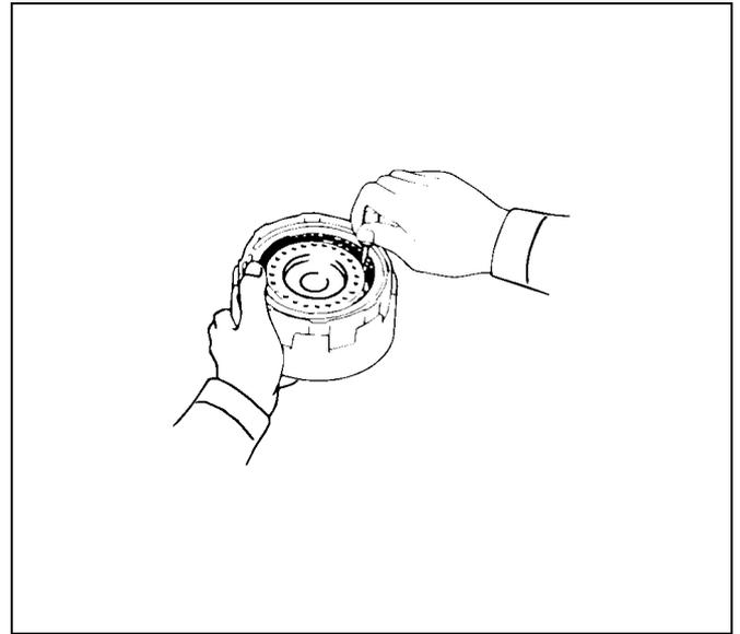
17. Align the spline of the front planetary gear with the flukes of the discs and install the front planetary gear to the forward clutch.
