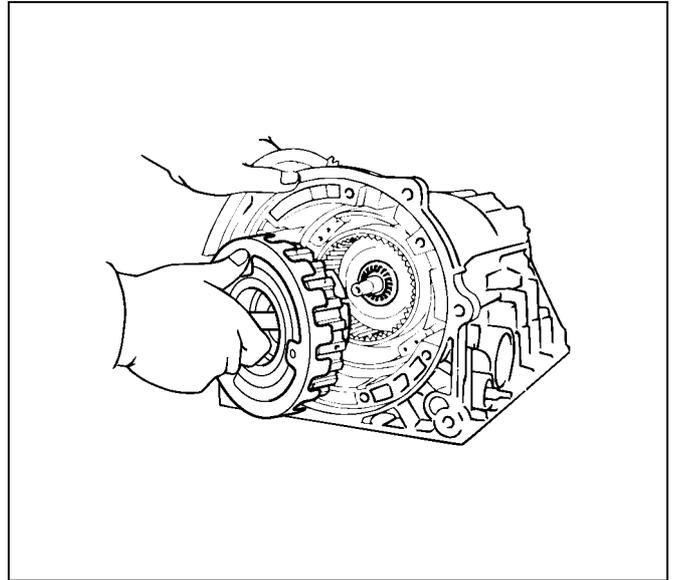
4. Remove the race from OD planetary gear.
