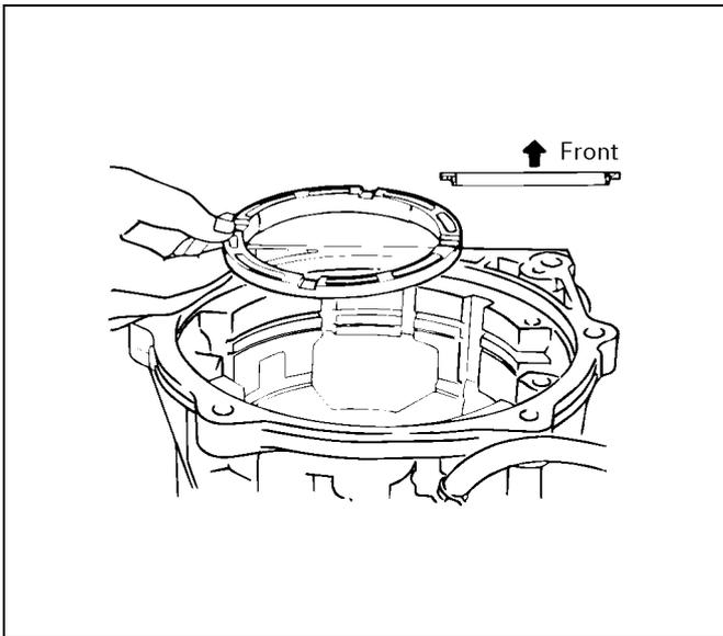
6. Install one-way clutch in the transmission case.
