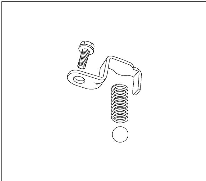
14. Install the accumulator sub-assembly (8) and clamp(7) to the valve body.
