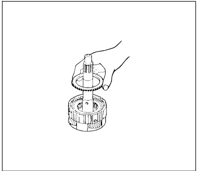
17. Remove OD one-way clutch with outer race.
