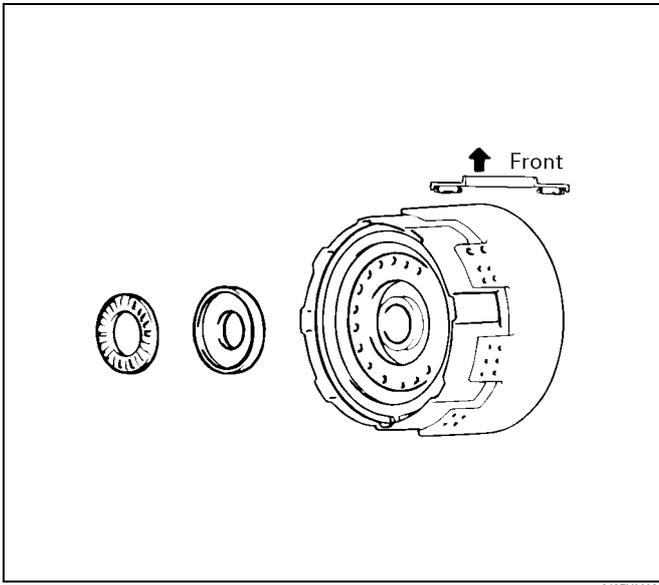
16. Coat the race with petroleum jelly and install it onto the front planetary ring gear.
