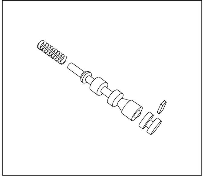
10. Install the retainer(14) by pushing the plug.
