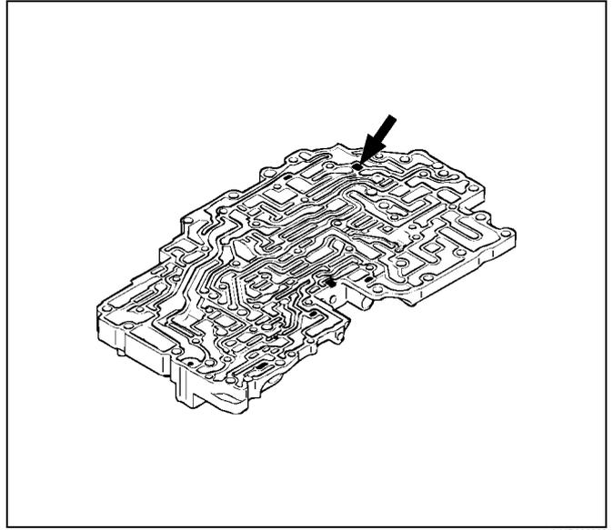
9. Install the low coast modulator valve(18) and spring(17) into the bore.
