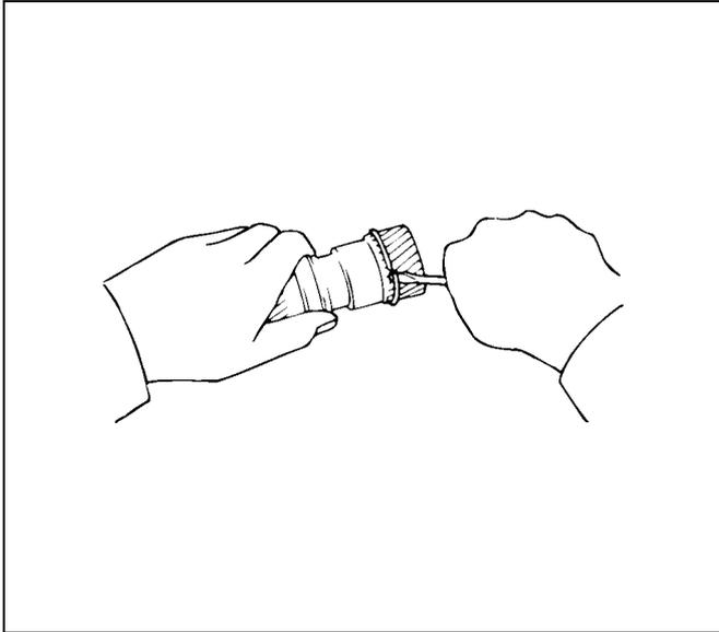
2. Place a wooden block, etc. as a work stand and place the planetary sun gear onto it. Install the sun gear input drum onto the planetary sun gear.
