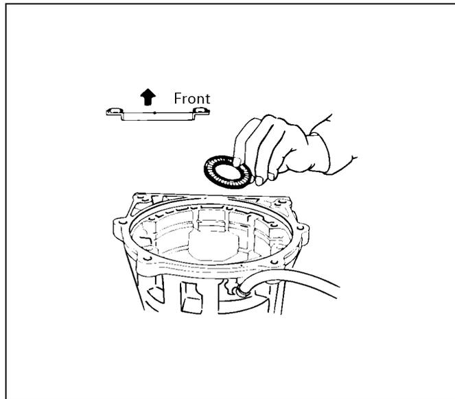
2. Install the rear planetary gear, second brake drum and output shaft.
