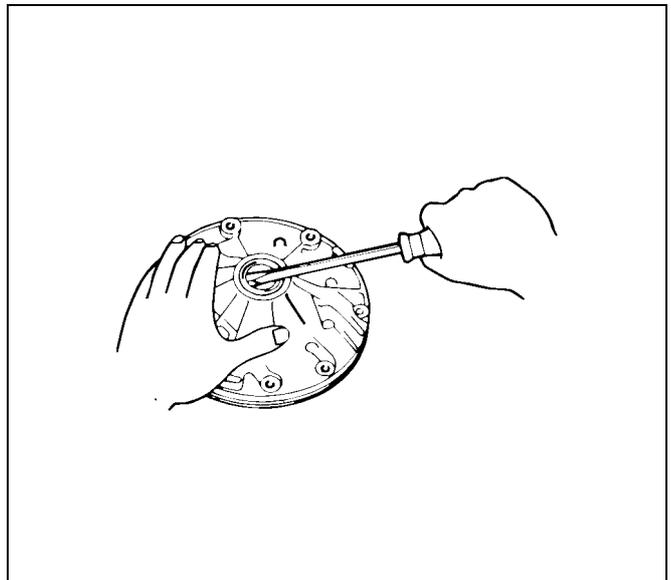
Using special tool, install a new oil seal.
