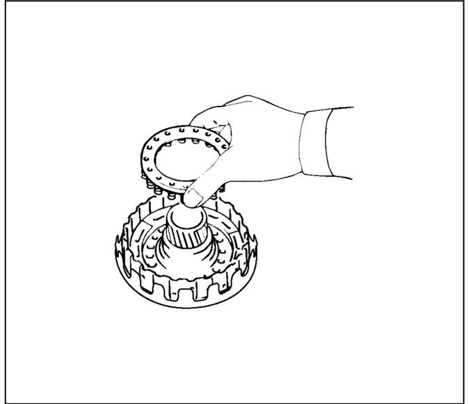
12. Place special tool on the spring retainer, and compress the return spring.
