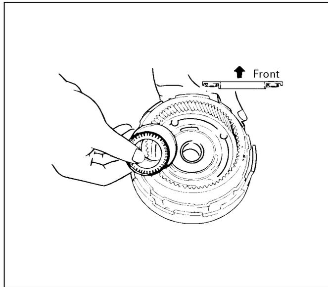
19. Install the assembled direct clutch, forward clutch and front planetary ring gear into the transmission case.
