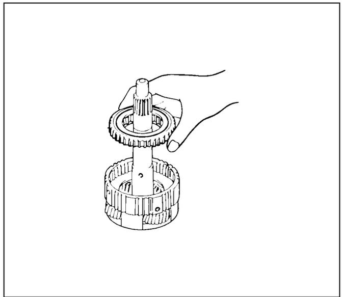
18. Remove the thrust washer.
