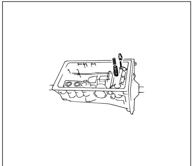
8. Remove the accumulator piston (B-2).
