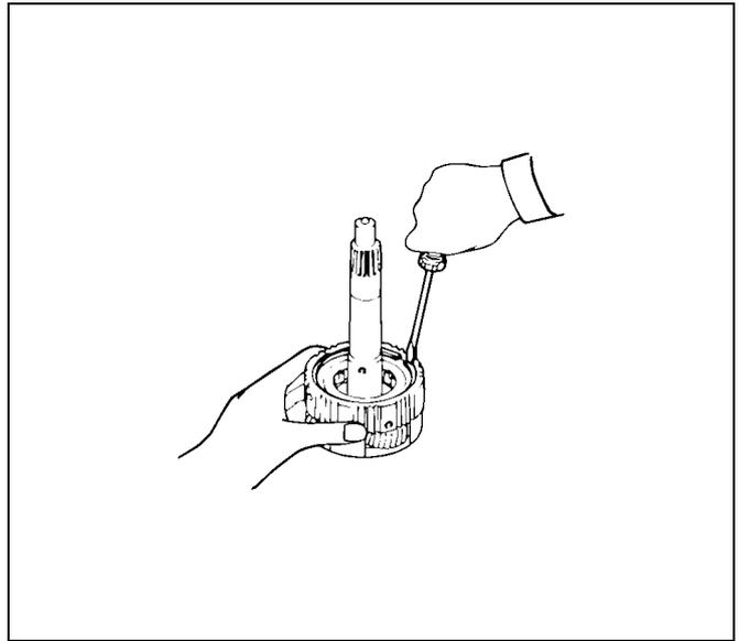
16. Remove retaining plate from OD planetary gear.
