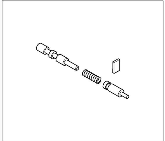
4. Install the retainer(26) by pushing the plug.
