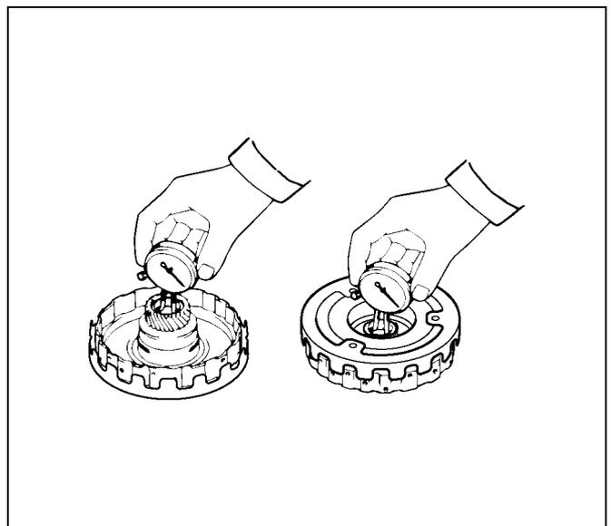
5. Check OD planetary gear bushing.
