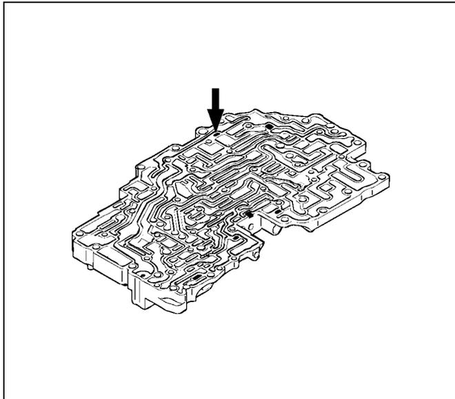
13. Install the ball(11), spring(10) and retainer (9) to the valve body.
