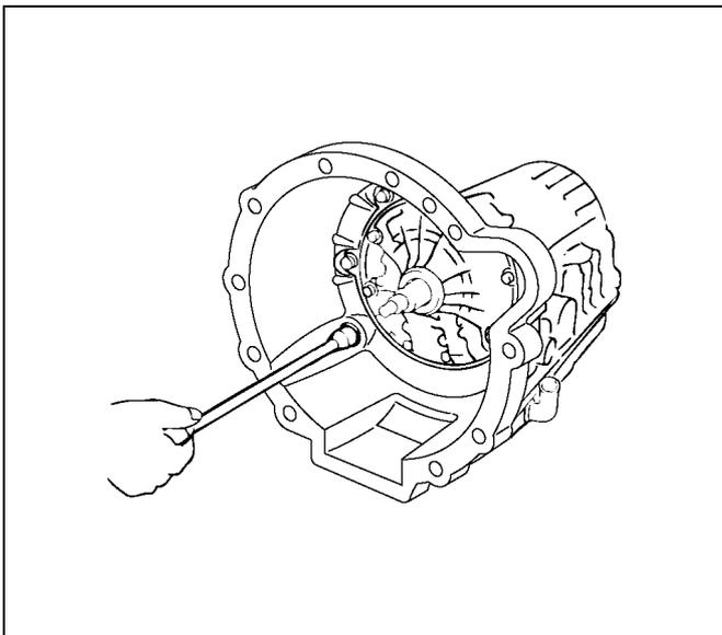
2. Install the snap ring, key and rotor (4×2).
