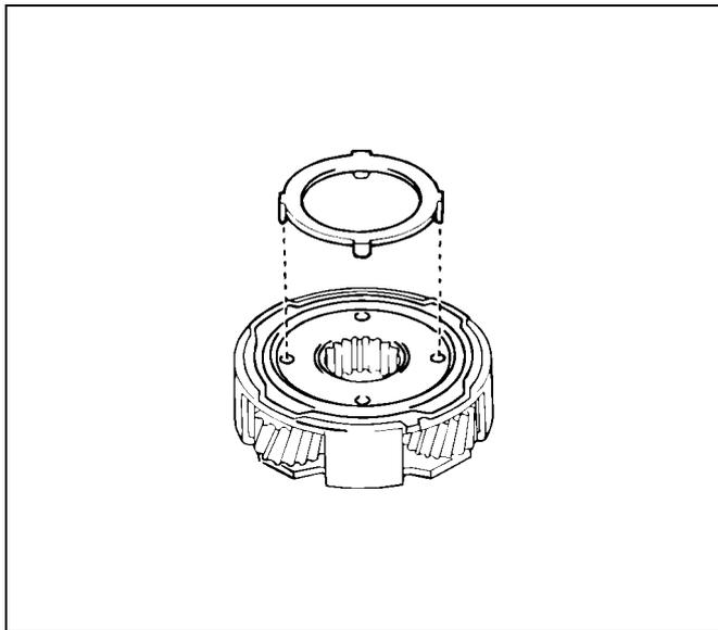
3. Coat the race and thrust bearing with petroleum jelly.
