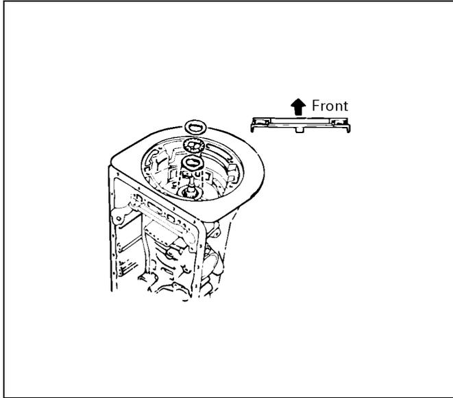
31. Install the overdrive planetary ring gear.
