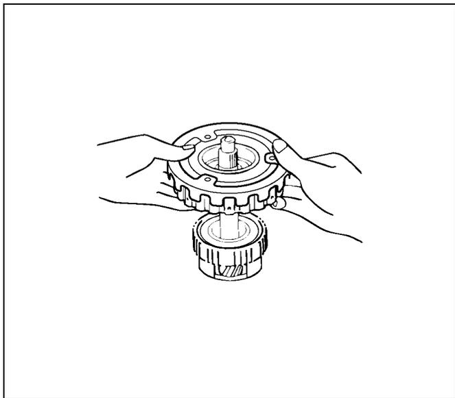
18. Check operation of one-way clutch
