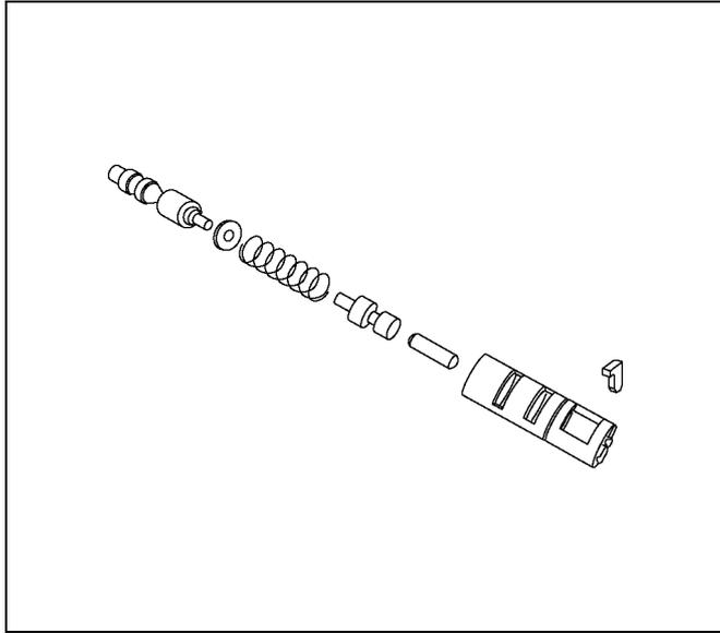
2. Install the retainer(30) by pushing the sleeve.
