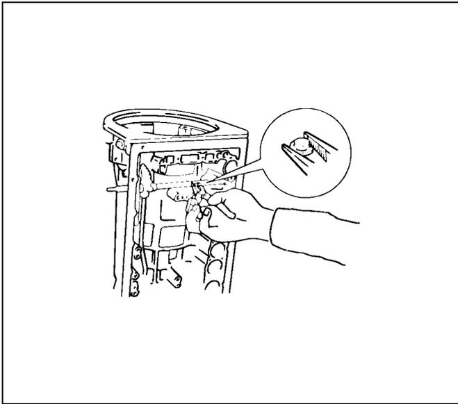
15. Coat the bearing and race with petroleum jelly and install them onto the forward clutch.
