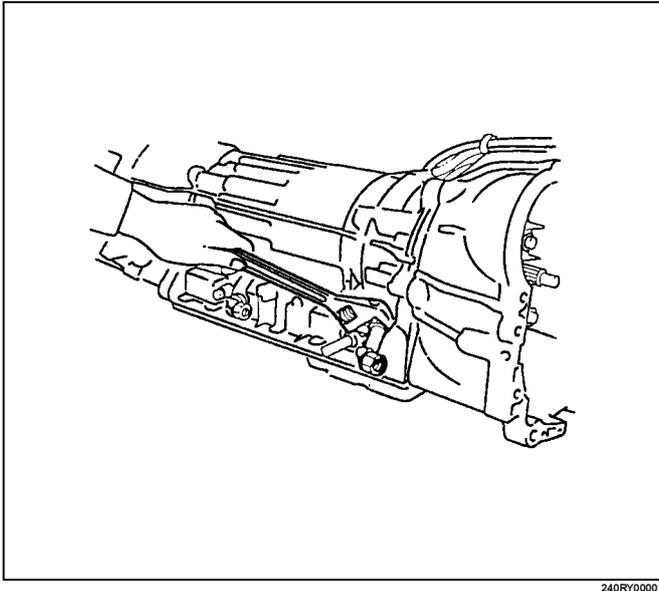
5. Remove the oil temperature sensor.
