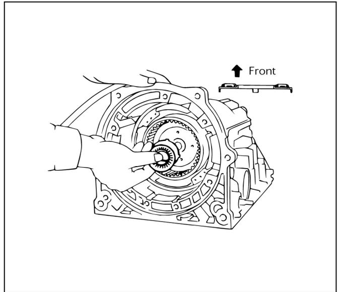
Install the (flat ring) 4.0 mm (0.157 in) thick flange with the rounded edge side of the flange facing the disc.
