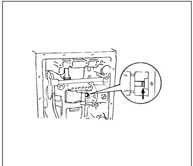
14. Using snap ring pliers, remove the snap ring.
