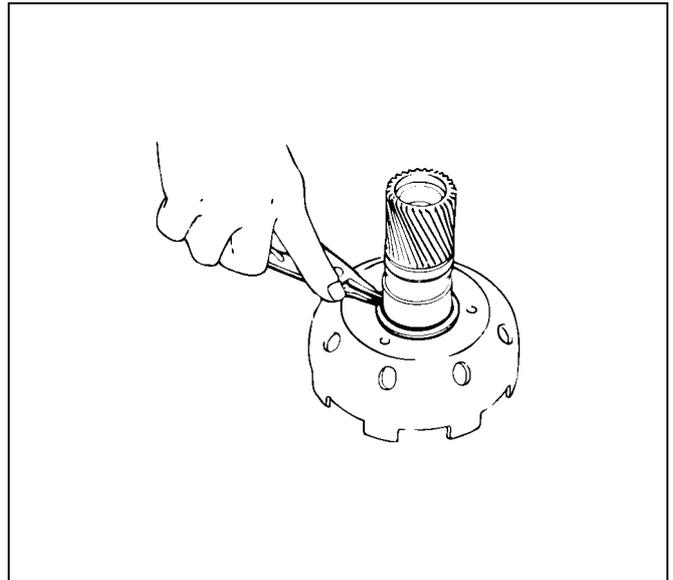
4. Coat the two oil seal rings (metal) with ATF. Install the two oil seal rings onto the planetary sun gear.
