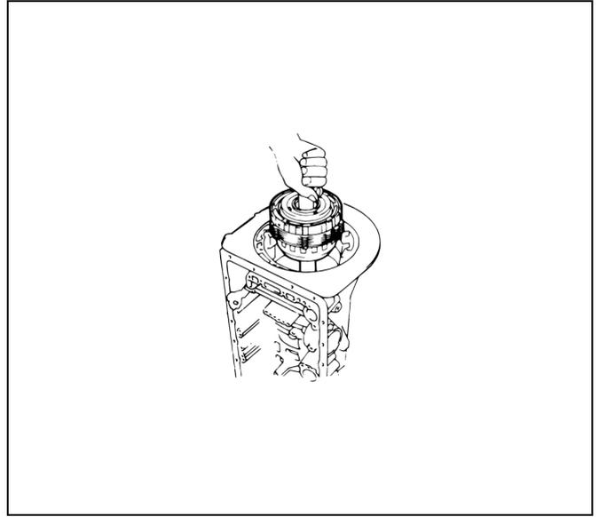
30. Remove the assembled thrust bearing and race from the transmission case.
