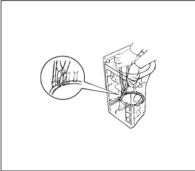
29. Remove the rear planetary gear, second brake drum and output shaft as an assembly.
