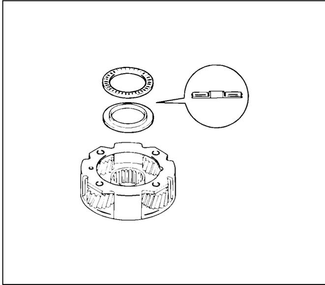
2. Turn over the planetary ring gear and install the race (metal).
