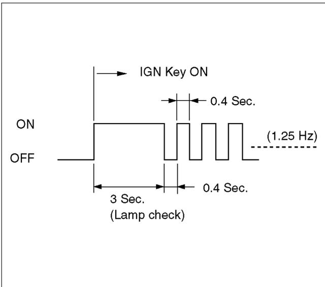
2. Indicator is flashing and the flash is 0.4 seconds ON and 0.4 seconds OFF always when ignition is on (engine cranked or not). This means that there is a malfunction. Go to **DIAGNOSTIC CHECK**.
