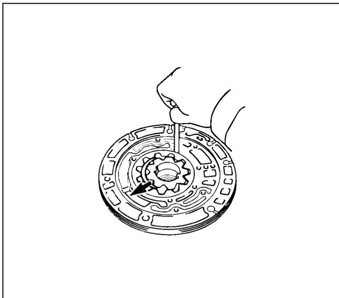
5. Check side clearance of both gears.
