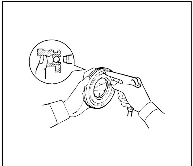
4. Check OD direct clutch drum bushings.
