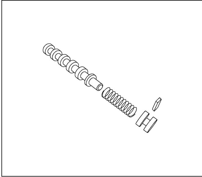
11. Install the spring(13), secondary regulator valve(12) and plug(11) into the bore.
