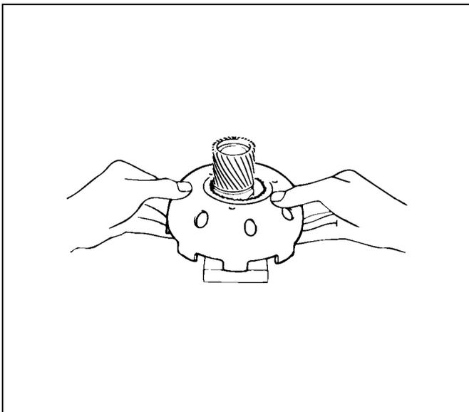
3. Install snap ring with snap ring pliers.
