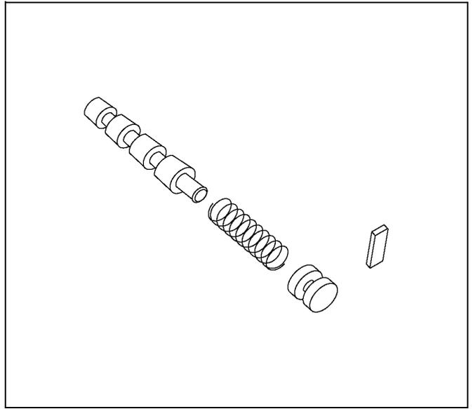
12. Install the retainer(12) by pushing the plug.
