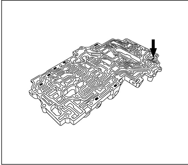
17. Remove the sleeve(31) with the plunger(32), spring(33) and lock-up relay valve(34). Remove the lock-up relay valve(34), spring(33) and plunger(32) from the sleeve(31).
