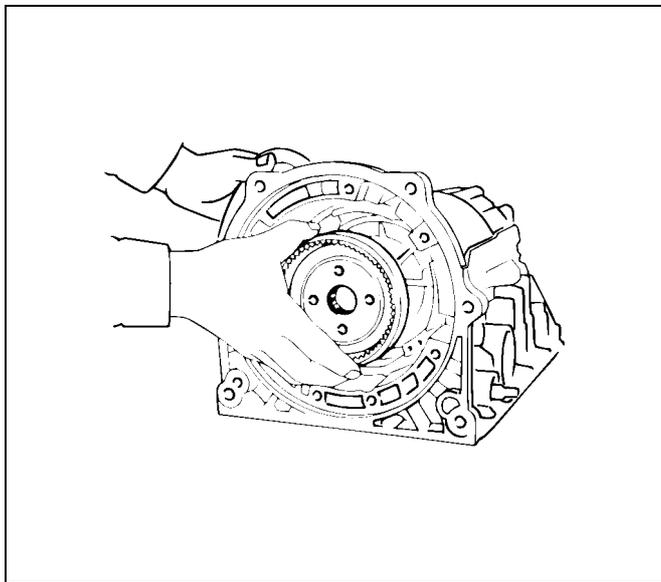
32. Coat the bearing and race with petroleum jelly and install them onto the planetary ring gear.
