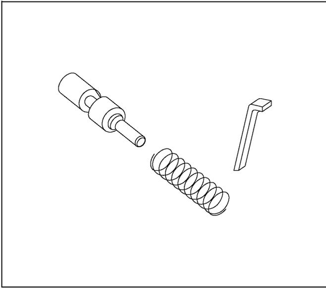
11. Install the 1-2 shift valve(15), spring(14) and plug(13) into the bore.
