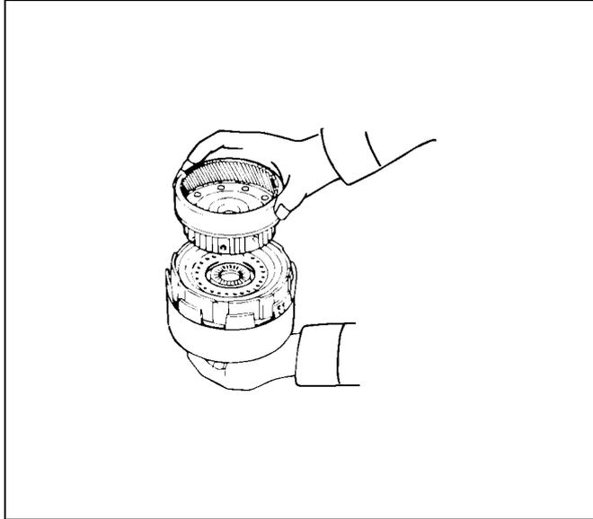
18. Coat the bearing and race with petroleum jelly and install them onto the ring gear.
