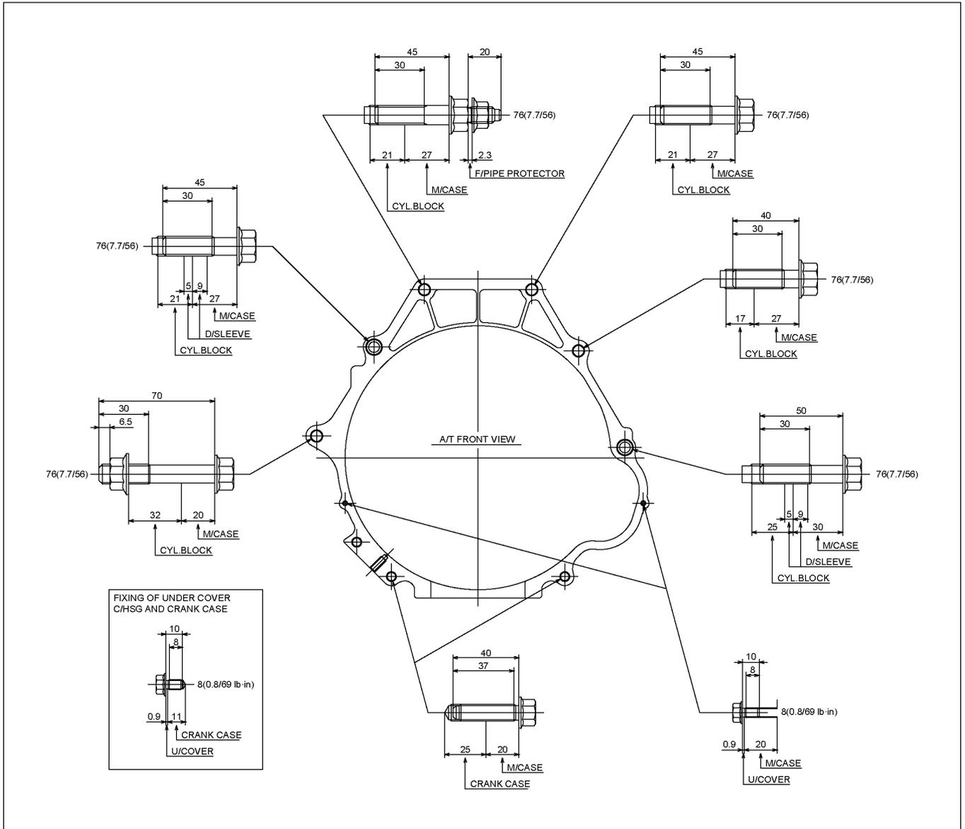
3. Install the protector and fuel pipe bracket.
