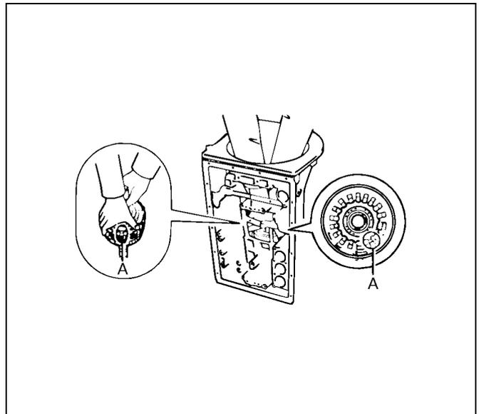
3. Using snap ring pliers, install the snap ring.
