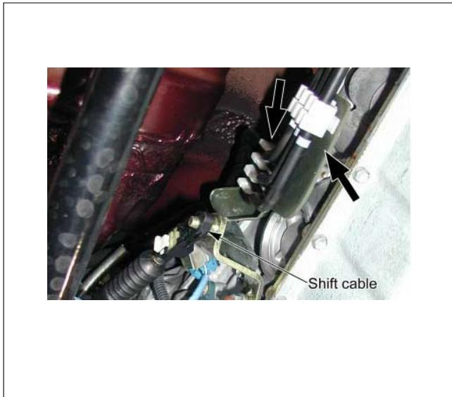
15. Connect the transmission harness connectors and clips.
