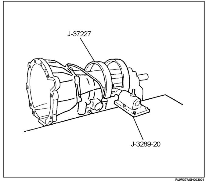
4. Remove the two elbows from transmission case.
