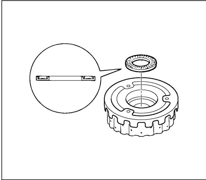
17. Align the flukes of discs in the direct clutch. Install the OD direct clutch assembly onto the OD planetary gear.
