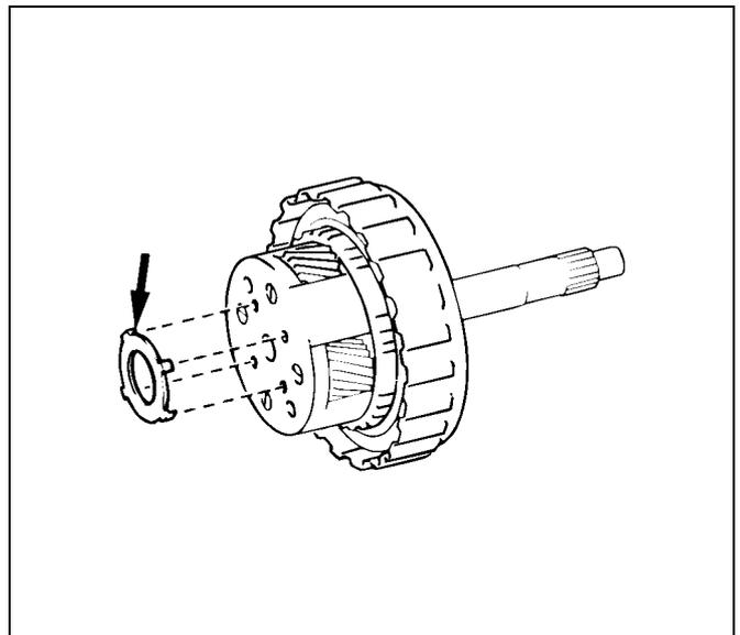
34. Install the overdrive planetary gear and direct clutch.
