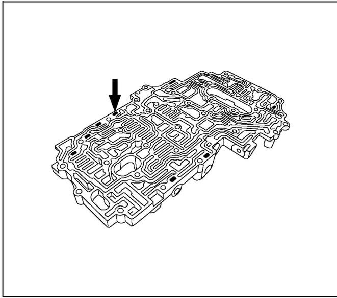
12. Install the retainer(10) by pushing the plug.
