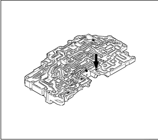
10. Install the retainer(16) by pushing the spring.
