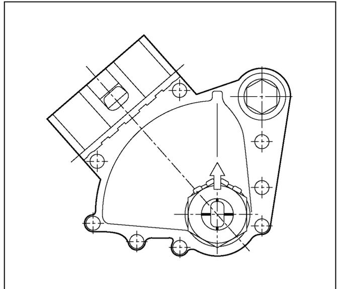
5. Install the oil temperature sensor to the transmission case.
