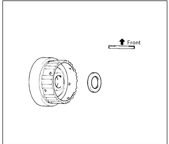
Align the flukes of the discs in the forward clutch.
