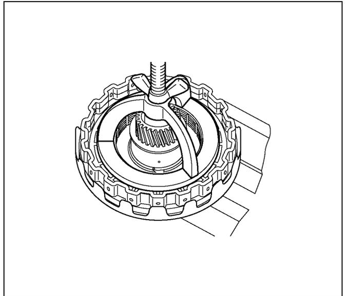
13. Install two plates and two discs then install the flange, with the flat side facing downward.
