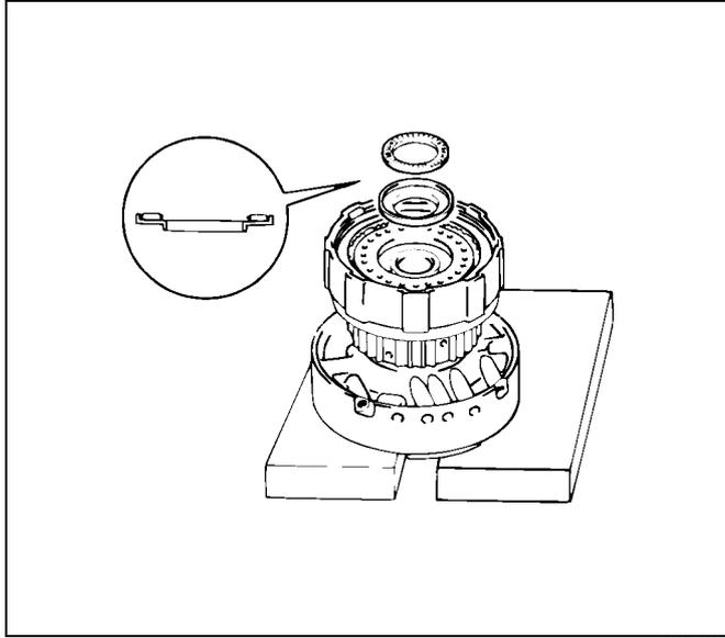
Check that the distance from the direct clutch end to the forward clutch end is 71.2mm (2.803in).
