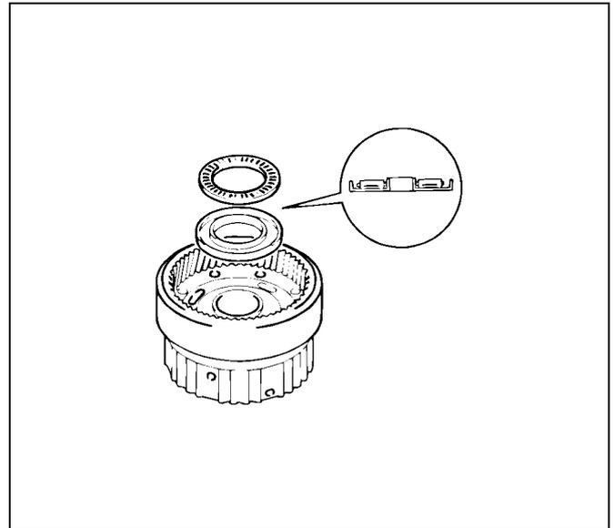
4. Turn over the planetary ring gear and install the race onto the front side of the front planetary ring gear.
