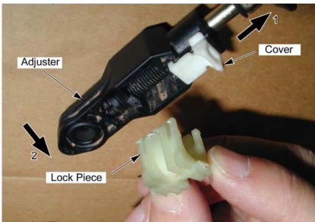
9. Connect the shift cable to the manual shaft select lever at the transmission side.
