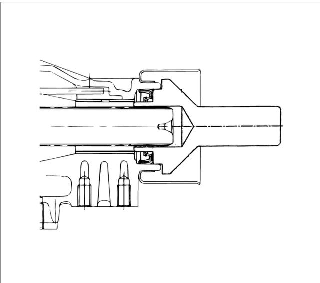
3. Install the rear propeller shaft.
