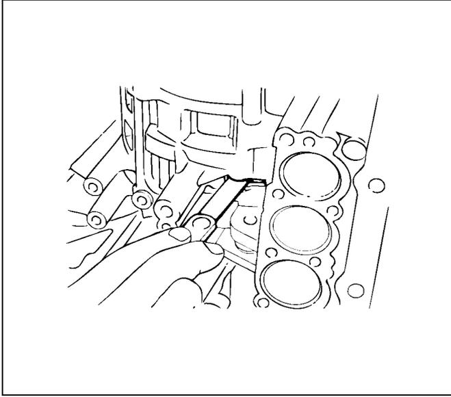
28. Using snap ring pliers, remove the snap ring.
