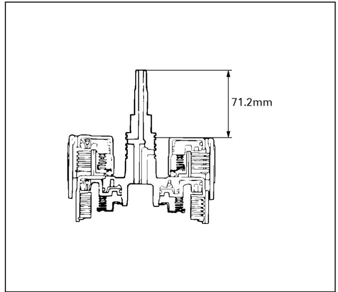
14. Align the flukes of discs in the direct clutch.
