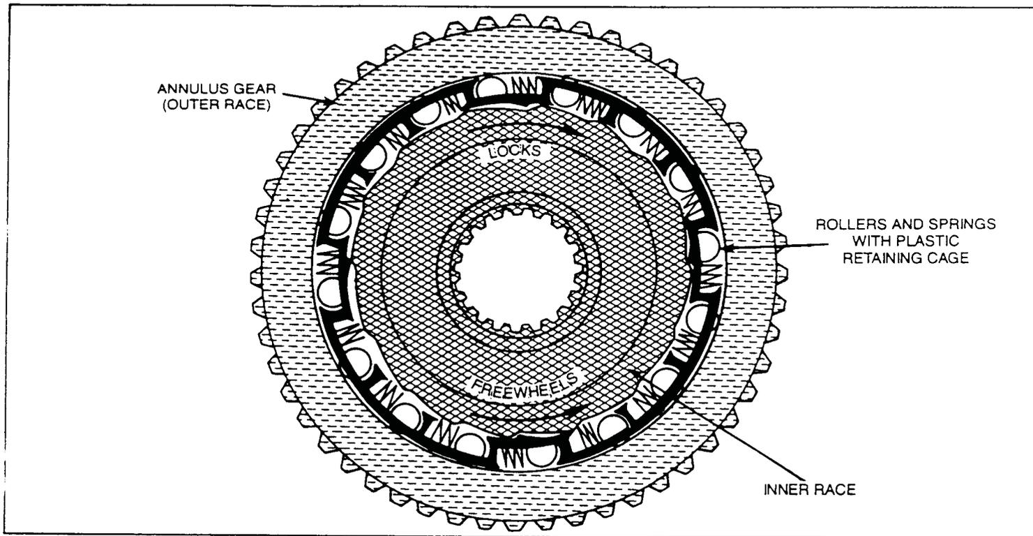
**THE OVERDRIVE OVERRUNNING CLUTCH** acts as a coupler between the intermediate shaft and the output shaft.
