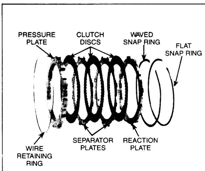
**OVERDRIVE CLUTCH:** The overdrive clutch is splined externally to the overdrive case, and internally to the sliding hub. A wire ring retains the overdrive clutch pack in the housing. This clutch is applied with the overdrive piston. When applied, the clutch holds the sliding hub from turning, as mentioned earlier.
