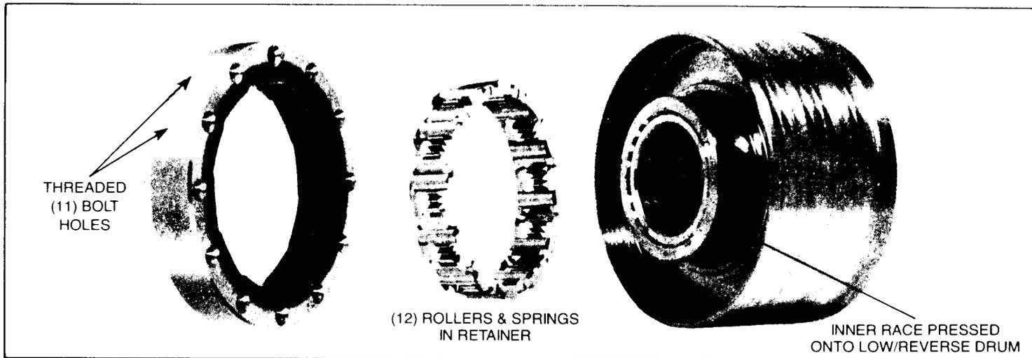
**OVERRUNNING CLUTCH:** A new overrunning clutch incorporates a spring and roller assembly with 12 rollers instead of 10. The new overrunning clutch cam has a feature that prevents the rollers from crushing the springs in the event of roller spit-back. Eleven bolts retain the cam into the
