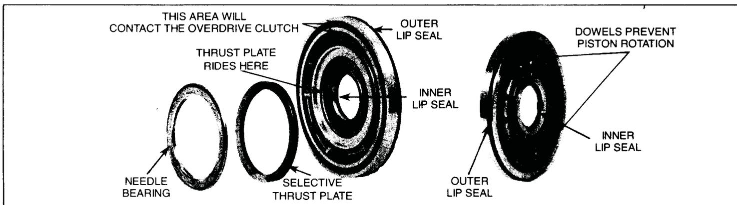
**OVERDRIVE PISTON:** The overdrive piston is located inside the O/D piston retainer. The piston seals to the retainer using two lip seals. There are no rotating seal rings and, there is no pressurized oil in the overdrive housing for the clutches. Two anti-rotating dowels on the piston prevent the piston from turning in the retainer.
