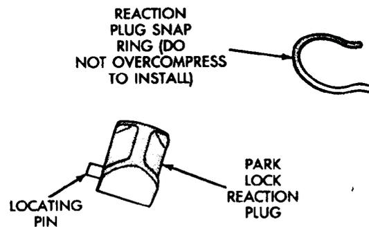
**Fig. 69 Reaction Plug Locating Pin And Snap Ring**
