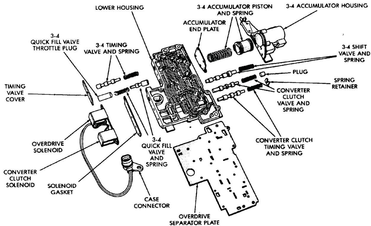
**Fig. 39 Lower Housing Shift Valves And Springs**
