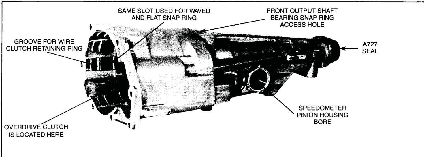
**OVERDRIVE CASE:** The overdrive case is a lightweight cast aluminum, one piece housing. The rear most part of the housing retains an oil seal and bushing, both seal and bushing are from the A-727 transmission. The left side of the hous-
