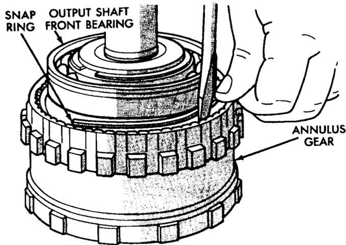
**Fig. 45 Annulus Gear And Snap Ring Installation**
