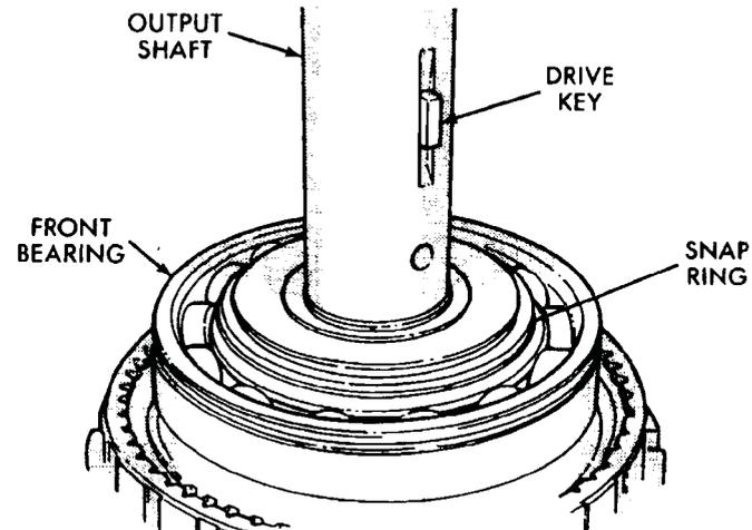
**Fig. 64 Front Bearing And Drive Key Installation**
