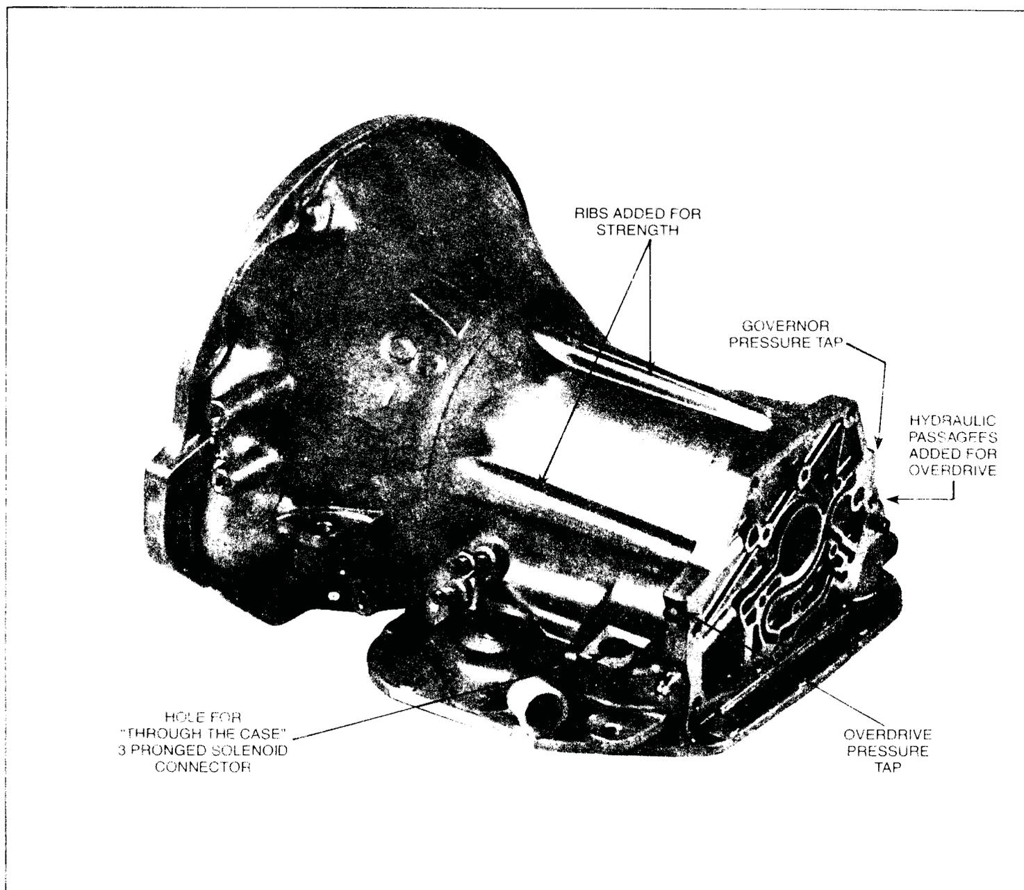
**CASE.** The transmission case has been increased in strength in several areas. The case now has ribs on the top and both sides to improve its rigidity. The back face of the case has changed because of the hydraulic circuits needed to operate the overdrive clutch piston. The mounting
