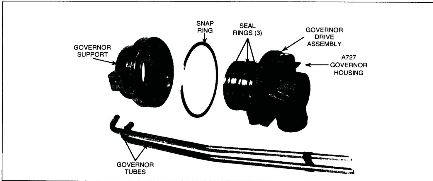
**GOVERNOR DRIVE ASSEMBLY:** The governor is located on the overdrive output shaft, as previously mentioned. The cast aluminum housing, governor valve, and weights are from the A727 transmission. There are now three seal rings on the governor drive.
