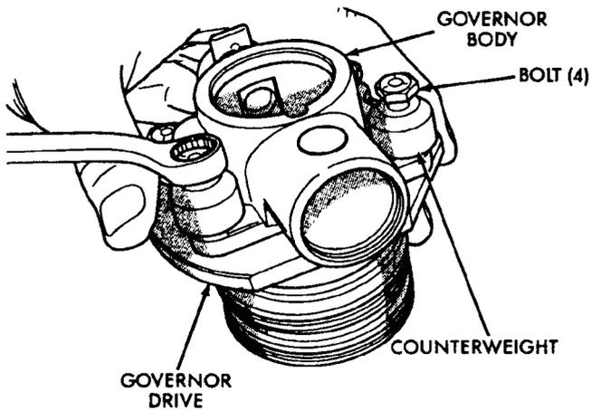
**Fig. 39 Governor Body Attaching Bolts And Spacer Removal**
