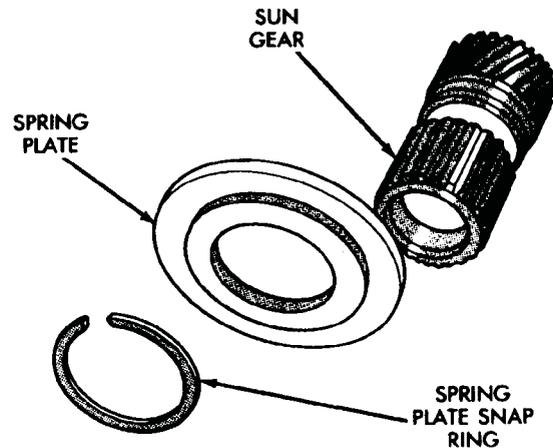
**Fig. 52 Sun Gear And Spring Plate Assembly**
