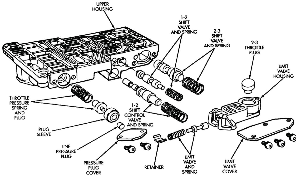
**Fig. 38 Upper Housing Shift Valves And Pressure Plugs**
