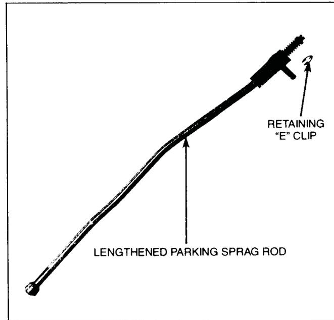
**PARKING SPRAG ROD:** The park mechanism has been moved rearward in the overdrive housing. As a result, the parking sprag rod assembly has been lengthened. The park gear is integral with the annulus gear.
