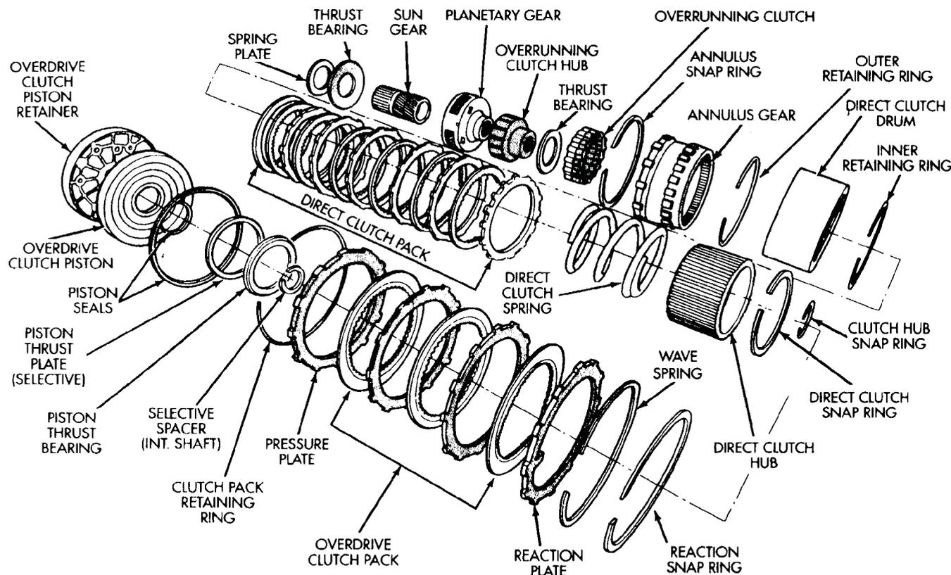
Fig. 34 Overdrive Geartrain Components (42RH Shown)
