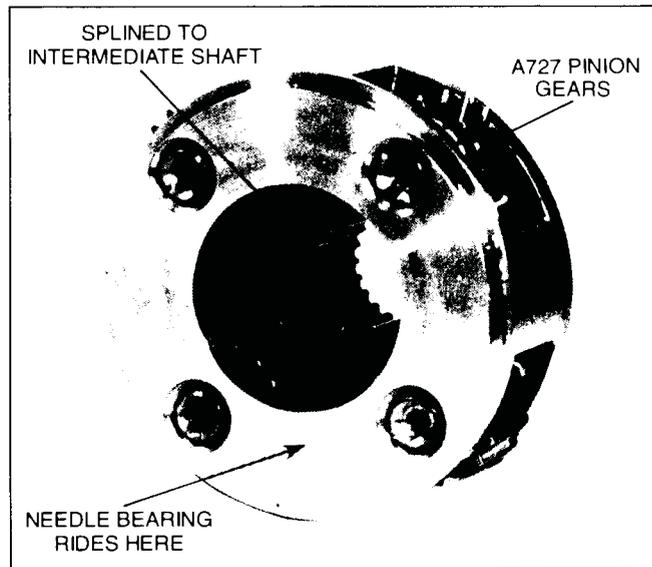
**OVERDRIVE PLANETARY PINION ASSEMBLY:** The planet carrier is splined to the intermediate shaft. The planetary gears utilize A727 pinions and produce an overdrive ratio of .69 to 1.
