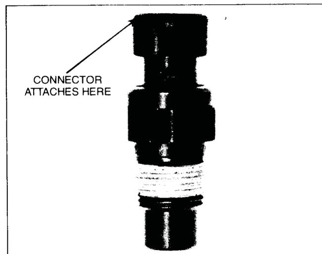
**COOLANT TEMPERATURE SENSOR:** One of the criteria for overdrive is the engine temperature must be at least 65°F. The temperature sensor is located in the intake manifold.
