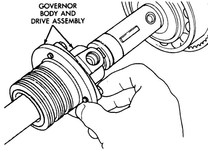
**Fig. 18 Governor Body And Drive Assembly Removal**
