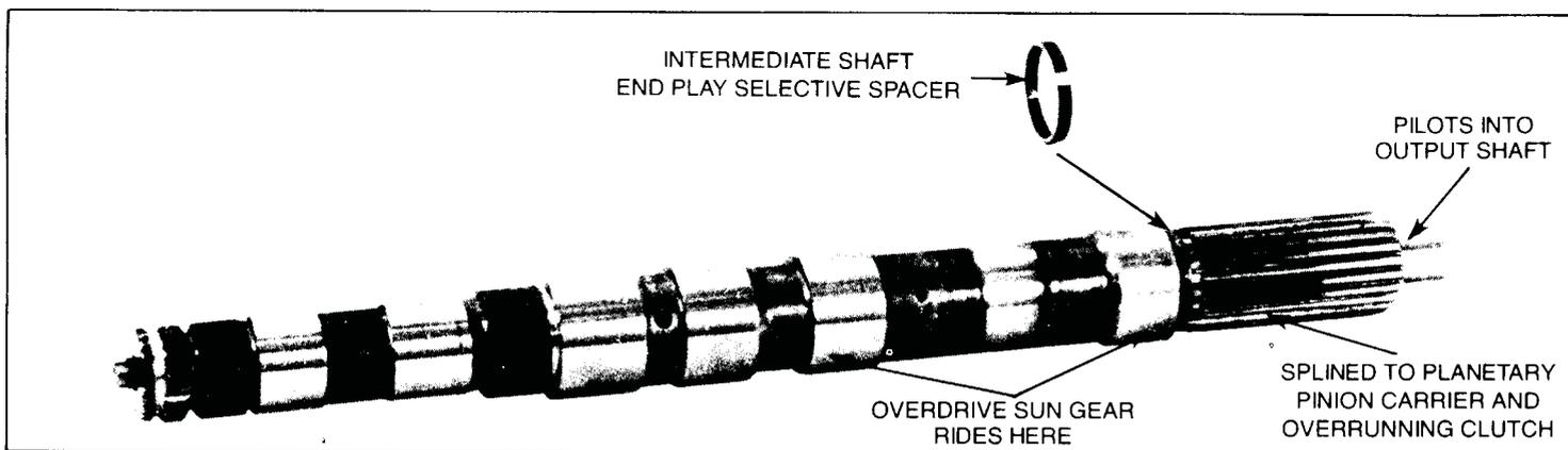
**OUTPUT SHAFT:** The output shaft is referred to as the intermediate shaft in the A-500. The back end has been modified so it splines with the overdrive planetary pinion carrier and overrunning clutch inner race. The shaft has been shortened, and no longer has the governor mounted on it. Other modifications include removal of the speedometer pinion gear drive, and the mounting surface for the output shaft bearing. The rear part of the intermediate shaft pilots in the output shaft.
