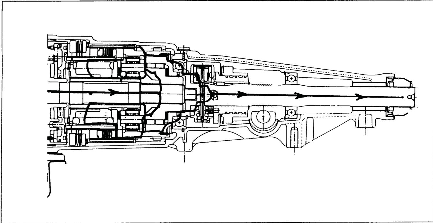
**REVERSE** - The power flow for reverse will be similar to the direct power flow explained earlier. The only difference will be that there is no power flow through the overrunning clutch. The overrunning clutch will freewheel in the reverse direction.
