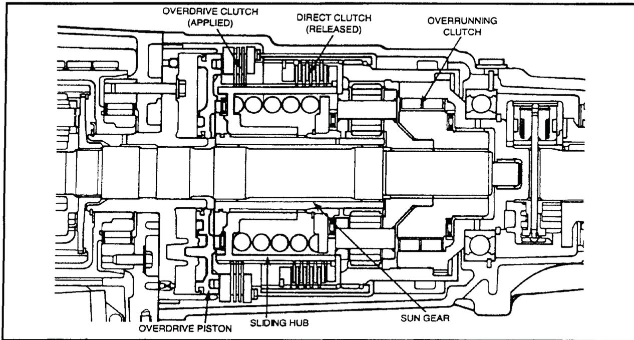
THE OVERDRIVE CLUTCH is normally not applied. The clutch is splined to the overdrive housing and the sliding hub. The purpose of the clutch is to hold the sun gear, through the sliding hub, when it's applied. That's all it does! The only time this clutch is engaged is in overdrive.
