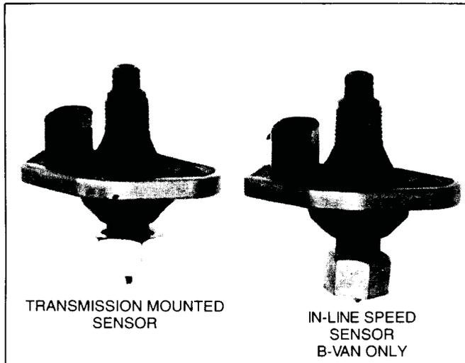
**VEHICLE SPEED/DISTANCE SENSOR:** The vehicle must be traveling a minimum speed of approximately 25 m.p.h. before the transmission can upshift to overdrive. The vehicle speed sensor is located on the speedometer pinion housing, or in the case of our B-van's, in-line.
