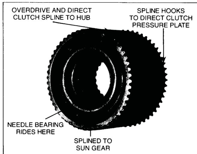
**SLIDING HUB:** This sliding hub is splined to the front of the sun gear, and held in place with a snap ring. The hub is used to apply the direct clutch using spring tension, and it will release the clutch using hydraulic force from the overdrive piston. The direct clutch and, the overdrive clutch are both splined to the hub. When the direct clutch is applied it will turn the hub for direct drive. When the overdrive clutch is applied it will hold the hub from turning, causing overdrive.
