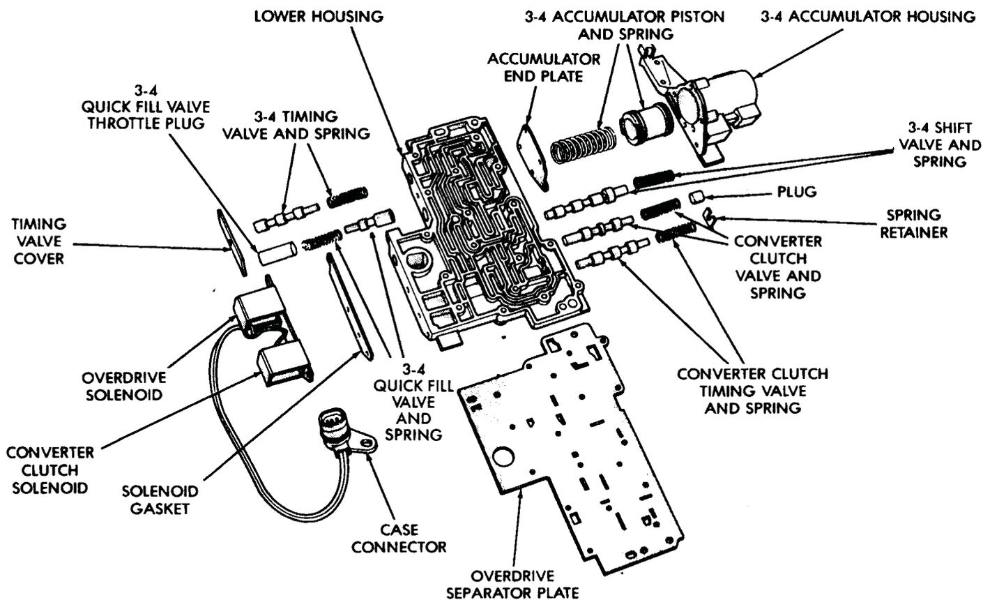
**Fig. 36 Lower Housing Shift Valves And Springs**
