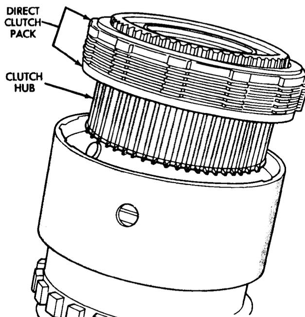
**Fig. 59 Installing Assembled Direct Clutch Pack And Hub**
