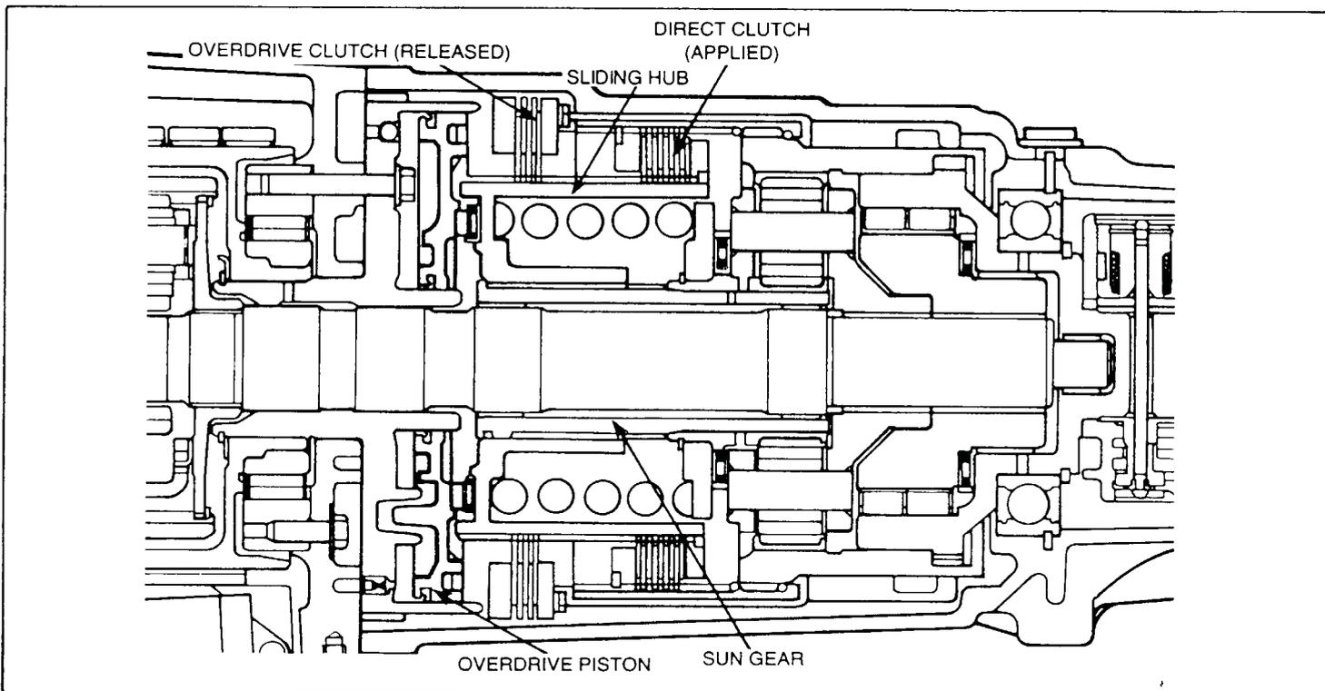
**THE DIRECT CLUTCH** is normally applied, even when the vehicle is turned off! This is done using a large spring. Looking at the illustration you will notice the spring is seated on a thrust plate. The spring is constantly pushing forward on the sliding hub, which is splined to the overdrive sun gear. Keep in mind that the hub and sun gear are splined together, so if the hub is turned the sun gear must turn, and, if the hub is held stationary the sun gear is stationary.
