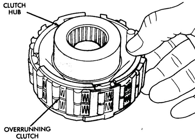
**Fig. 48 Assembling Overrunning Clutch And Hub**
