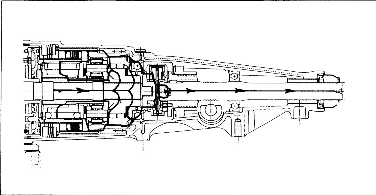
**DIRECT (FORWARD)**- The transmission must be in a forward gear, and the overdrive unit will have the overdrive clutch disengaged. Both the direct clutch and the overdrive overrunning clutch will be engaged.
