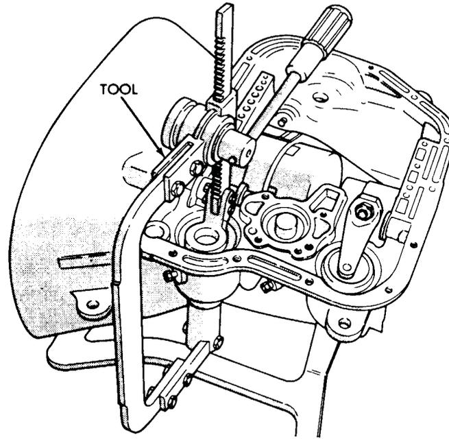
**Fig. 7—Compress Kickdown Servo Spring**
