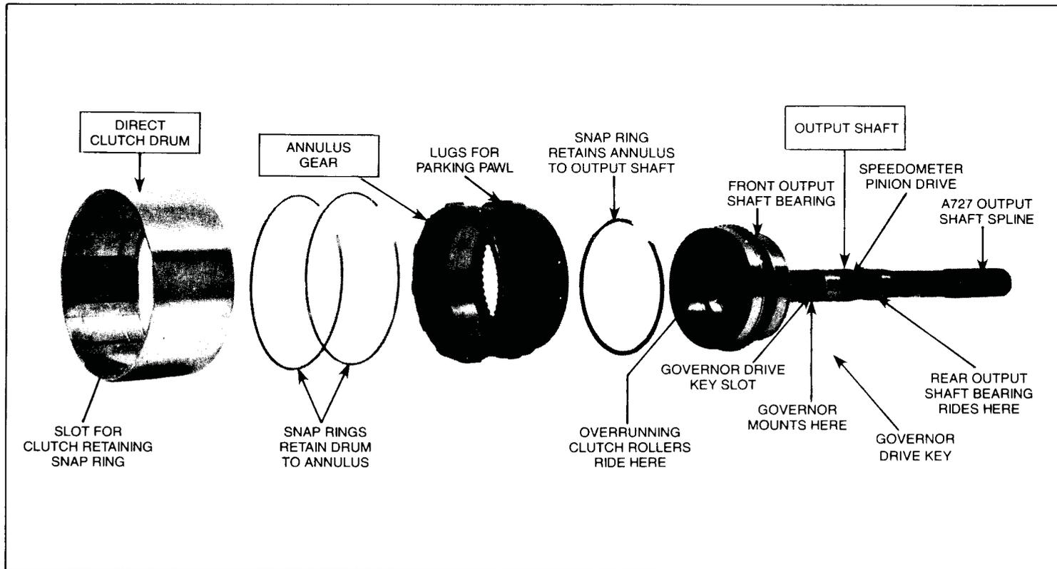
**DIRECT CLUTCH DRUM:** The direct clutch drum is splined to the annulus gear and held in place using two snap rings. The direct clutch plates are splined to the inside of the drum, and held in place with a snap ring.
