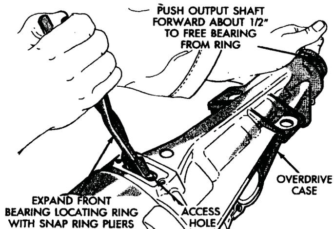
**Fig. 10 Releasing Shaft Front Bearing From Locating Ring**
