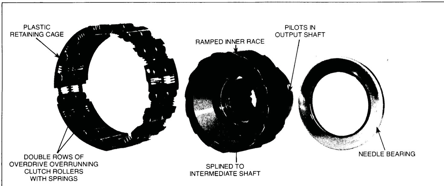
**OVERDRIVE OVERRUNNING CLUTCH INNER RACE AND ROLLER ASSEMBLY:** The inner race of the overrunning clutch is splined to the intermediate shaft. Around the outside of the inner race rides a double set of rollers for a one-way mechanical clutch. The overrunning clutch is used to allow a smooth shift from direct to overdrive.
