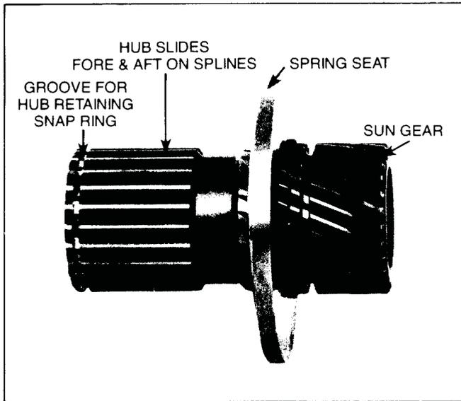
**OVERDRIVE SUN GEAR:** The sun gear rides on the intermediate shaft with the rear most part of the gear meshing with the planetary gears. The forward portion of the sun gear is splined to the sliding hub. The sun gear will be turned for direct drive and held for overdrive.
