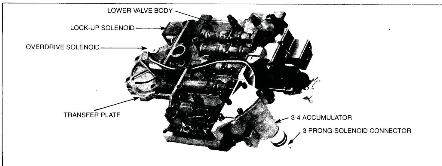
**VALVE BODY:** The valve body transfer plate has been modified so the lower valve body housing can be mounted to it. The lower valve body includes five valves and, an attaching accumulator assembly. Two, SMEC controlled, solenoids are mounted on the lower valve body. One solenoid controls the lock-up torque converter, while the
