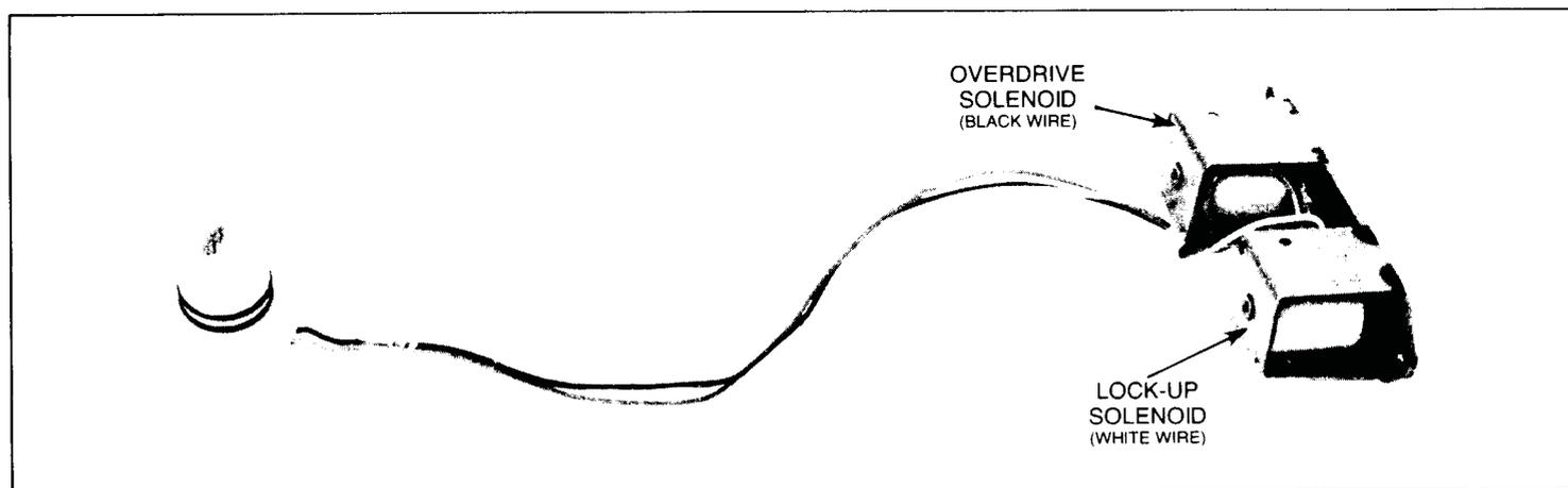
**OVERDRIVE SOLENOID:** The overdrive solenoid is coupled with the torque converter solenoid and mounted to the lower valve body. The two solenoids share a common three pin connector that is mounted so it passes through the case. The overdrive solenoid is designed to control third
