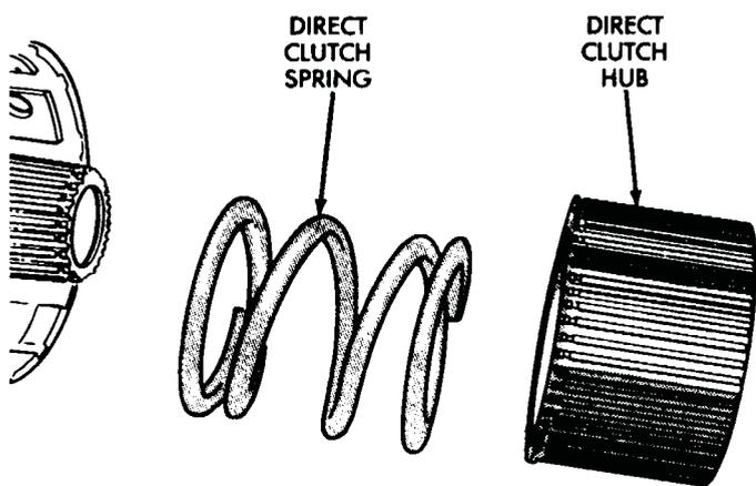
**Fig. 25 Direct Clutch Hub And Spring Removal**
