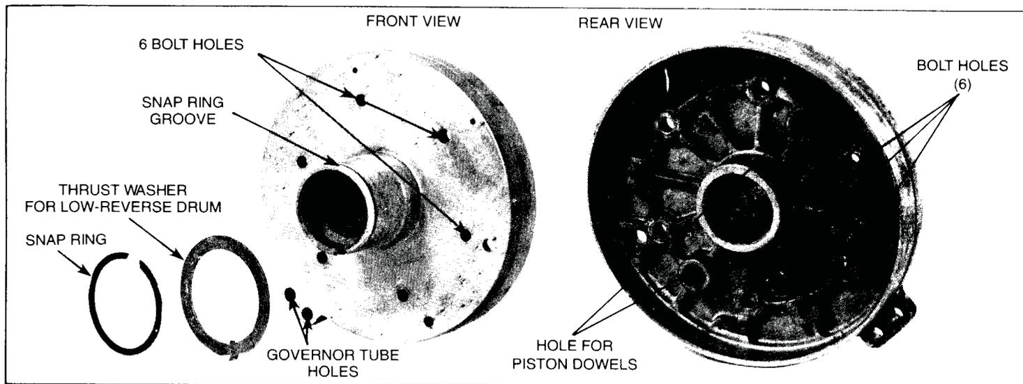
**OUTPUT SHAFT SUPPORT:** The most noticeable change of the output shaft support (**now called the OVERDRIVE PISTON RETAINER**) is the size. Where the governor assembly used to be located is now a piston bore for the overrunning clutch piston. The front end of the support has a groove that retains a snap ring that holds a thrust
