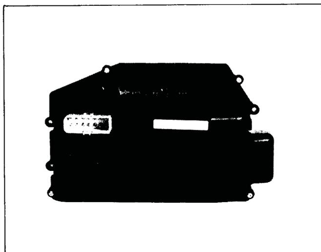
**SMEC (ENGINE CONTROLLER):** The SMEC has the added responsibility of controlling the ground circuit to activate, or deactivate, the overdrive solenoid. The SMEC uses already existing engine and vehicle sensors to determine the proper overdrive up-shift and down-shift points.
