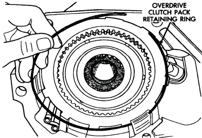
**Fig. 5 Overdrive Clutch Pack Retaining Ring Removal**
