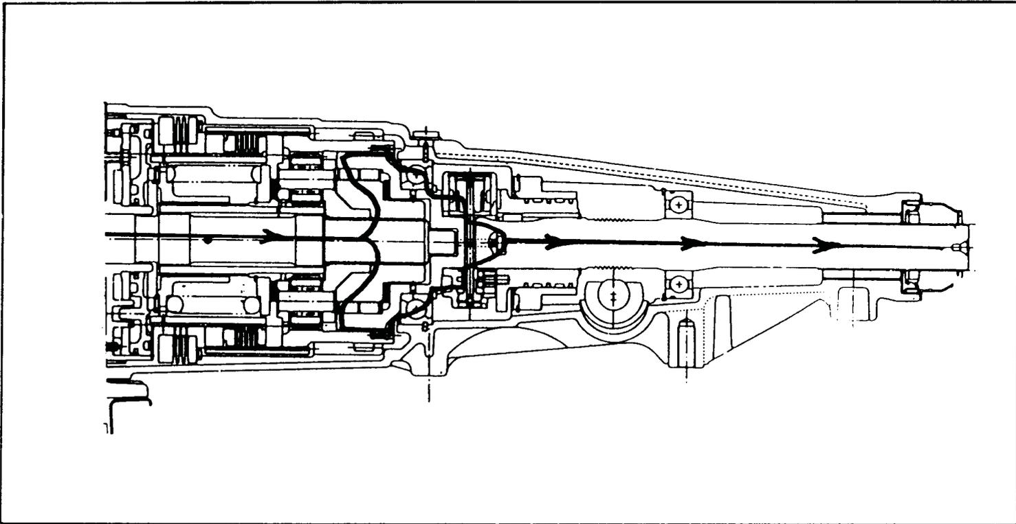
**OVERDRIVE-** The transmission must be in third gear, and the overdrive unit will have the overdrive clutch engaged. The direct clutch and the overrunning clutch will both be disengaged.
