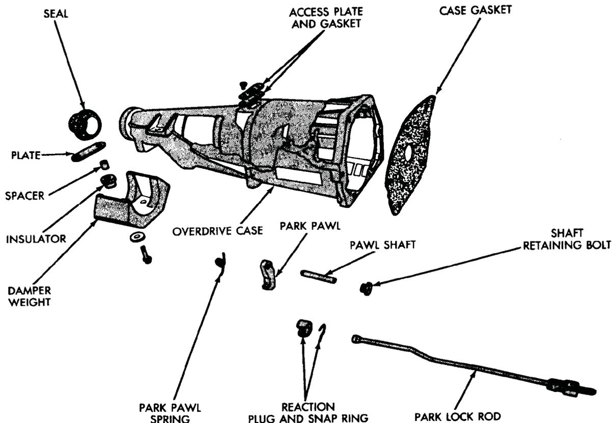
**Fig. 35 Overdrive Case And Park Lock Components**
