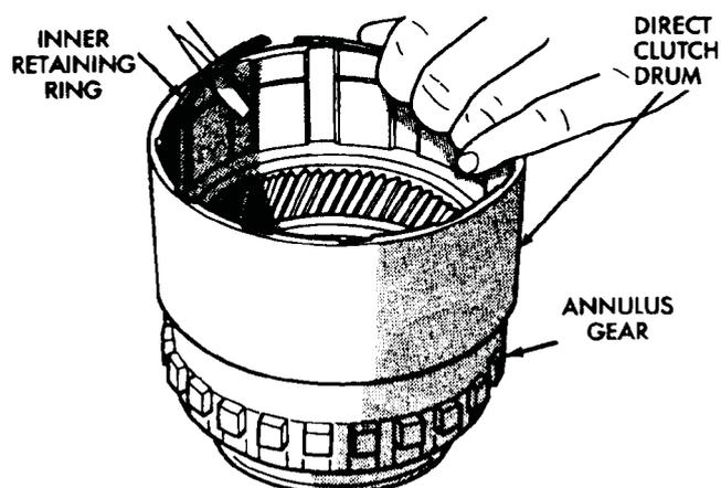
**Fig. 30 Removing Clutch Drum Inner Retaining Ring**
