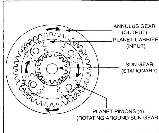
**OVERDRIVE-** This second condition shows the sun gear being held stationary. The planetary carrier is being turned by the intermediate shaft, causing the planetary pinions to walk around the stationary sun gear. The rotating planet pinions will drive the annulus gear at a faster rate of speed than the input speed. This ratio is .69 to 1, and is referred to as overdrive.
