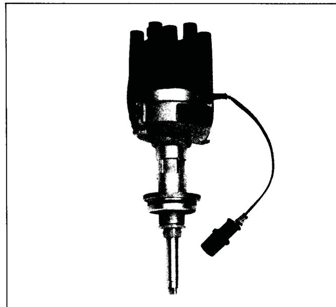
**ENGINE SPEED SIGNAL:** The engine speed signal comes from the distributor pick-up in the distributor. The engine speed signal is compared to the TPS signal to determine engagement and disengagement of the overdrive, as was mentioned earlier. This signal is also compared to the vehicle speed sensor to verify the transmission is in third gear before shifting to overdrive.
