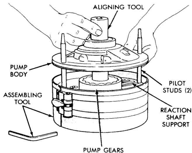
**Fig. 12—Assemble Pump and Reaction Shaft Support**
