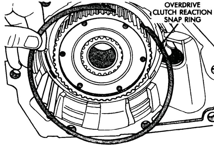
**Fig. 8 Overdrive Clutch Reaction Snap Ring Removal**
