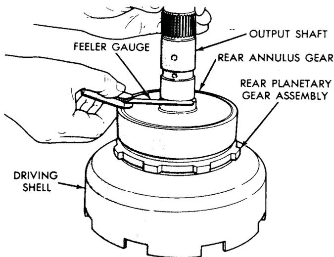
Fig. 20—Measure End Play of Planetary Gear Train
