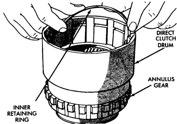
**Fig. 47 Clutch Drum Inner Retaining Ring Installation**
