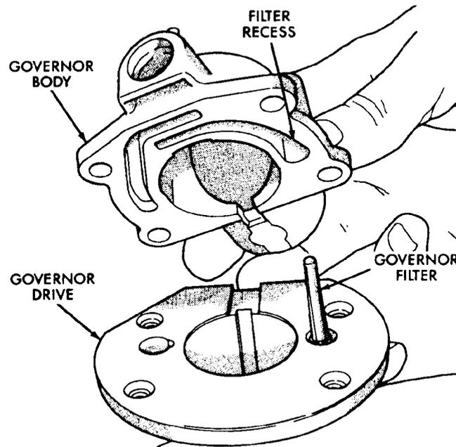
**Fig. 40 Governor Body And Filter Position (On Drive)**
