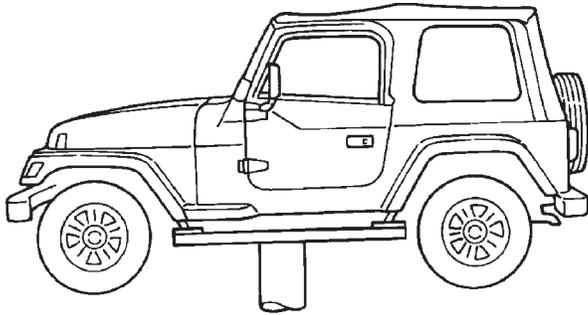
**NOTE:** Use the correct sub-frame rail or frame rail lifting locations only.
