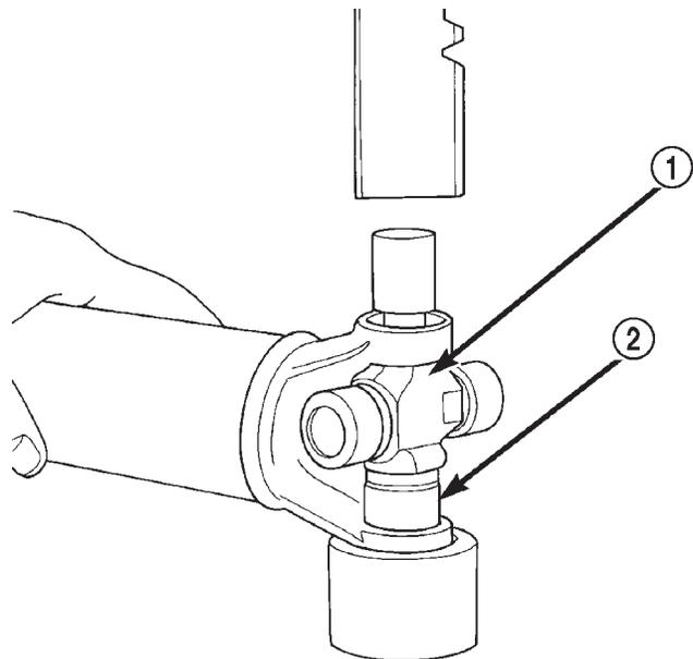
**Fig. 20 Press Out Remaining Bearing**1 - CROSS
