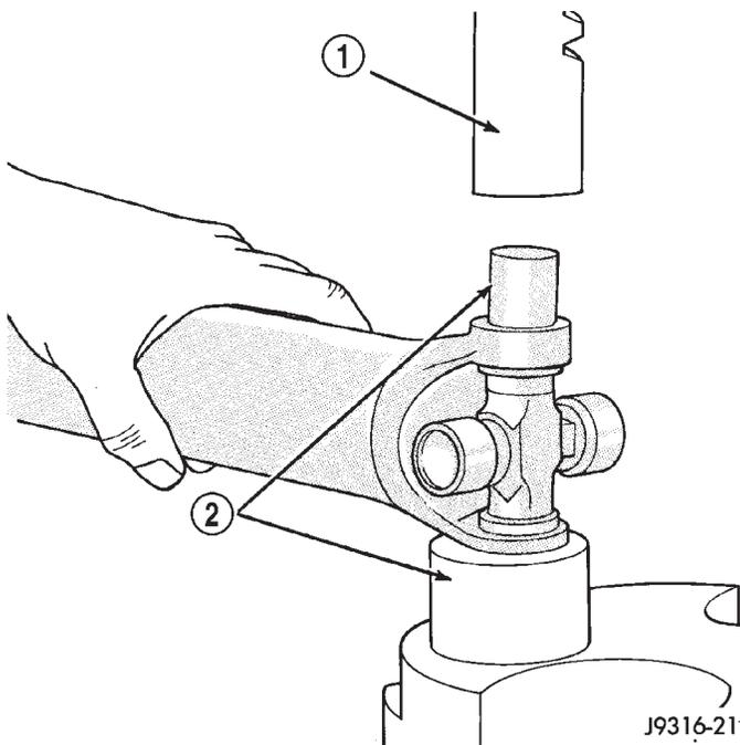
**Fig. 19 Press Out Bearing**1 - PRESS
