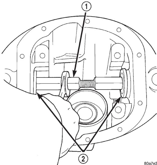
**Fig. 33 Axle Seal Installation**
