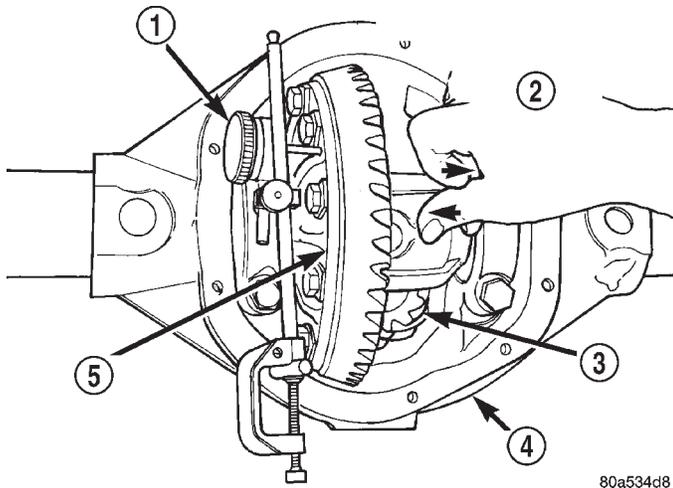
**Fig. 69 Hold Differential Case and Read Dial Indicator**
