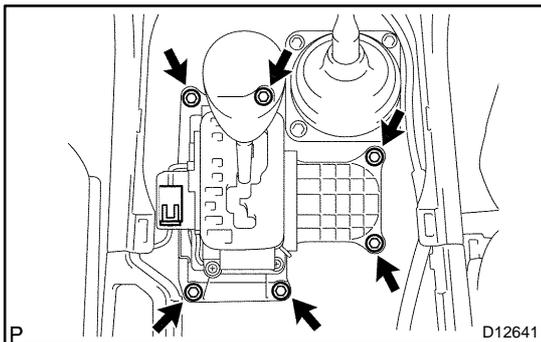
4. REMOVE FLOOR SHIFT LEVER ASSEMBLY
