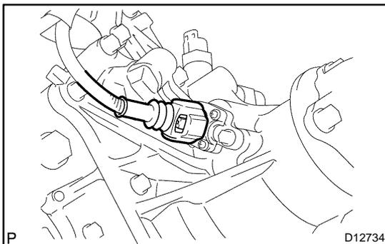
6. **CONNECT NO. 1 VEHICLE SPEED SENSOR CONNECTOR**
