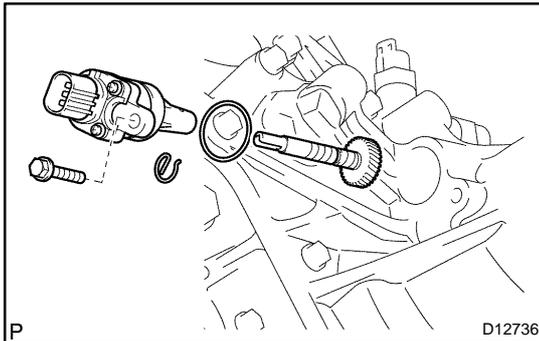
2. **REMOVE NO. 1 VEHICLE SPEED SENSOR**
