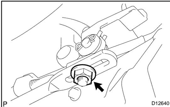
3. SEPARATE NO. 1 FLOOR SHIFT GEAR SHIFTING ROD
