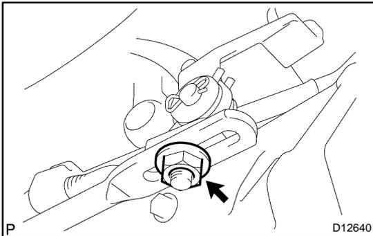
2. **INSTALL No.1 FLOOR SHIFT GEAR SHIFTING ROD**
