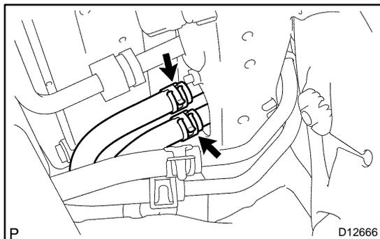
**4. REMOVE OIL COOLER PIPE BRACKET**
