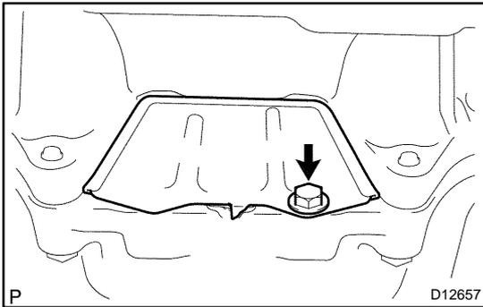
**11. REMOVE TORQUE CONVERTER CLUTCH MOUNTING BOLT**
