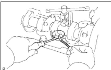
(4) Remove the adjusting shim with a screwdriver and magnetic finger.
