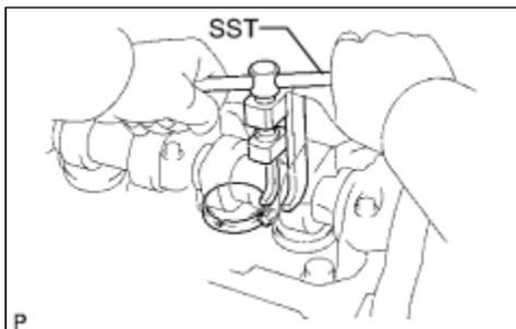
(c) Install a new adjusting shim.
