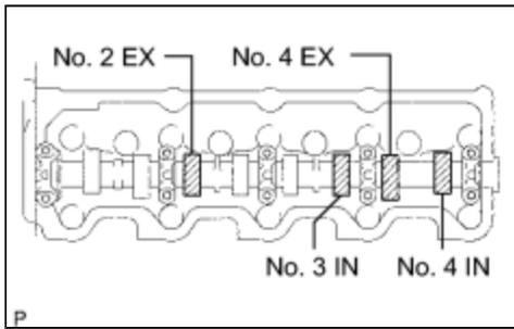
(b) Turn the crankshaft one revolution (360°) and align the mark as above. (See procedure in step 3)
