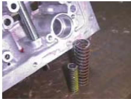
OD direct clutch Accumulator pistons
