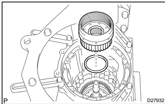
**97. INSTALL FRONT PLANETARY RING GEAR**
