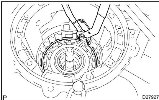
**39. REMOVE 2ND BRAKE PISTON HOLE SNAP RING**
