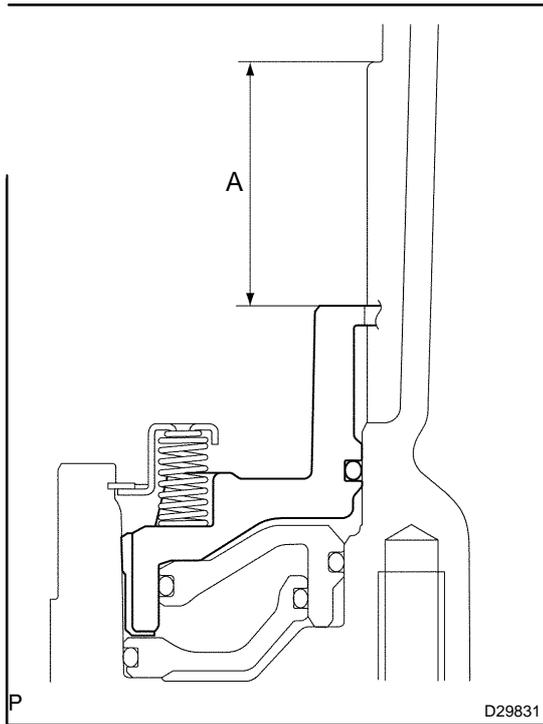
(b) Using vernier calipers, measure the level difference (length A) between the upper surface of the 1st & reverse brake piston and the hitting surface of the brake flange No.4 at the both end across a diameter, and calculate the average.
