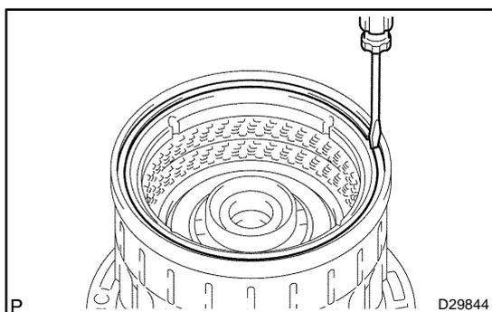
**35. REMOVE REVERSE CLUTCH REACTION SLEEVE**
