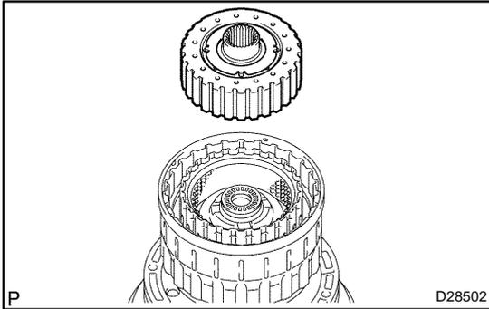
**9. REMOVE MULTIPLE DISC CLUTCH CLUTCH HUB**
