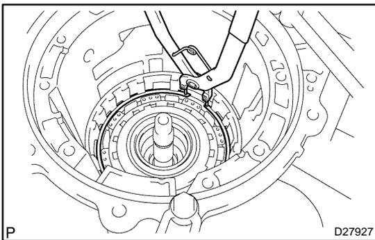
**103. INSTALL 2ND BRAKE PISTON HOLE SNAP RING**
