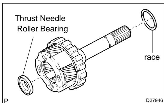
(b) Install the thrust needle roller bearing.
