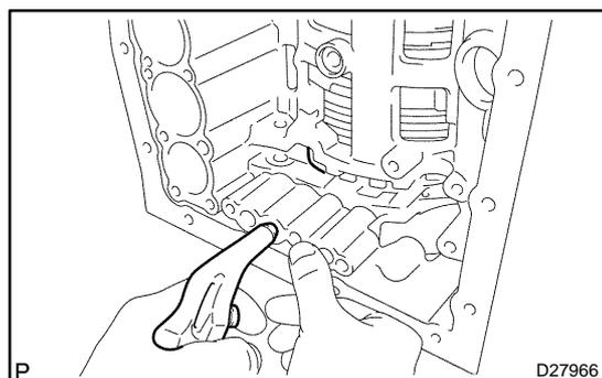
**83. INSPECT PACK CLEARANCE OF FIRST & REVERSE BRAKE**
