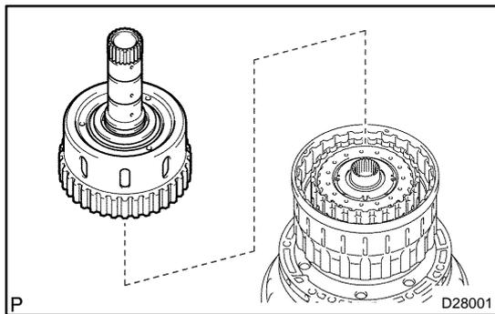
**7. REMOVE FORWARD CLUTCH HUB SUB-ASSY**
