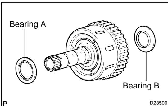
**43. INSTALL FORWARD CLUTCH HUB SUB-ASSY**
