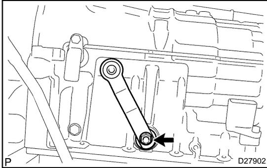
1. **REMOVE TRANSMISSION CONTROL SHAFT LEVER LH (A750F EXCEPT 4RUNNER, GX470)**
