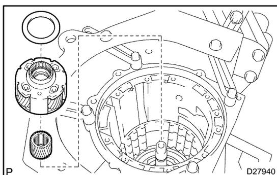
**59. REMOVE CTR PLANETARY GEAR ASSY**
