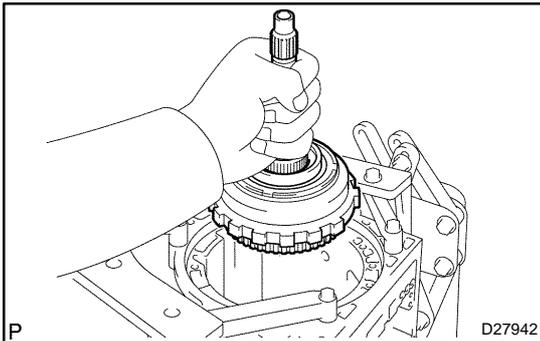
(b) Remove the intermediate shaft with the 1 way clutch assy No.3 from the case.
