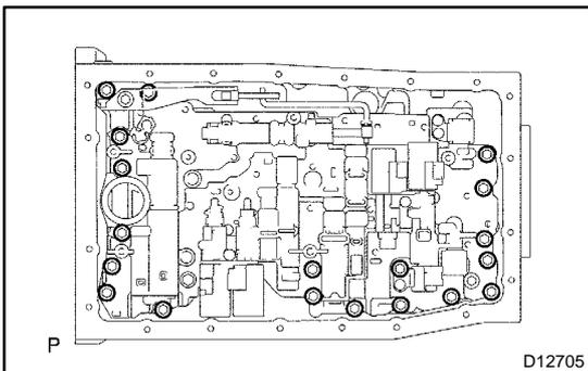
**19. REMOVE TRANSMISSION VALVE BODY ASSY**
