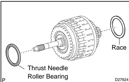
**107. INSTALL CLUTCH DRUM & INPUT SHAFT ASSY**
