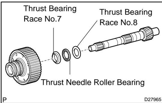
**86. INSTALL RR PLANETARY RING GEAR FLANGE SUB-ASSY**
