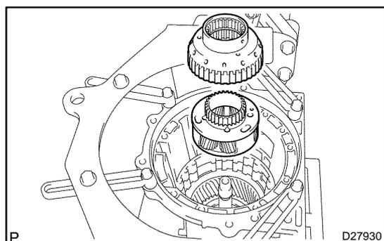
**44. REMOVE FRONT PLANETARY GEAR ASSY**
