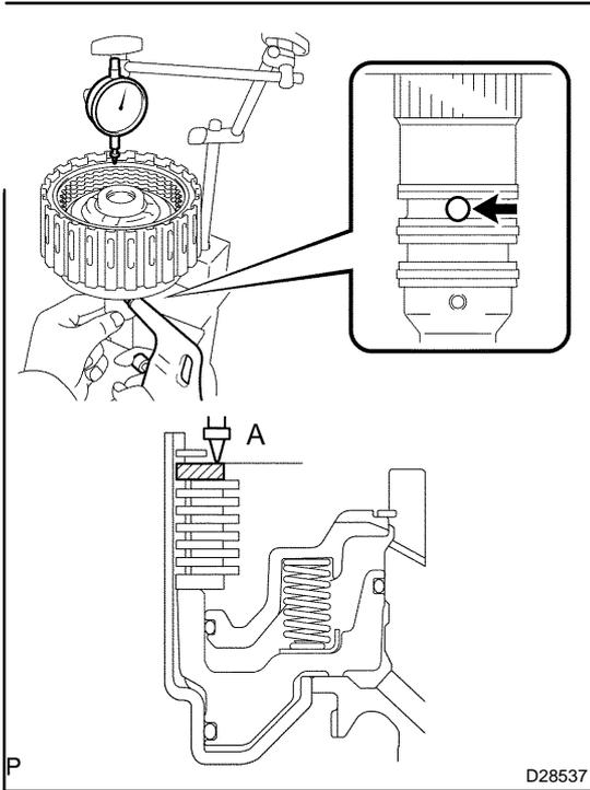
**40. INSPECT PACK CLEARANCE OF FORWARD CLUTCH**
