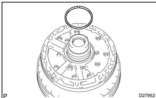
**18. INSTALL CLUTCH DRUM OIL SEAL RING**
