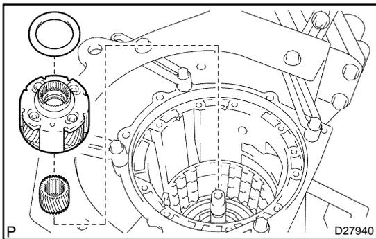
**89. INSTALL CTR PLANETARY GEAR ASSY**
