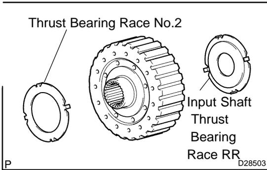
**42. INSTALL MULTIPLE DISC CLUTCH CLUTCH HUB**
