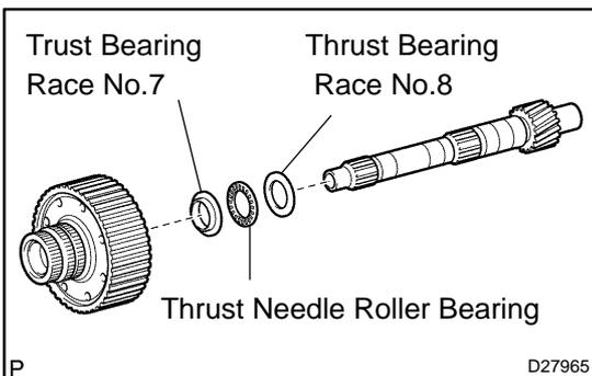
**64. REMOVE RR PLANETARY RING GEAR FLANGE SUB-ASSY**
