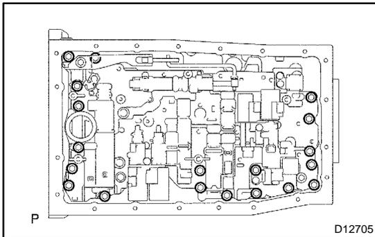
**1. REMOVE TRANSMISSION VALVE BODY ASSY**
