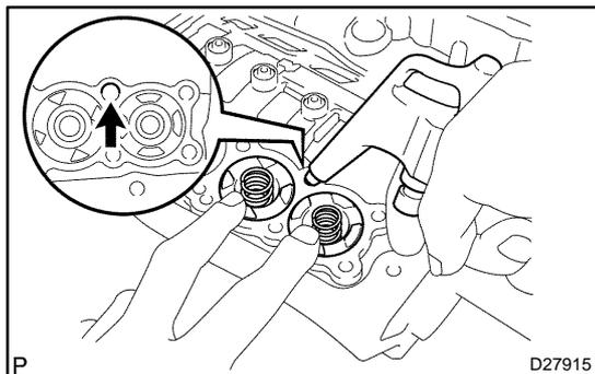
**24. REMOVE B-3 ACCUMULATOR PISTON**
