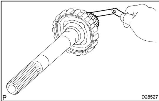
**71. INSPECT REAR PLANETARY GEAR ASSY**
