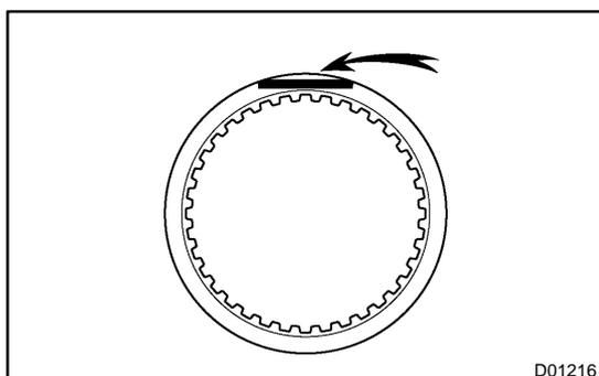
**13. INSPECT FORWARD MULTIPLE DISC CLUTCH CLUTCH DISC**
