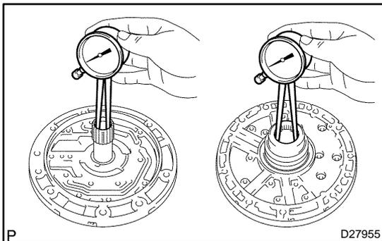
**7. INSPECT STATOR SHAFT ASSY**
