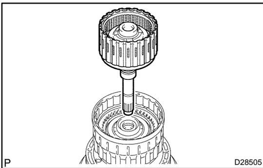
**41. INSTALL INPUT SHAFT ASSY**
