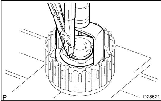
**14. REMOVE CLUTCH BALANCER NO.1**
