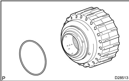
**27. INSTALL REVERSE CLUTCH PISTON SUB-ASSY**
