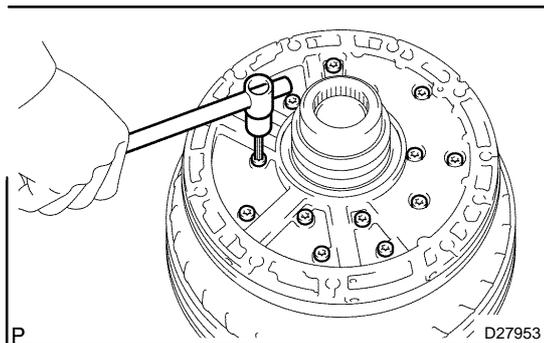
**17. INSTALL STATOR SHAFT ASSY**
