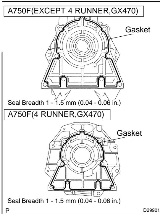
**131. INSTALL TRANSMISSION CASE ADAPTER ADAPTER SUB-ASSY (4WD DRIVE TYPE)**
