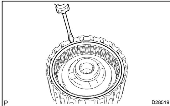
**12. REMOVE FORWARD MULTIPLE DISC CLUTCH CLUTCH DISC**
