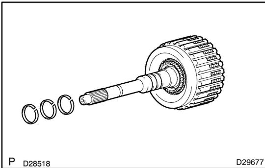
**39. INSTALL INPUT SHAFT OIL SEAL RING**
