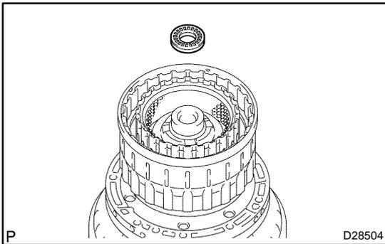
**10. REMOVE INPUT SHAFT ASSY**
