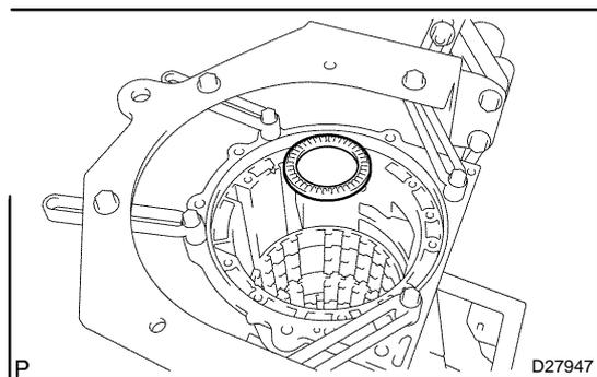
**82. INSTALL REAR PLANETARY GEAR ASSY**
