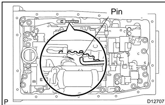
**122. INSTALL TRANSMISSION VALVE BODY ASSY**
