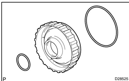
**36. INSTALL FORWARD CLUTCH PISTON**
