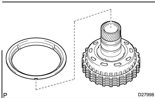
**45. INSTALL REVERSE CLUTCH REACTION SLEEVE**
