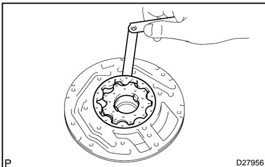
**8. INSPECT CLEARANCE OF OIL PUMP ASSEMBLY**
