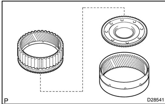
**96. INSTALL CTR PLANETARY RING GEAR**
