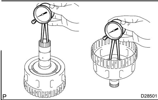
**8. INSPECT FORWARD CLUTCH HUB SUB-ASSY**
