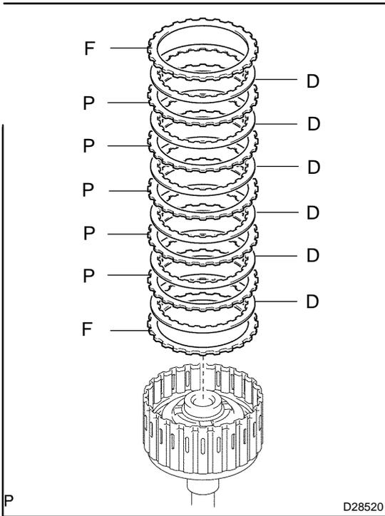
**38. INSTALL FORWARD MULTIPLE DISC CLUTCH CLUTCH DISC**
