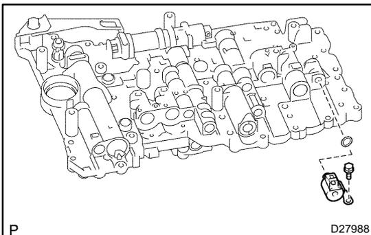
**8. REMOVE SHIFT SOLENOID VALVE S2**
