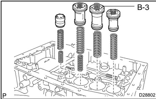
**117. INSTALL B-3 ACCUMULATOR PISTON**
