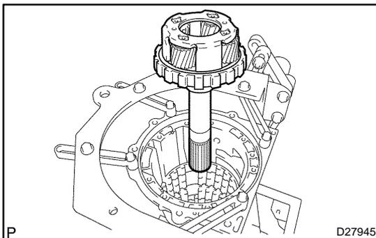
**70. REMOVE REAR PLANETARY GEAR ASSY**
