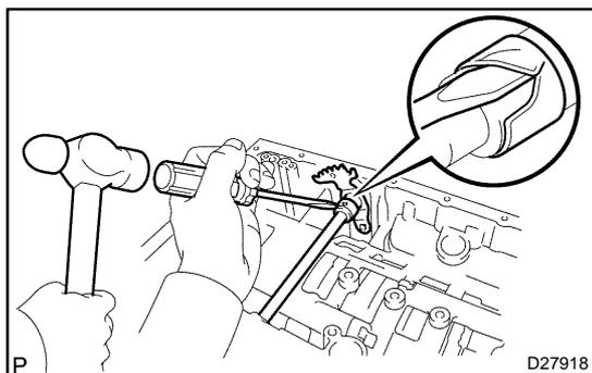
**30. REMOVE MANUAL VALVE LEVER SUB-ASSY**
