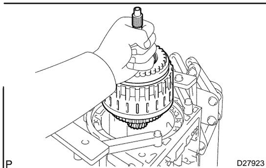
**33. REMOVE CLUTCH DRUM & INPUT SHAFT ASSY**
