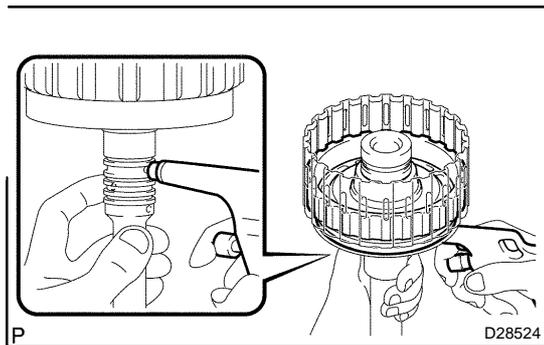
**16. REMOVE FORWARD CLUTCH PISTON**
