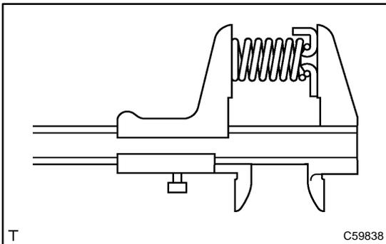
**15. INSPECT FORWARD CLUTCH RETURN SPRING SUB-ASSY**
