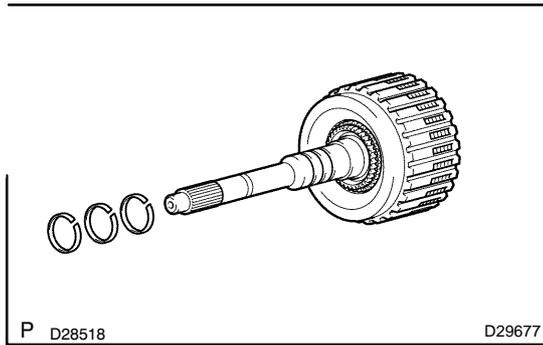
**11. REMOVE INPUT SHAFT OIL SEAL RING**
