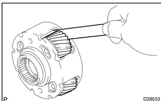
**60. INSPECT CTR PLANETARY GEAR ASSY**
