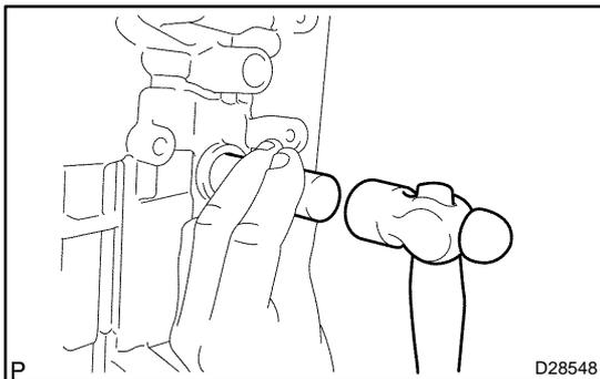
**109. INSTALL MANUAL VALVE LEVER SHAFT OIL SEAL**
