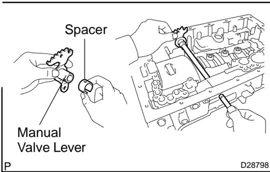
**111. INSTALL MANUAL VALVE LEVER SUB-ASSY**
