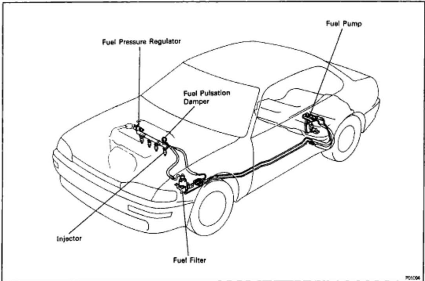
Fuel pumped up by the fuel pump, flows through the fuel filter and is distributed to each injector at a set pressure maintained by the pressure regulator.
