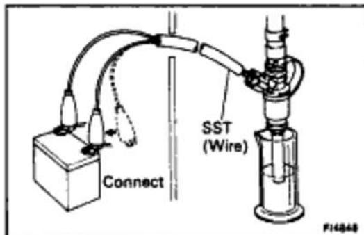
(l) Connect SST (wire) to the injector and battery for 15 seconds, and measure the injection volume with a graduated cylinder. Test each injector 2 or 3 times.
