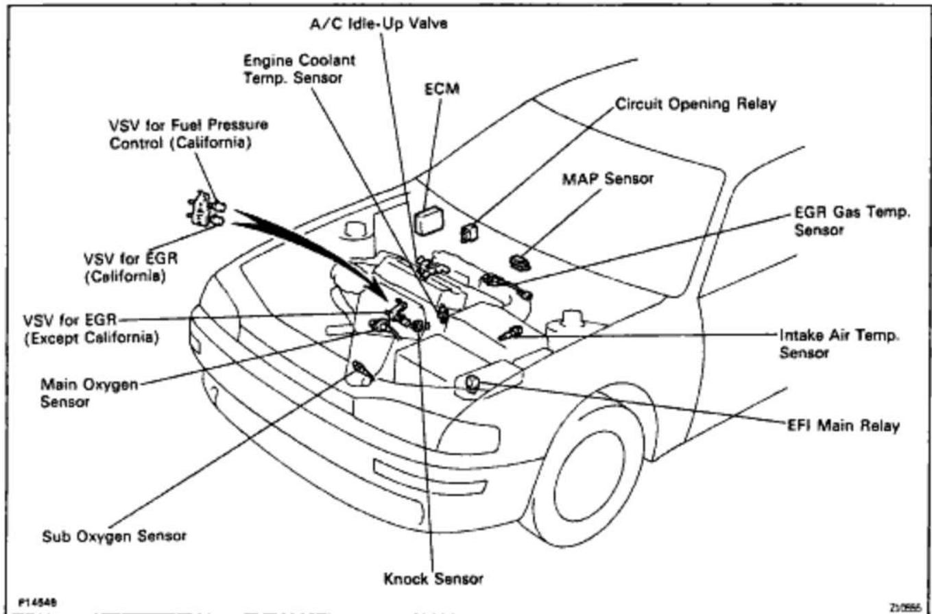
The control system consists of sensors which detect various engine conditions, and a ECM which determines the injection volume (timing) based on the signals from the sensors.
