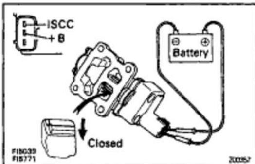
**IAC VALVE INSPECTION****INSPECT IAC VALVE OPERATION**
