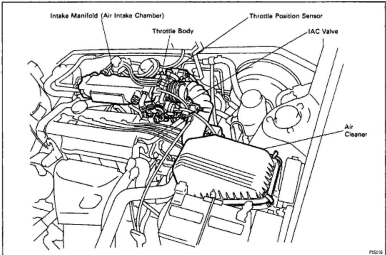
Air is filtered through the air cleaner and the amount flowing to the air intake chamber is determined according to the throttle valve opening in the throttle body and the engine speed. Intake air controlled by the throttle valve opening is distributed from the air intake chamber to the manifold of each cylinder and is drawn into the combustion chamber.
