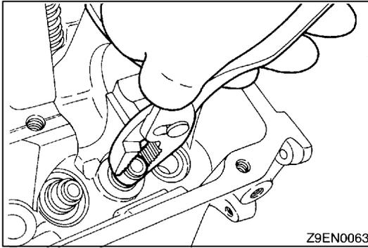
**◀C▶ VALVE STEM SEAL REMOVAL****◀D▶ VALVE HANDLING PRECAUTIONS**
