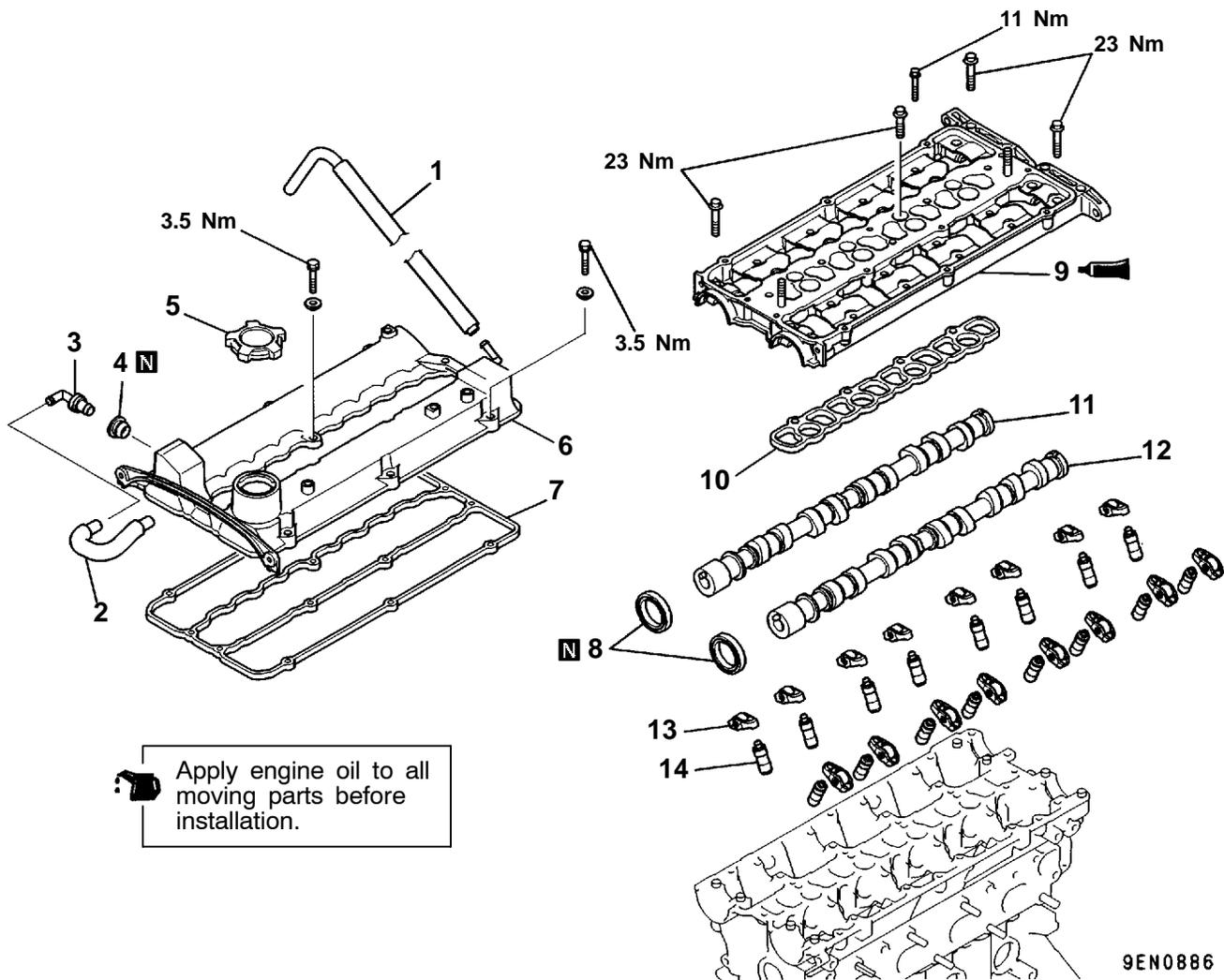
Apply engine oil to all moving parts before installation.
