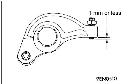
**INSTALLATION SERVICE POINTS****▶A◀ ADJUSTING SCREW INSTALLATION**
