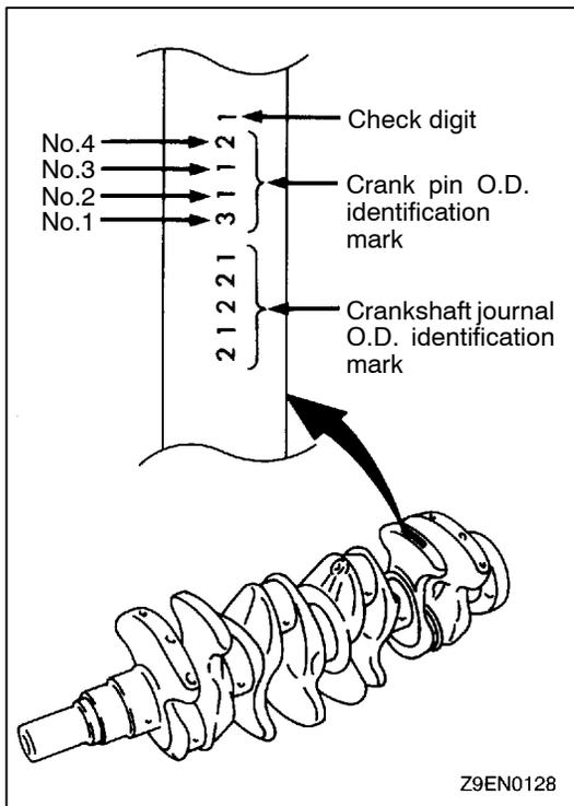
**►E◄ CONNECTING ROD BEARING INSTALLATION**
