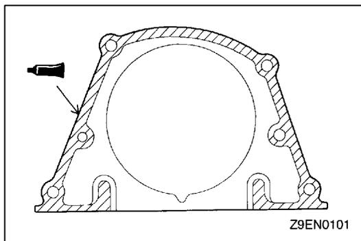
▶E◀ **SEALANT APPLICATION TO OIL SEAL CASE**
