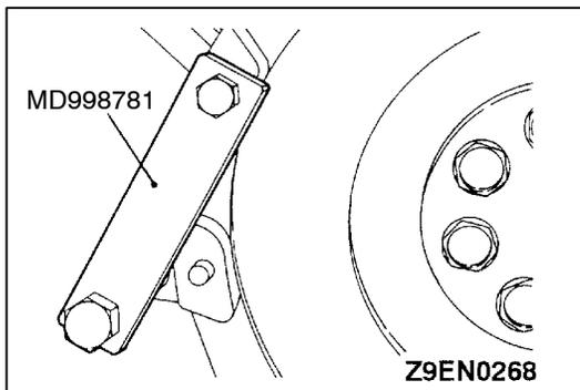
**▶B◀ CRANKSHAFT BOLT INSTALLATION**
