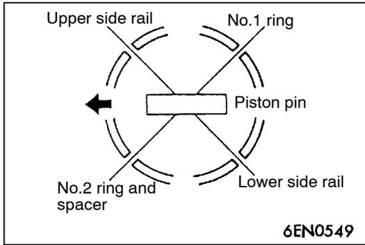
**►D◄ PISTON AND CONNECTING ROD INSTALLATION**
