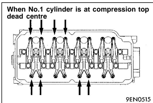
(2) The valve clearances at the places indicated by arrows in the illustration can be adjusted.
