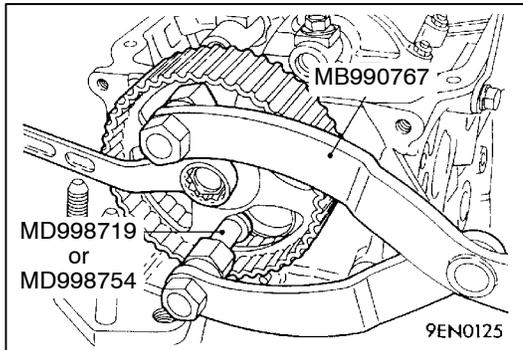
**◀B▶ CAMSHAFT SPROCKET BOLT REMOVAL****<With rocker cover removed> (Except SOHC)**
