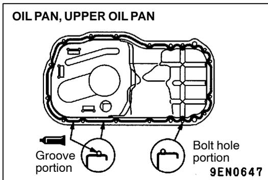
▶D◀ **OIL PAN/UPPER OIL PAN/LOWER OIL PAN INSTALLATION**
