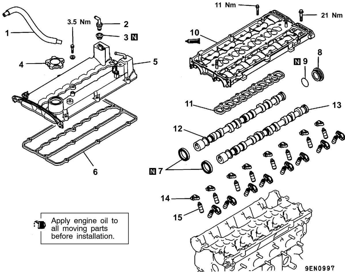
Apply engine oil to all moving parts before installation.
