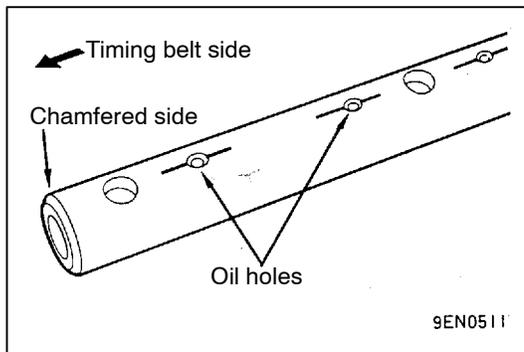
**▶B◀ ROCKER ARM SHAFT INSTALLATION**
