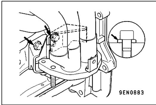
**INSTALLATION SERVICE POINTS****▶A◀ EXHAUST MANIFOLD BRACKET INSTALLATION**
