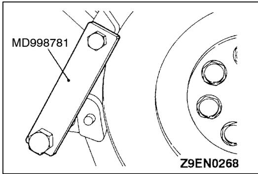
**REMOVAL SERVICE POINT****◀A▶ CRANKSHAFT BOLT REMOVAL**
