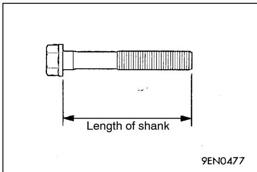
▶◀ BEARING CAP/BEARING CAP BOLT INSTALLATION
