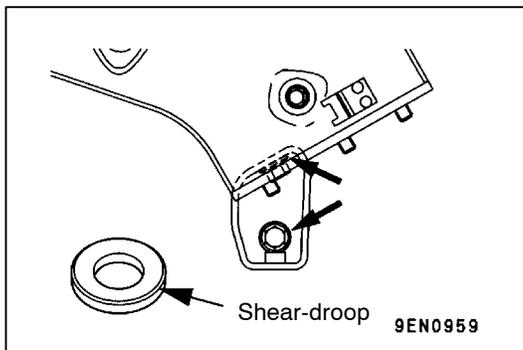
**▶B◀ EXHAUST MANIFOLD BRACKET INSTALLATION**
