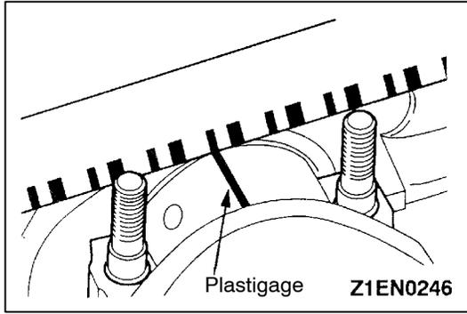
**CRANKSHAFT PIN OIL CLEARANCE (PLASTIGAGE METHOD)**
