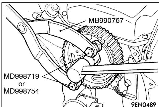
**INSTALLATION SERVICE POINTS****▶A◀ CAMSHAFT SPROCKET BOLT INSTALLATION**
