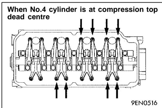
(6) Adjust the valve clearances indicated by arrows in the illustration by the same procedure as in steps (3) and (4) above.
