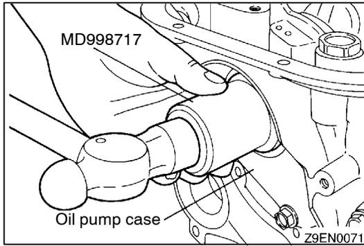
▶C◀ **CRANKSHAFT FRONT OIL SEAL INSTALLATION**
