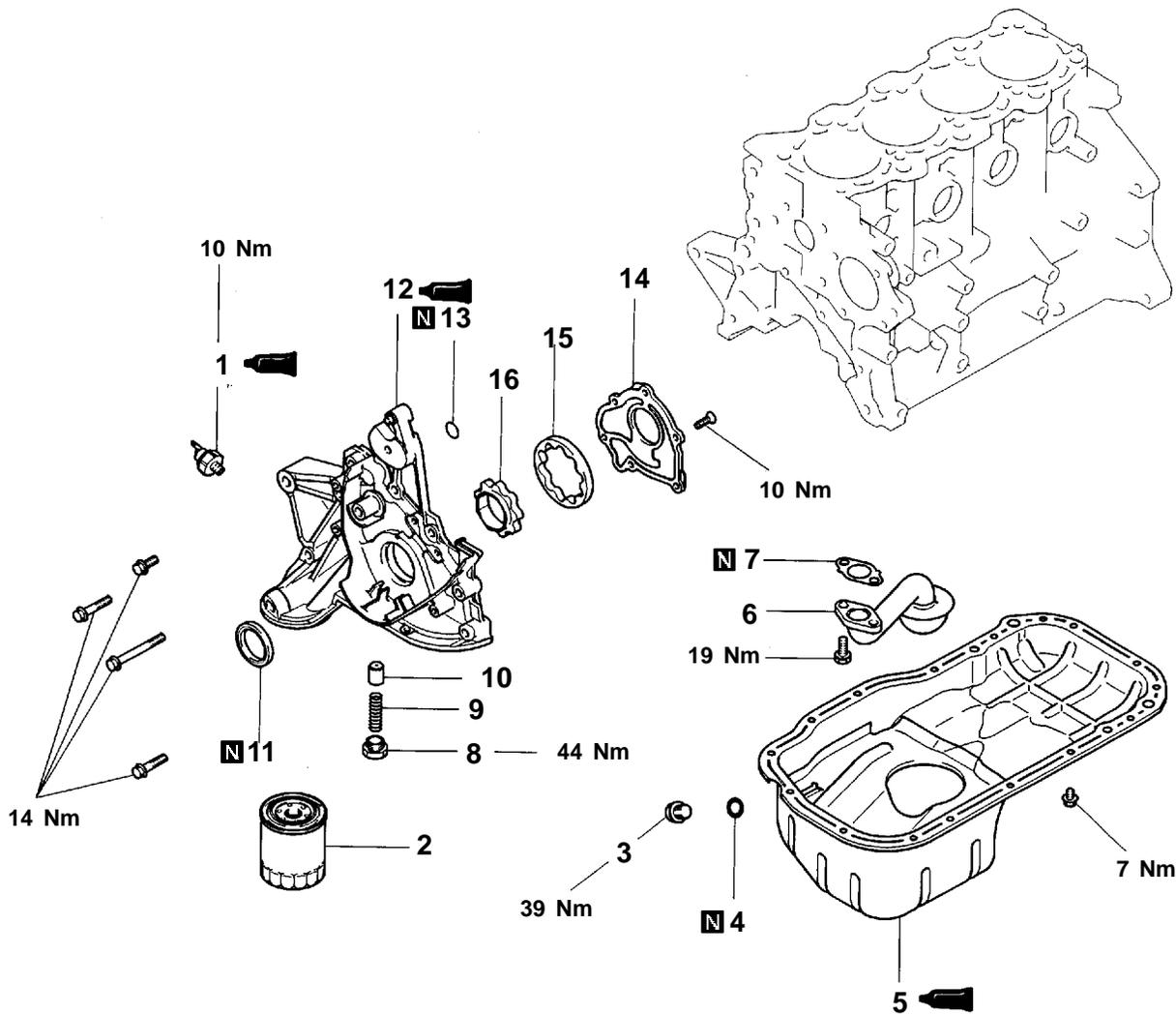
Apply engine oil to all moving parts before installation.
