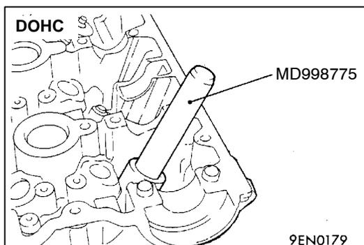
**INSTALLATION SERVICE POINTS****▶A◀ VALVE STEM SEAL INSTALLATION**
