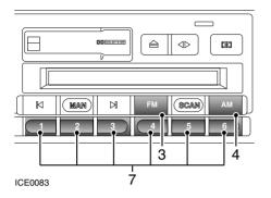
The six pre-set buttons (7) can be used to manually store up to twelve FM stations (six each on FM1 and FM2) and twelve AM stations (six each on AM1 and AM2). The pre-sets are programmed as follows:
