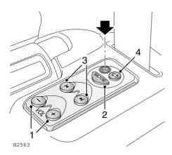
The rear passenger headphone controls only operate with the main audio unit switched on. Plug the headphones into the socket (arrowed in illustration) to activate the controls - bass response from the vehicle speakers reduces and the headphone symbol, along with a symbol indicating the current headphone unit mode, appears in the display.
