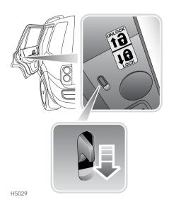
On 5-door models, move the lever on the rear doors down (arrowed in illustration) to engage.
