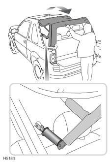
5. Unfold the softback rearwards. Check that the elbow stays have remained unlocked, as indicated above.
