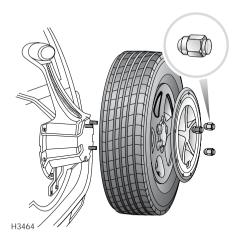
Vehicles fitted with a steel spare wheel are supplied with a cover, which fits against the wheel, and is secured by the wheel nuts.
