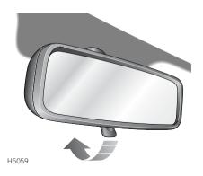
The interior mirror can be dipped to reduce glare from following vehicles. In the event of excessive glare, move the lever at the base of the mirror forward to 'dip' the mirror. Normal visibility is restored by pulling the lever back to its original position.
