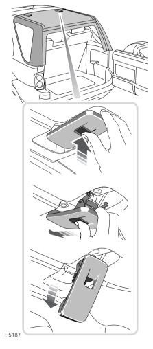
**1.** Press the button on the catch, then push the catch forwards and allow to drop.
