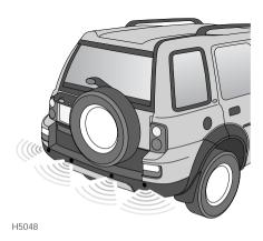
The parking system assists the driver when manoeuvring the vehicle into a parking space, or anywhere that there are obstacles that need to be avoided, warning the driver accordingly.
