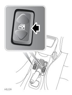
The switches on centre console operate the windows as follows:
