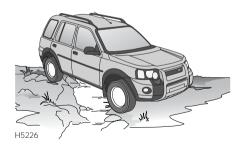
Cross ditches at an angle so that three wheels always maintain contact with the ground. If a ditch is approached head on, both front wheels will drop into the ditch together, possibly resulting in the body and front bumper being trapped on opposite sides of the ditch.
