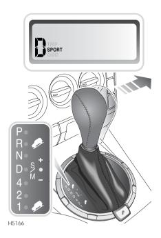
In Sport mode, full automatic progression through the gear ratios is retained. By selecting Sport mode however, the power transmitted to the road wheels is increased, resulting in improved acceleration. Engine revs are higher in all driving conditions, making the vehicle more responsive to driver commands.
