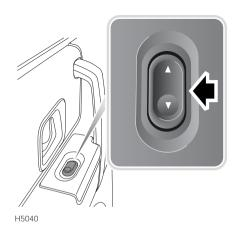
Rear seat passengers can control the raising and lowering of their window by using the switch on either of the rear doors. (Provided that the rear windows have not been isolated by the driver).
