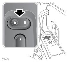
This is a personal security feature which allows the driver (or passenger) to lock (or unlock) all the doors from inside the vehicle (while driving or with the vehicle stationary). Press the padlock symbol part of the switch to lock (the alarm will not be armed), and the unlocked padlock symbol to unlock.
