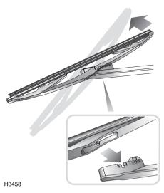
Lift the wiper arm away from the rear window, as far as the spare wheel carrier will allow. Pivot the blade assembly away from the arm (as arrowed), levering against resistance, until the two retaining lugs detach from their slots at the end of the arm. Carefully replace the arm to its stowed position.
