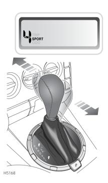
There are five predetermined gear ratios, all of which can be selected sequentially by a single forward or rearward movement of the gear selector lever, as follows:
