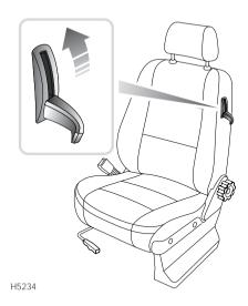
To enable rear seat passengers to enter or exit the vehicle, lift the backrest release lever upwards to fold the front seat backrest forwards.
