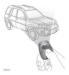
While it is not necessary to point the handset at the vehicle, the handset must be within range of the vehicle when a button is pressed. Note that the operating range may vary depending upon handset battery condition and may sometimes be limited by physical and geographical factors beyond your control. From a security point of view, it may not be wise to unlock unless you are in close proximity to the vehicle.
