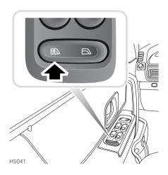
Press switch '5' as indicated to isolate the rear window switches. Press the other end of the switch to restore independent control.
