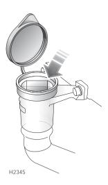
The windshield washer reservoir supplies both front and rear screen washer jets.
