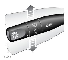
Move the lever DOWN to indicate a LEFT turn, and UP to indicate a RIGHT turn.
