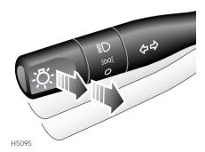
Pull the lever fully towards the steering wheel to change headlight beams (BLUE warning light glows when the headlights are on high beam).
