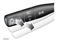
Pull the lever fully towards the steering wheel to change headlight beams.
