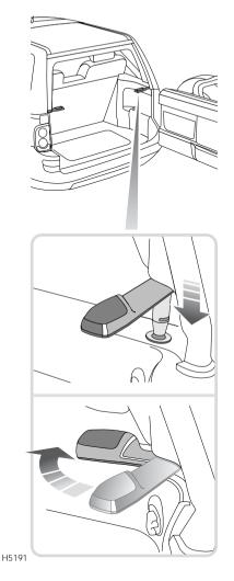
2. Locate the rear locking pins and pivot both locking levers 90° forwards.
