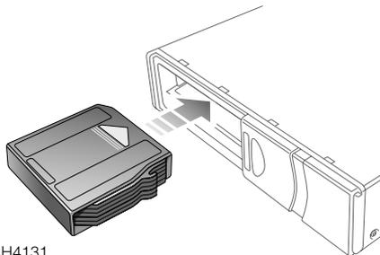
Correctly align the tray with the parallel slots on each side of the magazine and slide the tray fully into the magazine. Finally, close the sliding cover.
