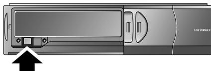
Press the button to eject the magazine.
