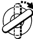
**6. FINALLY,** turn the key to the UNLOCK position once more to disarm the alarm and re-mobilise the engine. If the code has been entered successfully, the anti-theft alarm indicator light will extinguish, the doors will unlock and the engine can be started.
