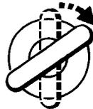
**4. Enter the THIRD digit of the code.** If the third digit is 2, turn the key to the UNLOCK position twice, ensuring that the key is FULLY returned to the centre position after each turn of the key.
