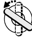
**3. Enter the SECOND digit of the code.** If the second digit is 3, turn the key to the LOCK position 3 times. Remember; the key must be FULLY returned to the centre position after each turn of the key.
