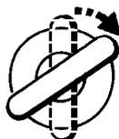
**6. FINALLY**, turn the key to the UNLOCK position once more to disarm the alarm and re-mobilise the engine. If the code has been entered successfully, the anti-theft
