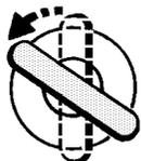
**1. Using the key**, turn the driver's door lock (anti-clockwise) to the LOCK position 4 times and return the key to the centre position
