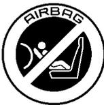
The above symbol affixed to the fascia panel of your vehicle, warns against the use of a REAR FACING child seat in the front passenger seat. This type of child seat could cause serious injury to your child in the event of an airbag deployment.
