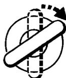
**4. Enter the THIRD digit of the code.** If the third digit is 2, turn the key to the UNLOCK position twice, ensuring that the key is FULLY returned to the centre position after each
