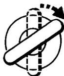
**2. Enter the FIRST digit of the code.** If the first digit is 4, turn the key (clockwise) to the UNLOCK position 4 times. Ensure the key is FULLY returned to the centre position
