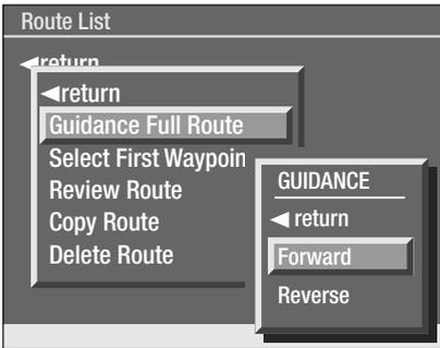
If you want to reverse the direction of the route you are following, highlight and select 'Guidance Full Route', then highlight and select 'Reverse'. The navigation computer returns to the route guidance screen while calculating the new route and new audio instructions are given.
