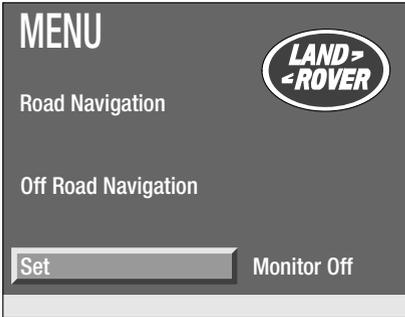
Press the 'MENU' control to view the display main menu, then use the rotary select control to highlight and select 'Set'.
