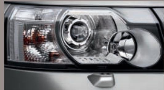
**HEADLAMPS** Three types of headlamp are available: Projector Halogen headlamps with impact-resistant polycarbonate lenses. Xenon projector lamps providing crisp blue-white light letting you see further. Adaptive Xenon projector lamps that automatically swivel with the direction of travel to improve the view of the road ahead.
