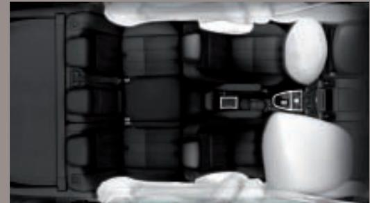
**SAFETY** Ultra-high-strength steel is used to construct an immensely strong monocoque body and inner safety cell protected by front and rear energy absorbent crumple zones. Seven airbags are fitted as standard on all vehicles. When tested in 2007 Freelander 2 was the first vehicle in its class to be awarded a five star rating for Adult Occupant Protection in the rigorous Euro NCAP tests.
