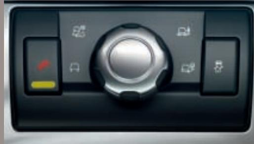
**TERRAIN RESPONSE®** Land Rover's patented Terrain Response® system\* adds to Freelander 2's breadth of capability. Any of the four programmes – general driving, grass/gravel/snow, mud and ruts, or sand – can be easily selected by simply turning the rotary control. In addition all vehicles with Terrain Response® are also fitted with Hill Descent Control\* and Land Rover's Gradient Release Control systems\*.
