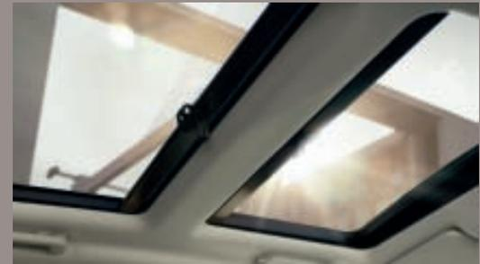
**PANORAMIC SUNROOF** The optional panoramic sunroof – with a fixed rear section and electric tilting/sliding front section – adds to the feeling of lightness and airiness within the cabin. The glass is specially formulated to filter the sun's infrared rays, providing light without unpleasant heat. Both sections also include a convenient blind.
