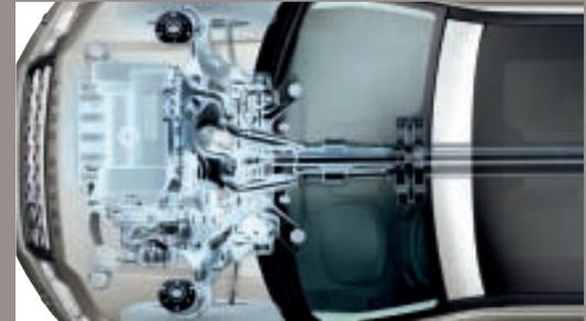
**PERFORMANCE WITH REFINEMENT.** The 2.2 litre turbodiesel engines, now available in power outputs of 150PS and 190PS, come with common-rail diesel technology which aids economy and refinement and a Variable Nozzle turbocharger helping to deliver exceptional torque.
