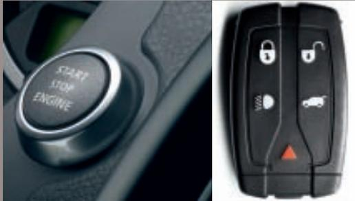
**REMOTE CONTROL AND START/STOP BUTTON** The remote control includes the following functions: locking and unlocking of the doors and tailgate, a 30 second courtesy headlamp delay and activation of panic alarm. In order to start the car the remote has to be docked into the fascia and the correct procedure followed using the Start/Stop button.
