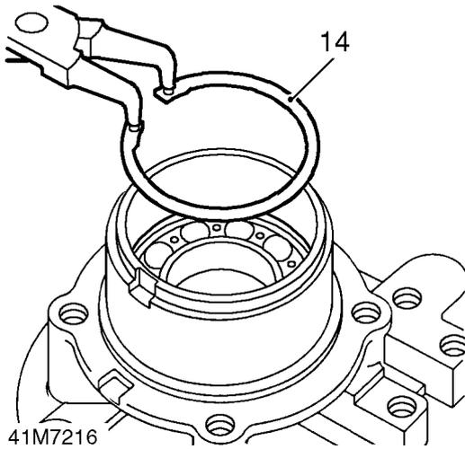
14. Using suitable circlip pliers, remove and discard circlip retaining output shaft bearing.
