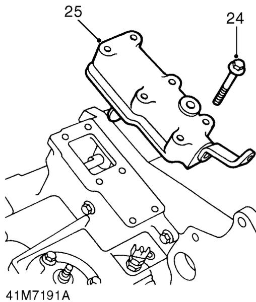
24. Remove 6 bolts securing high/low cross shaft housing.
