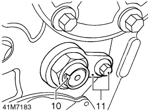
10. Release staking from intermediate shaft nut, remove and discard nut.
