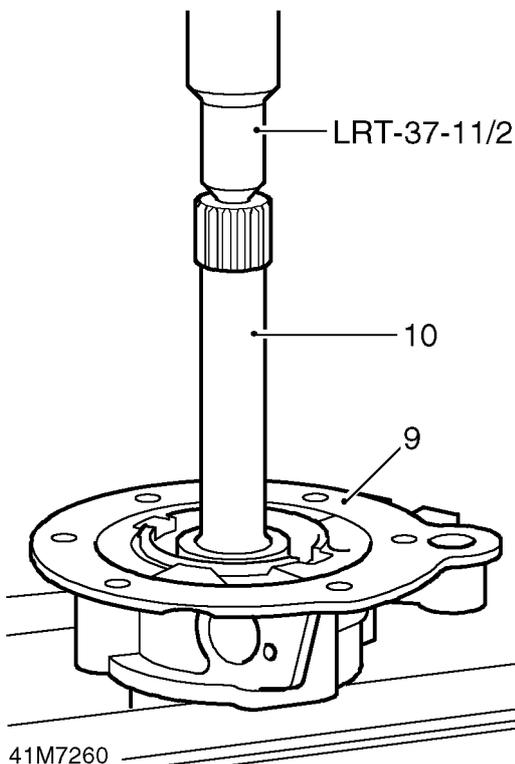
9. Position rear output housing on bed of hand press.
