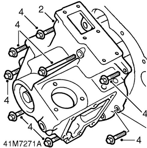
11. Position front output housing as shown.
