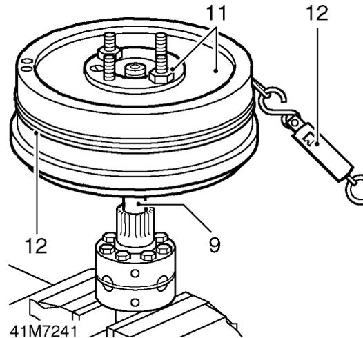
9. Insert front output shaft into front half carrier, check that gears rotate freely.
