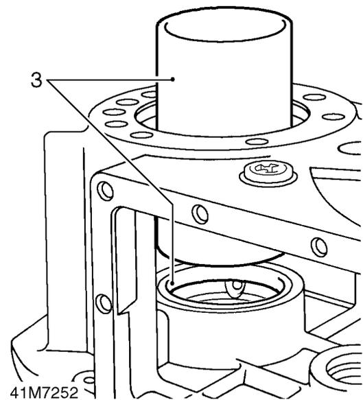
3. Using a suitable mandrel, fit a new mainshaft input gear bearing track.
