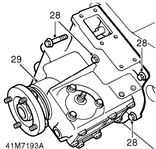
28. Noting fitted position of longest bolt, remove 8 bolts securing front output housing to main casing.
