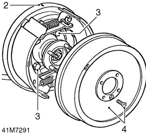
2. Position brake backplate on rear output housing ensuring that alignment marks are together.
