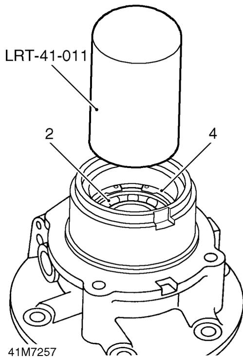
2. Fit new output shaft bearing using tool **LRT-41-011**.
