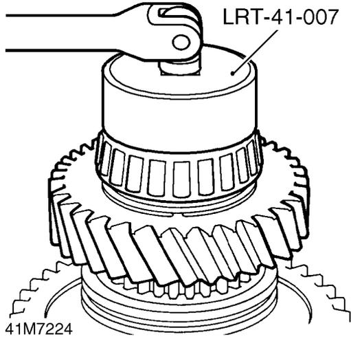
3. Remove nut using tool **LRT-41-007**; discard nut.
