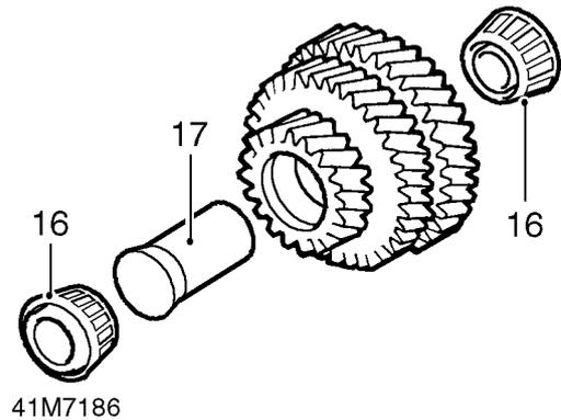
16. Remove and discard 2 taper roller bearings from intermediate gears.
