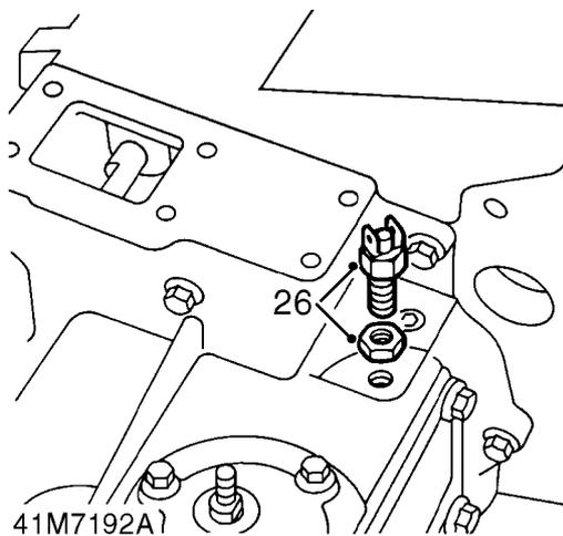
26. Slacken locknut and remove differential lock warning lamp switch from front output housing.
