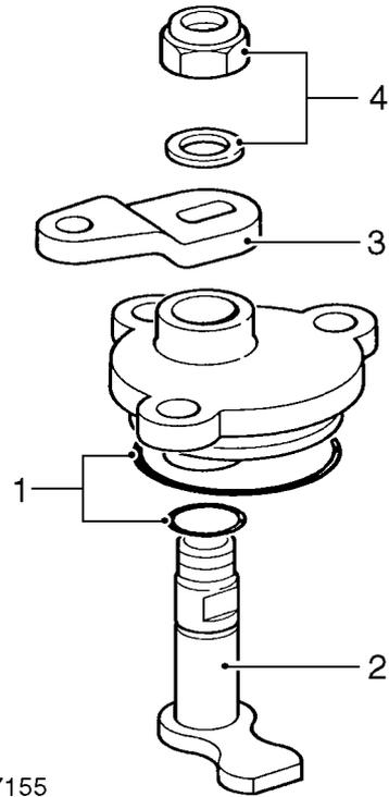
1. Lubricate new 'O' rings with recommended oil, fit to selector finger shaft and housing.
