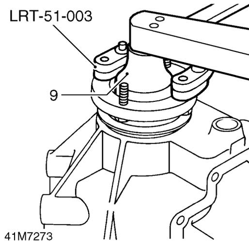
8. Position propeller shaft flange holding tool **LRT-51-003** to output flange.
