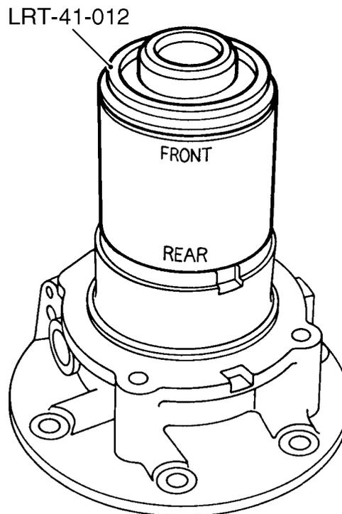
6. Fit oil seal using tool **LRT-41-012**.
