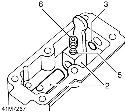
2. Insert cross shaft into housing, position high/low selector finger on shaft.
