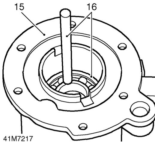
15. Support rear output housing on suitable blocks of wood.
