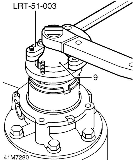
8. Position propeller shaft flange holding tool **LRT-51-003** to output flange.
