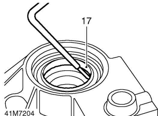
17. Taking care not to damage front output housing, remove and discard output shaft oil seal.
