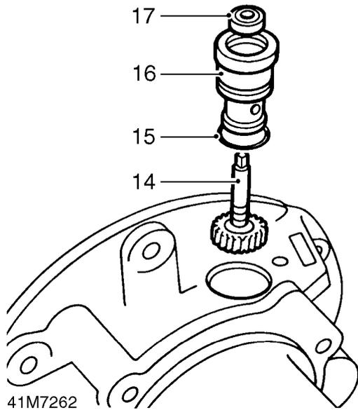
14. Fit speedometer driven gear into rear output housing ensuring that gear teeth are engaged with drive gear.
