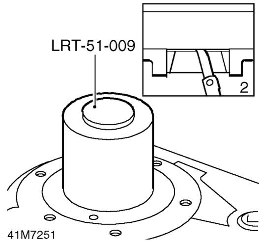
1. Fit a new differential rear bearing track using tool **LRT-51-009**.
