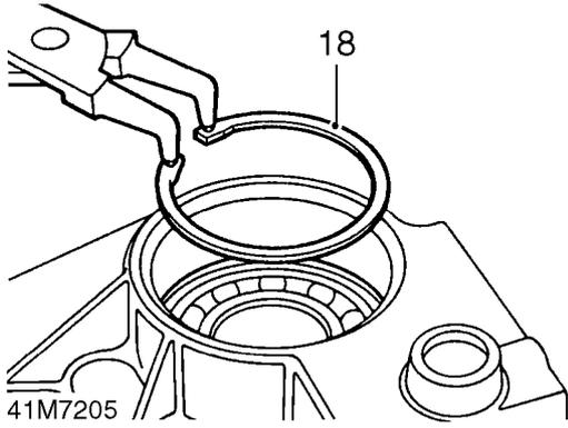
18. Using suitable circlip pliers, remove and discard circlip retaining output shaft bearing.
