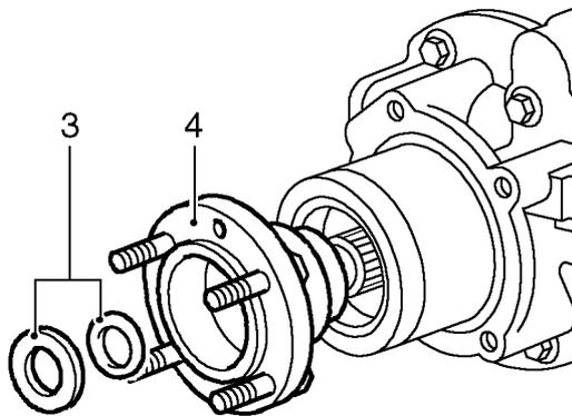
3. Remove steel and felt washers, discard felt washer.
