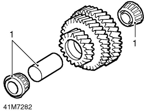
1. Insert a new collapsible spacer into intermediate gears, fit bearings into bearing tracks.
