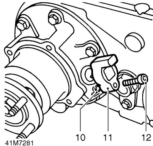
10. Lubricate a new 'O' ring with recommended oil and fit to vehicle speed sensor - if fitted.
