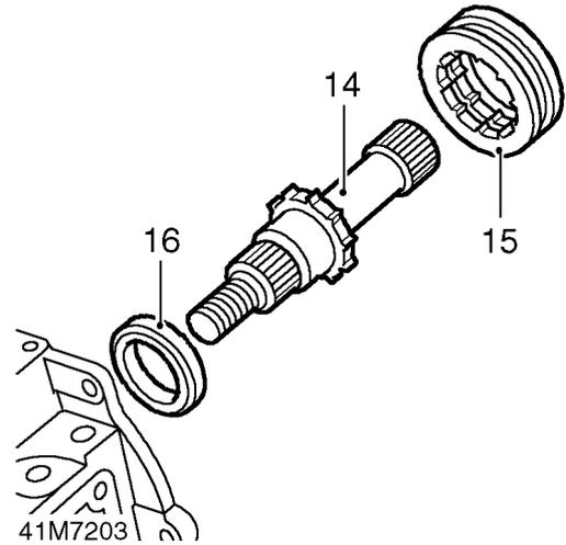
14. Using a mallet, drive output shaft out of front output housing.
