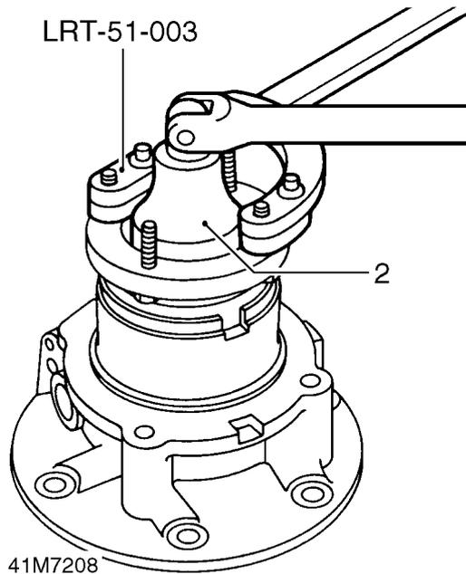
1. Position propeller shaft flange holding tool **LRT-51-003** to output shaft flange.
