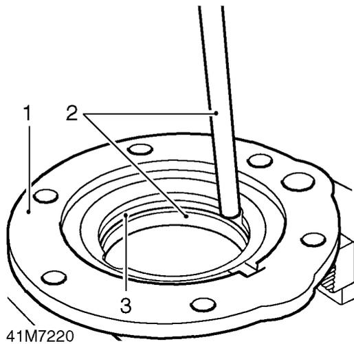
1. Secure mainshaft input gear bearing housing in a soft-jawed vice.
