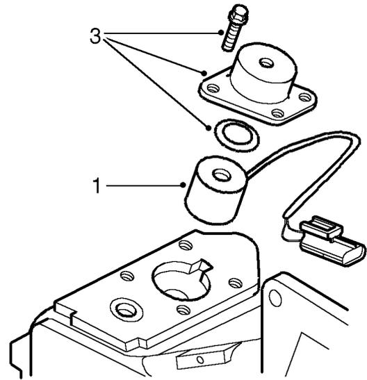
1. Position solenoid in main casing.
