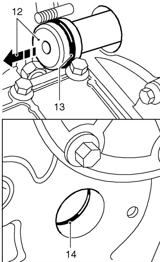
12. Using a soft metal drift on threaded end of intermediate shaft, drive shaft out of main casing.
