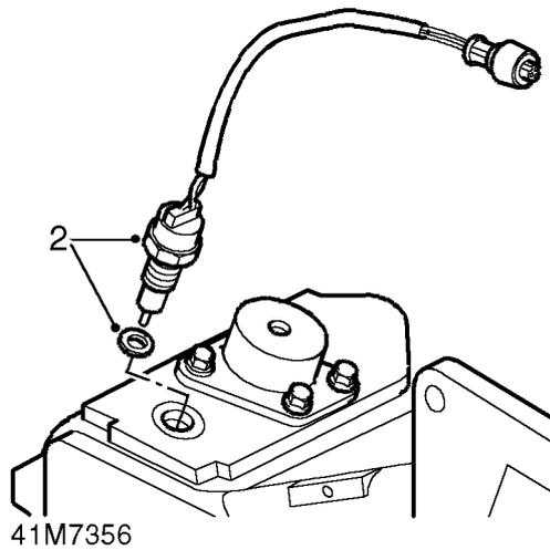
1. Apply Hylosil PL 32 sealant to threads of switch.
