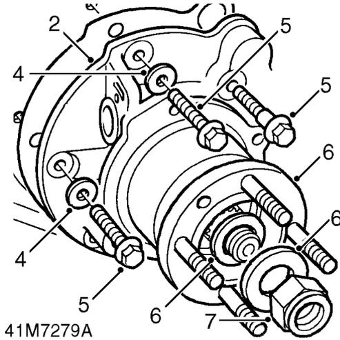
2. Fit rear output housing to main casing.
