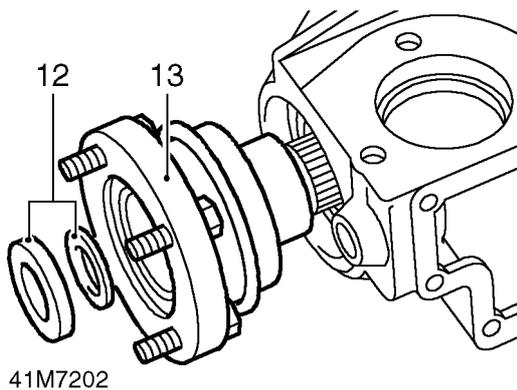
12. Remove steel and felt washers, discard felt washer.
