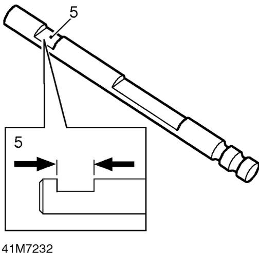
5. Check differential lock selector finger groove width in differential lock selector shaft:
