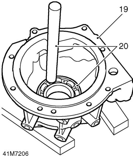
19. Support front output housing on suitable blocks of wood.
