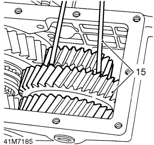
15. Wrap a suitable length of wire around intermediate gears and using assistance, lift gears out of main casing.
