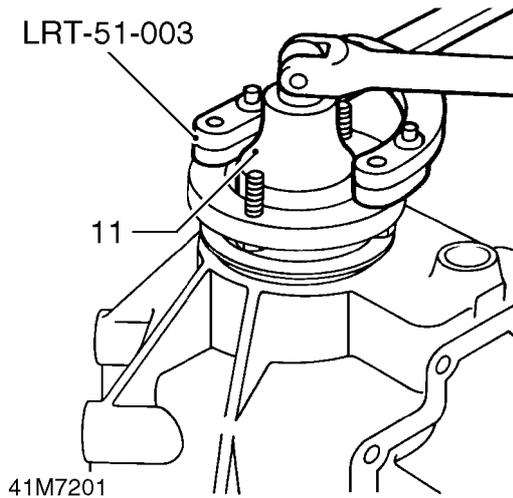
10. Position propeller shaft flange holding tool **LRT-51-003** to output shaft flange.
