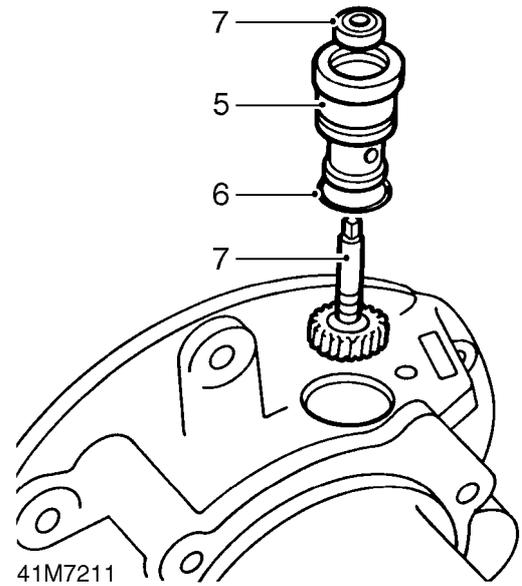
5. Carefully lever speedometer driven gear and housing out of rear output housing.
