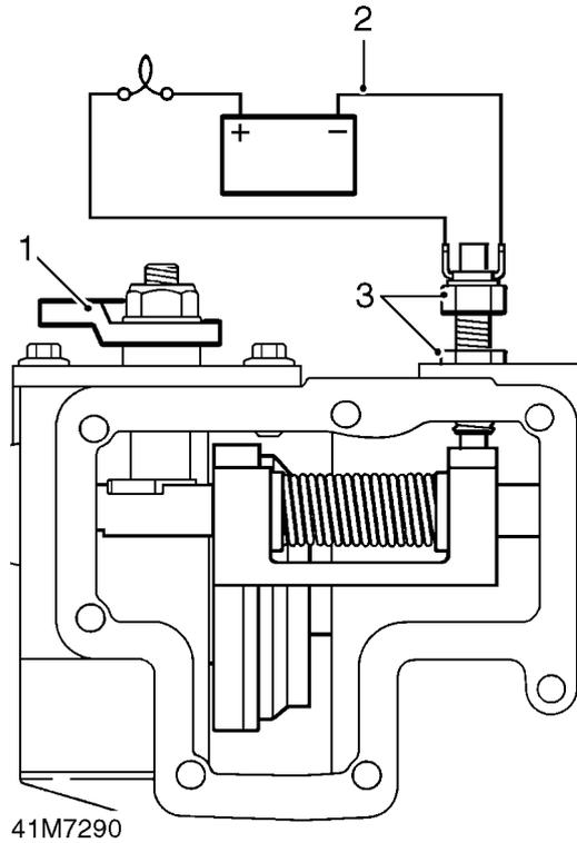
1. Move differential lock selector fork to differential locked position.
