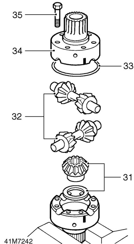
31. Fit a 1.05 mm (0.04 in) thick thrust washer to rear half carrier sun gear, position gear in rear half carrier.
