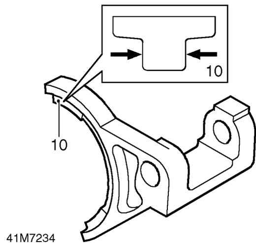
10. Check differential lock selector fork finger width:
