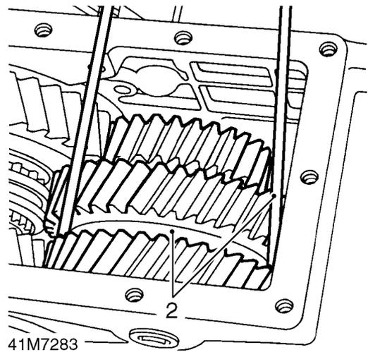
2. Wrap a suitable length of wire around intermediate gears and using assistance, lower gears into main casing ensuring that they are meshing with input and differential gears.
