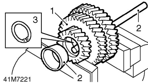
1. Secure intermediate gears in a soft-jawed vice.
