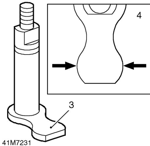
3. Check differential lock selector finger for wear.
