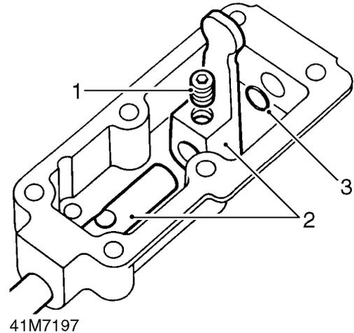
1. Remove setscrew securing high/low selector finger to cross shaft.
