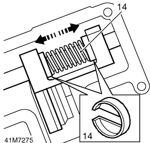
14. Compress selector spring and fit retaining clips at each end of spring.
