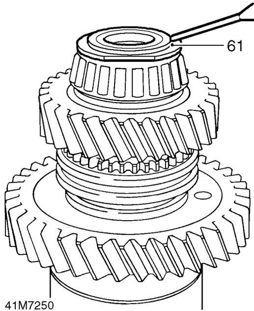
61. Using a round nosed punch, stake collar of nut into recess in differential shaft.
