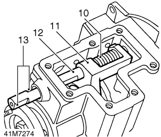
10. Compress differential lock selector spring and fit to selector fork.
