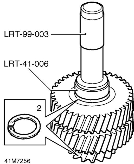
2. Fit new circlips into intermediate gears.
