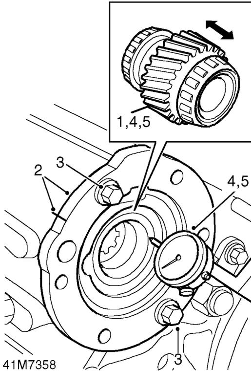
1. Position mainshaft input gear assembly in main casing.
