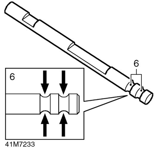
6. Check detent grooves in differential lock selector shaft for wear.
