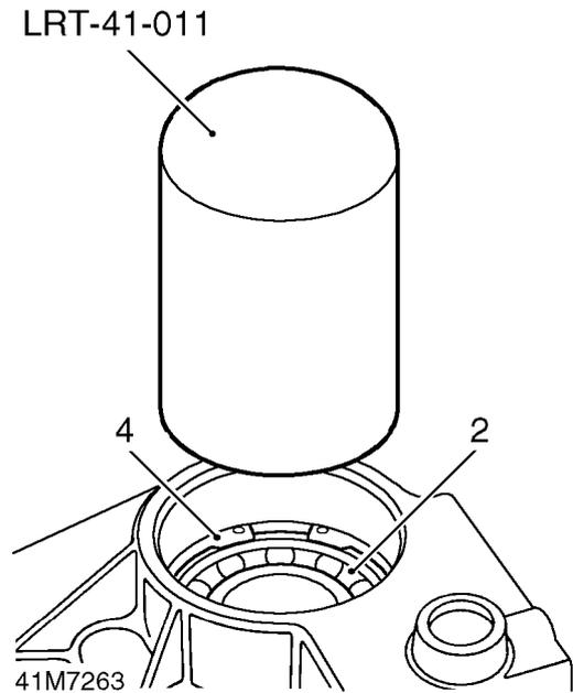
2. Fit new output shaft bearing using tool **LRT-41-011**.
