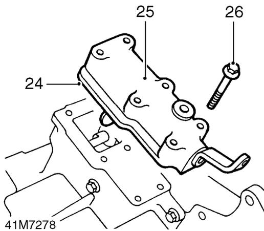
24. Apply Hylosil RTV 102 sealant to mating flange of high/low selector housing.
