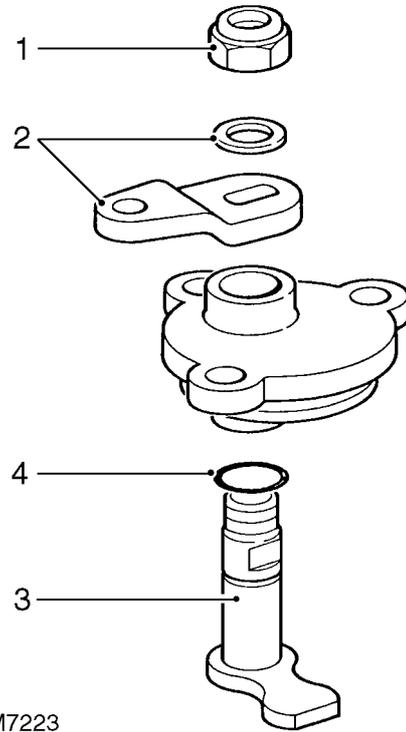
1. Remove and discard self-locking nut retaining selector lever.
