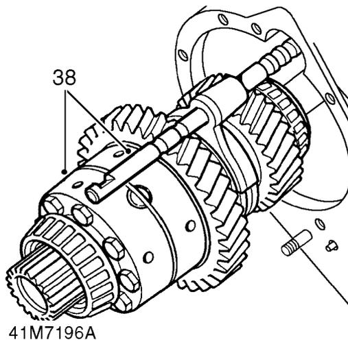
38. Withdraw differential assembly together with high/low selector shaft and fork.
