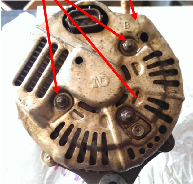
Remove the bolts (screw them back in after removing all parts) to remove the regulator, the brushes, and the rectifier
