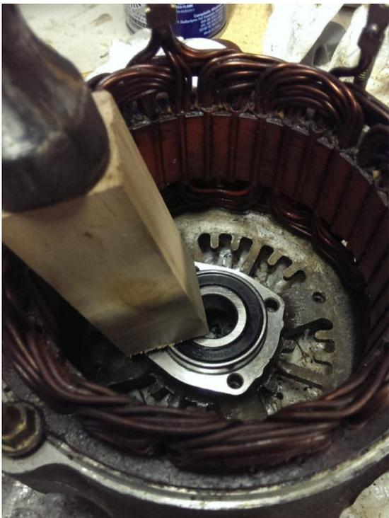
Insert the other bearing in the alternator case. I used a wood stick because it is not possible to reach it with the hammer, and using a wood stick rather than a metal stick will avoid to damage the bearing. Hit the bearing only on the edge.
