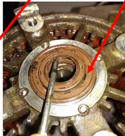
Remove the bearing (OD=40mm, ID=17mm, th=12mm) hitting with a hammer on a 22mm socket seated on the bearing.
