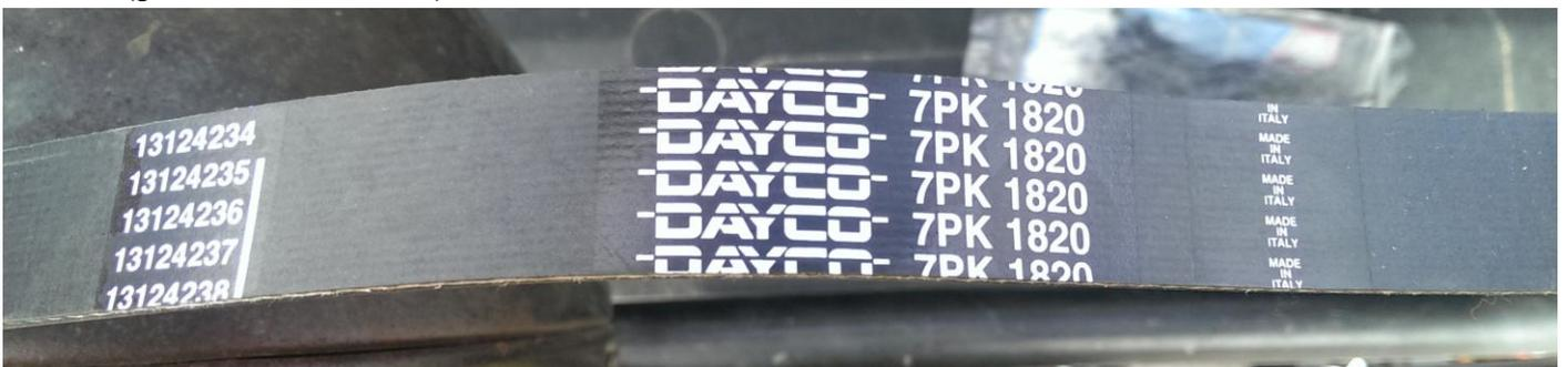
Now you have to remove the drive belt. To do so, use a 15mm spanner to disengage the **drive belt tensioner**, and remove the belt **pulling** from the **bottom**
