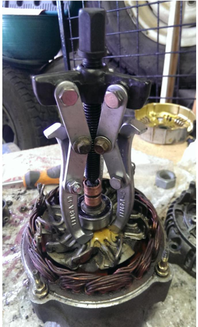
Remove the rotor and clean all the parts with a lubricant.
