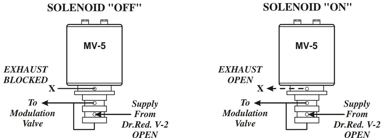
When MV-5 solenoid is "OFF," solenoid reducing pressure, from Dr. Red. V-2, is high to MOD-V valve which creates high line pressure.
