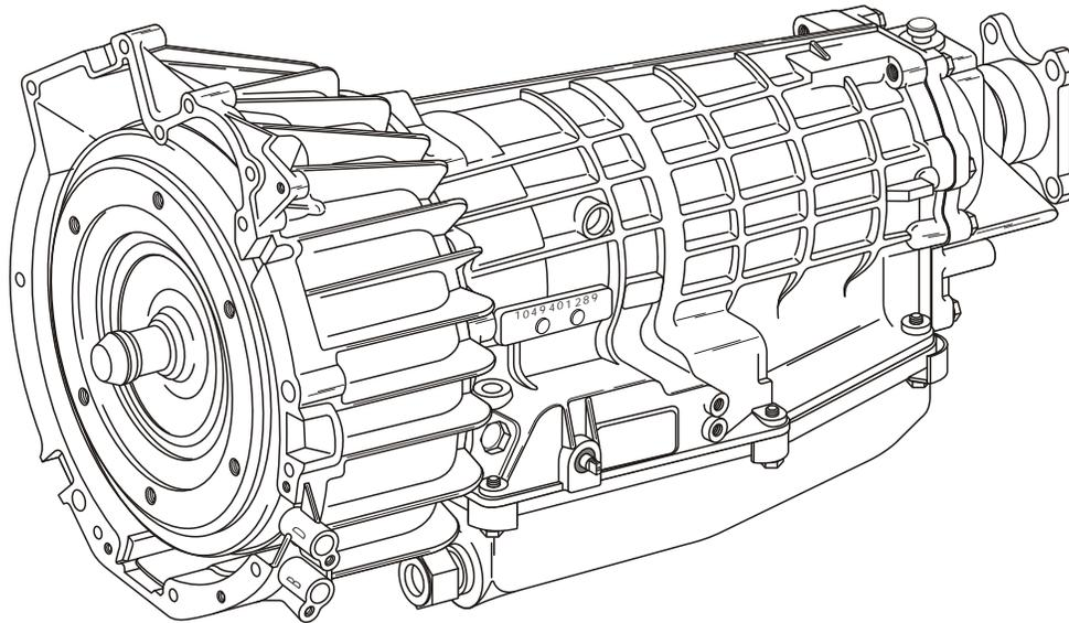
The Electronic Control system was first introduced in 1986 and was incorporated into the totally hydraulic 4HP-22 unit produced by ZF. It combines the hydraulic control of forward and reverse gear engagement, with electronic control for automatic upshifts from 1st thru 4th and automatic downshifts from 4th thru 1st gears. Three different versions of valve bodies have been used on BMW vehicles, with minor differences between them
